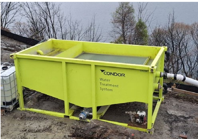
Water treatment system / settlement tank as part of the treatment train
