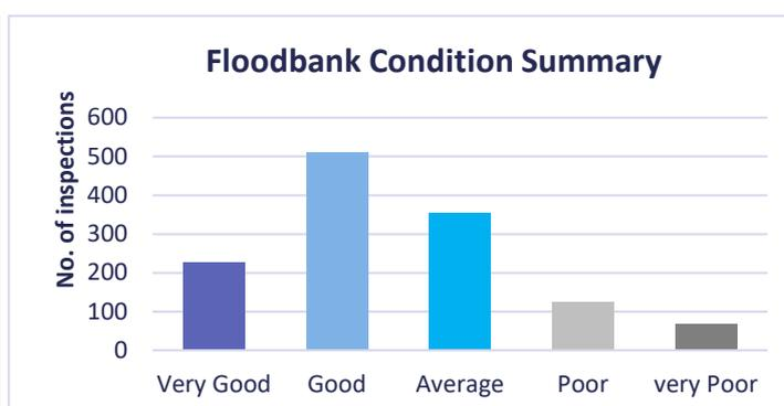
*Figure 10 Summary of floodbank condition by grade. Source T+T, 2018. N.b. Inspection frequency varies, average is one inspection every 170 metres of floodbank.*
