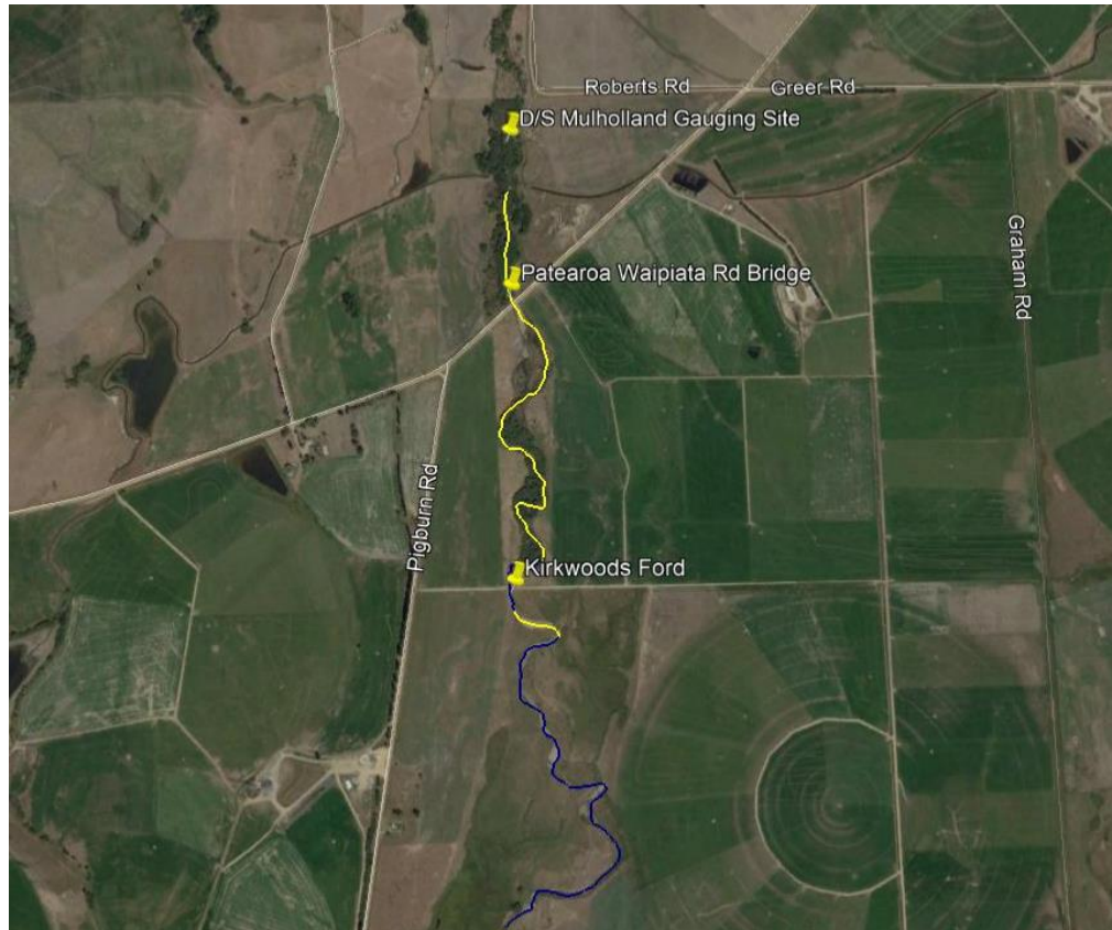
Figure 2. Aerial photograph of the lower losing reach on the 18 th of January 2020, three days prior to the gaugings in Table 4. The flow pattern above matches the gauged flow pattern on the 21 st of January 2020. Dry reaches are in yellow and wetted reaches are shown in blue.
