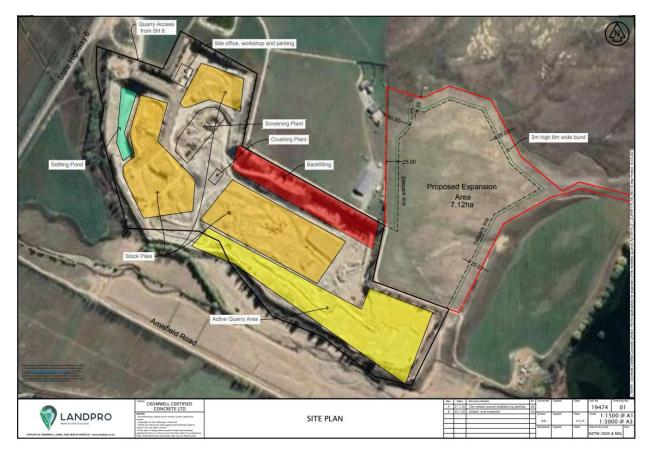
Figure 2-1: Amisfield quarry proposed site plan (Source: Beca, 2020).
