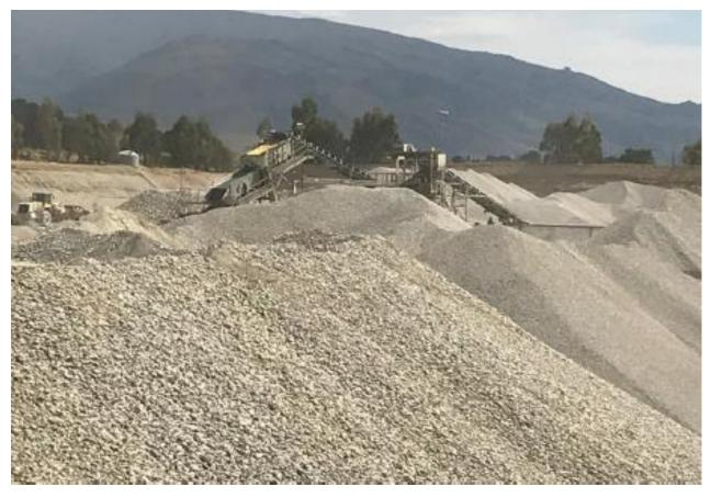
Figure 3-3: Photograph of screening and washing plant with washed aggregate in the foreground (Source: Beca, 2020).
