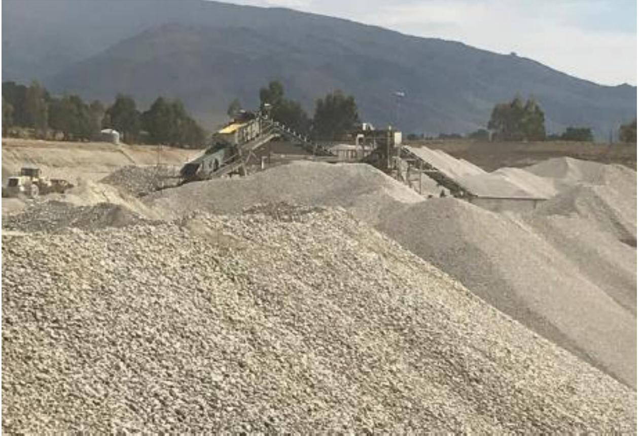
**Figure 3-3: Photograph of screening and washing plant with washed aggregate in the foreground (Source: Beca, 2020).**
