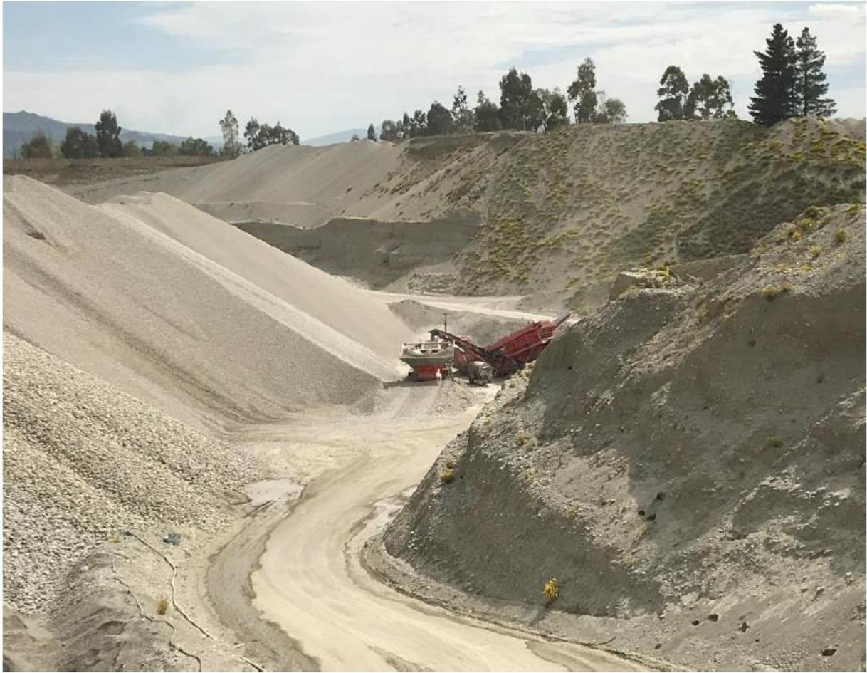
**Figure 3-2 Photograph of mobile crushing plant operating on the quarry floor (Source: Beca, 2020).**
