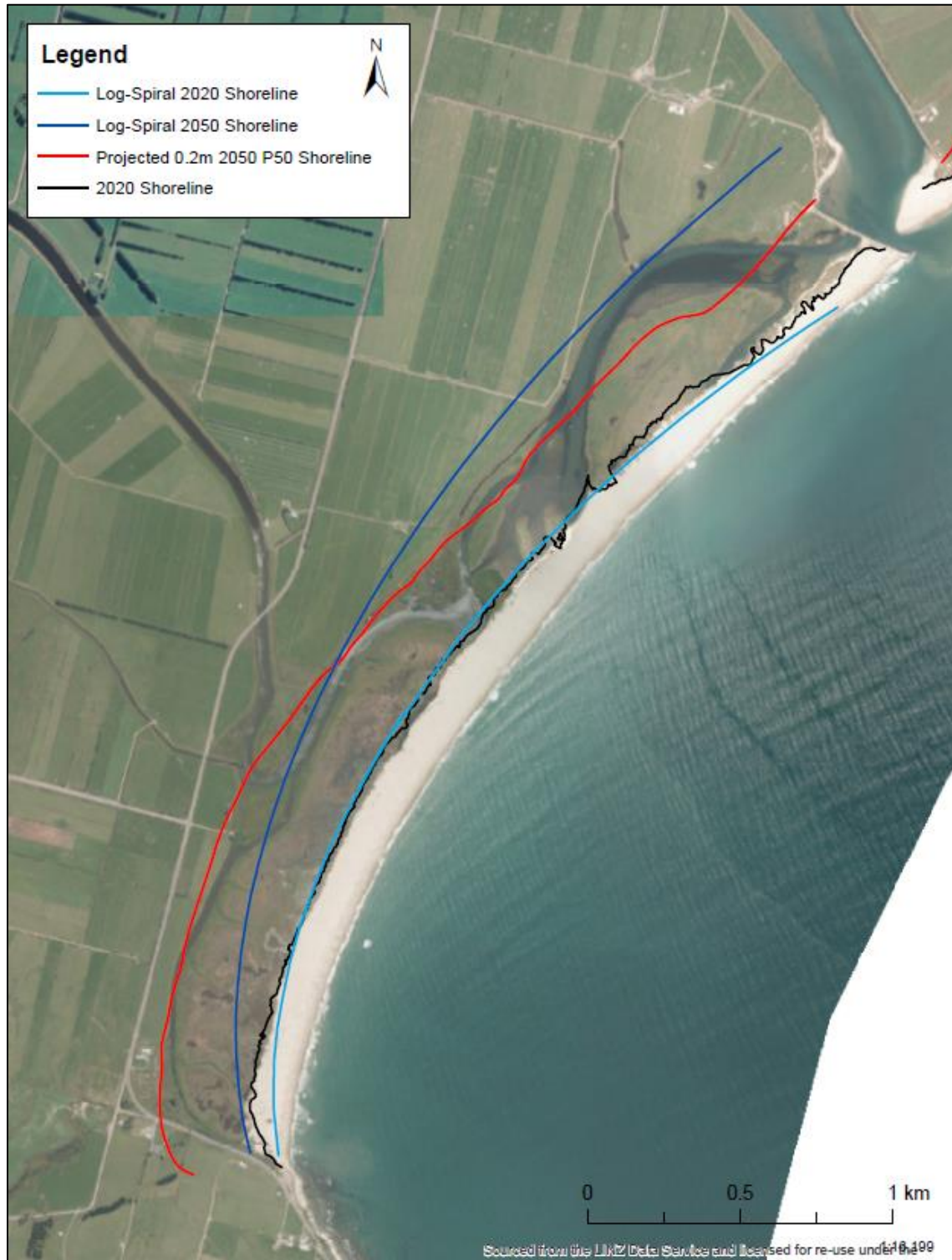
Figure 4.7: Theoretical log-spiral plan shape fitting for southern Molyneux Bay compared to calculated PFSP over a 30-year period to 2050.
