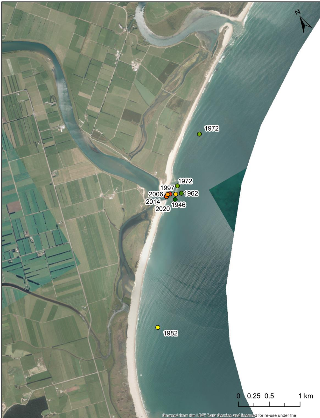
Figure 4.3: Koau River Mouth longshore positions from aerial photographs 1946-2020. Note the 1972 image shows two river mouth openings to the ocean.
