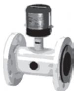
Electromagnetic flow meters provide high-accuracy readings, especially at lower flow rates. These are also available in a clamp-on option, but long-term installations tend to be built-in. Pricing is often slightly higher than clamp-on meters, as the electrodes are mounted in a heavy duty flange which must be fitted into the pipeline. Power is required, but can be sourced from battery or mains. A datalogger can be attached with telemetry if desired.
