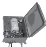
This system relies on measuring the force required to move an air bubble out of the end of a pipe submerged in the channel to find the depth of water in that channel. This system can be accurate, but requires a specialist to set up and cannot be mechanically dampened. Because all electronics can be installed a reasonable distance from the water, this system can be ideal for sites where equipment could get washed out.
