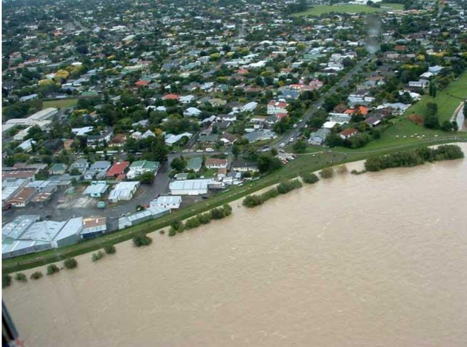
Figure 4.1: Stopbanks protected Palmerston North from inundation during the 2004 Manawatu River flood event. Source: [teara.govt.nz](http://teara.govt.nz)
