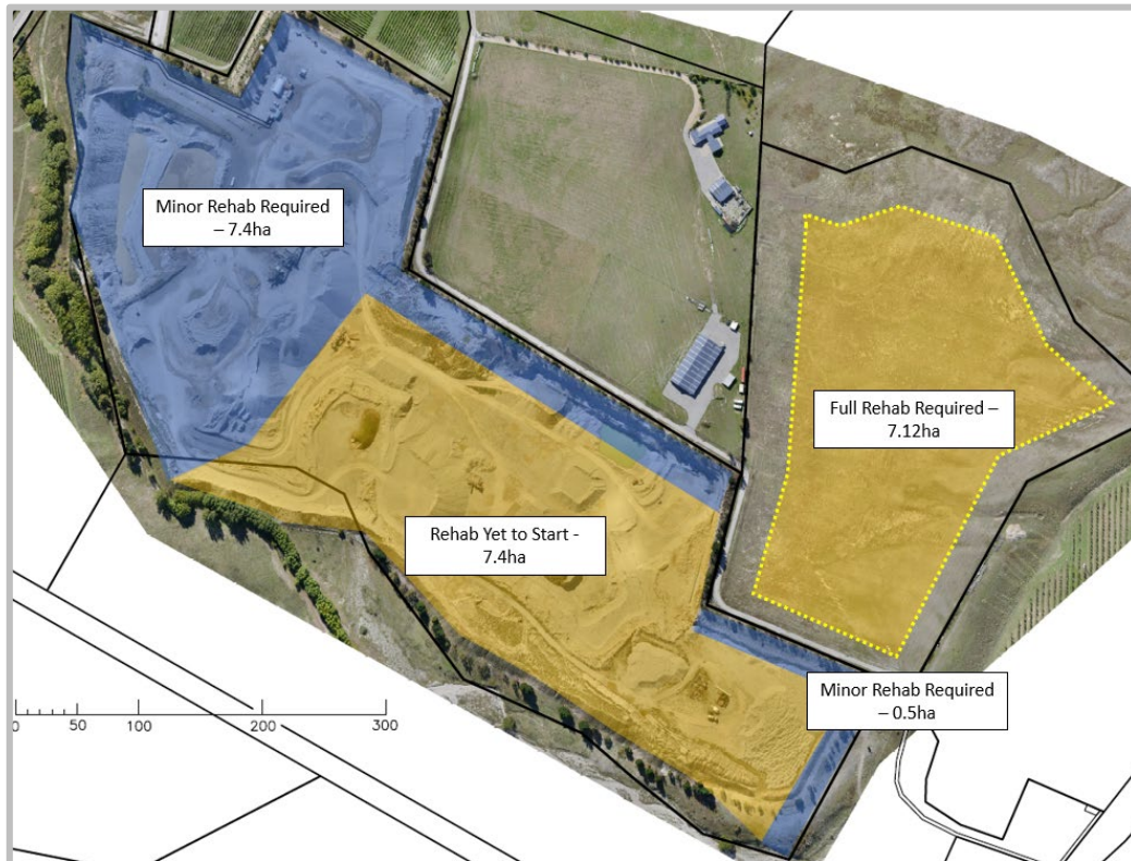
Fig. 2: Areas to be Rehabilitated
