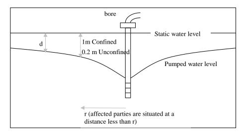
The radius will be determined using a significant interference of  $d \ge 1$  m for confined aquifers or  $d \ge 0.2$  m for unconfined aquifers, and the 'Theis' equation:
