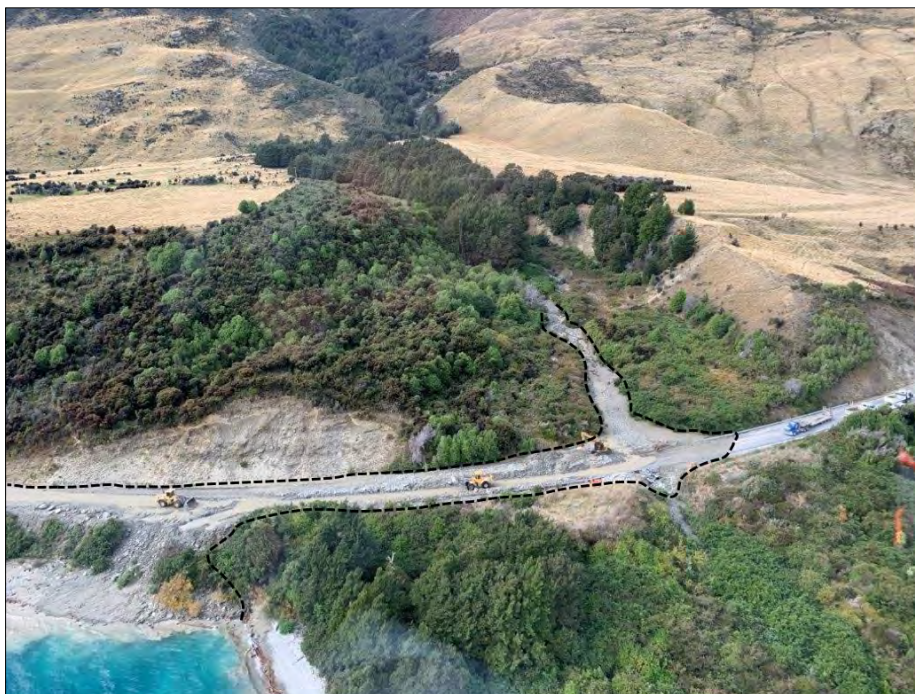
Figure 20: Aerial view of debris flow impacts at the Queenstown-Glenorchy road, annotated to show the approximate extent of debris deposition (photo provided by Maddi Phillips, WSP Ltd).
