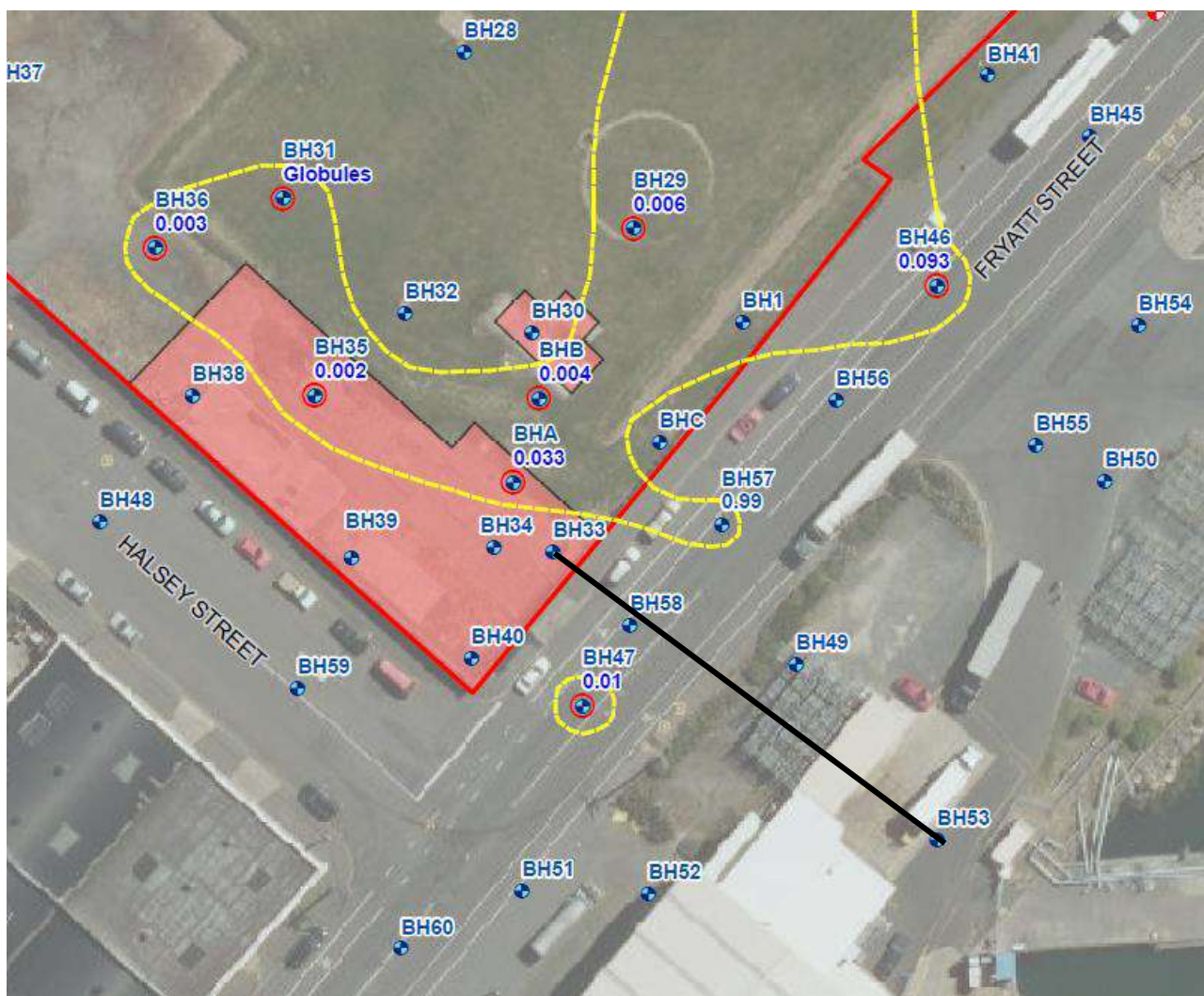
Figure 25: Transect location and monitoring wells used for natural attenuation rate assessment. Transect defined by black line. Inferred extent of LNAPL in April 2017 defined by yellow line.
