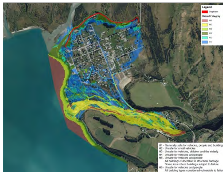
Figure 4: Flood hazard categorisation for a Buckler Burn flooding scenario with a 300 cumec peak flow (<1% AEP) and 3 metres channel aggradation on the mid-upper reaches of the alluvial fan. Colouring shows hazard categorisation according to the included legends.
