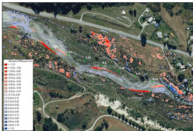
Figure 7-2 – GCD analysis between the 2022 and 2019 LiDAR. The dark red areas along the edges of the active braid plain indicate erosion and widening, whilst the dark blue between 0.25 and 0.30m likely indicates vegetation growth.
