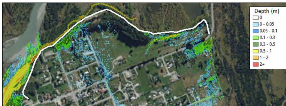
Figure 6-3 – Floodwaters from the Buckler Burn pooling behind the Glenorchy stopbank and eastern end of Mull St in the 250m 3 /s design (2019) run.
