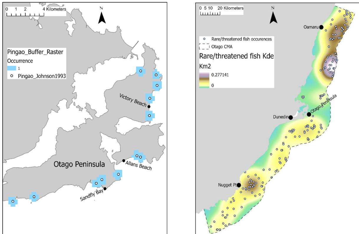
**Figure 2-3: Formatting point data.** Examples of formatting point data as raster datasets using two methods. Converting buffered areas around points to occurrence (left), and using Kde to construct a density surface (right).
