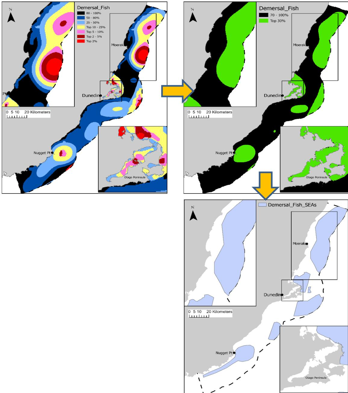
**Figure 2-4: Zonation SEA delineation.** Example of SEA delineation using Zonation where the output of a spatial prioritisation (top left) is converted to represent the top 30% priority areas (top right), with the final SEA boundaries being constructed as polygons (bottom). Note in this example using the demersal fish class, commercially sensitive data on catch distribution is masked out.
