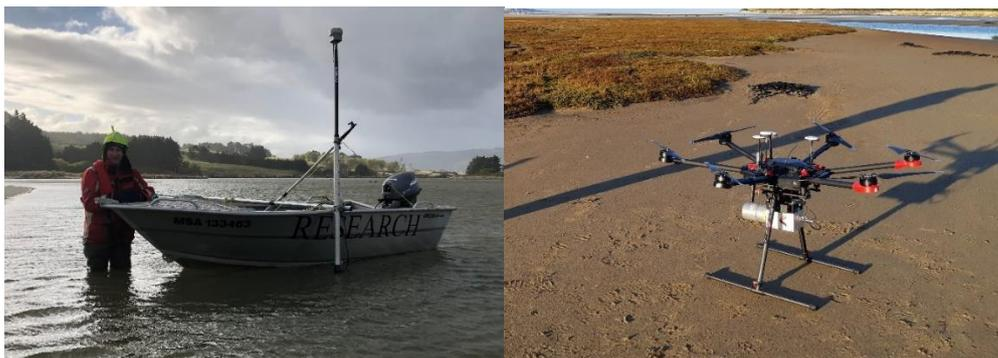
**Figure 3-1: Bathymetric surveying.** Bathymetry of submerged areas were mapped using a boat-mounted Sonarmite echosounder, with positions recorded with RTK-GPS. Intertidal areas were mapped with a drone-mounted LiDAR USA laser scanner.
