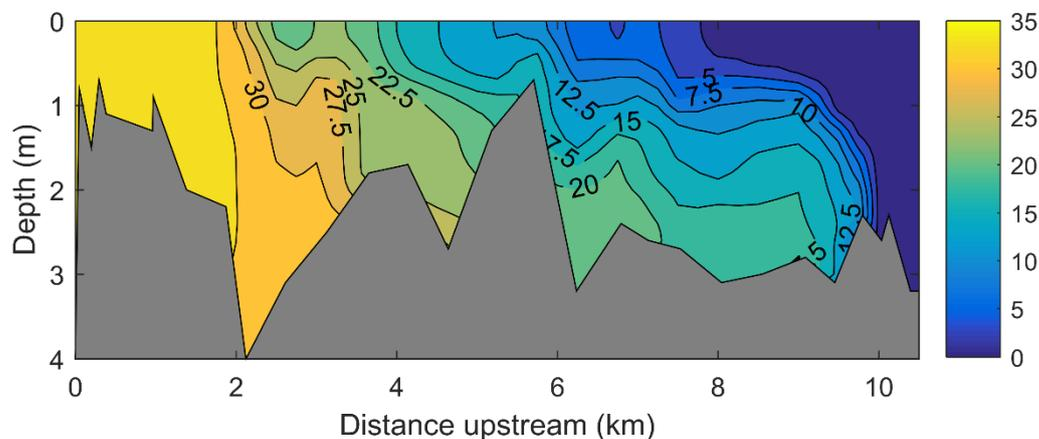
**Figure 3-3: Profiles of salinity recorded along the length of the Tokomairiro Estuary on 2 May 2019.** The presence of saline water was detected up to 9.8 km upstream of the estuary mouth.
