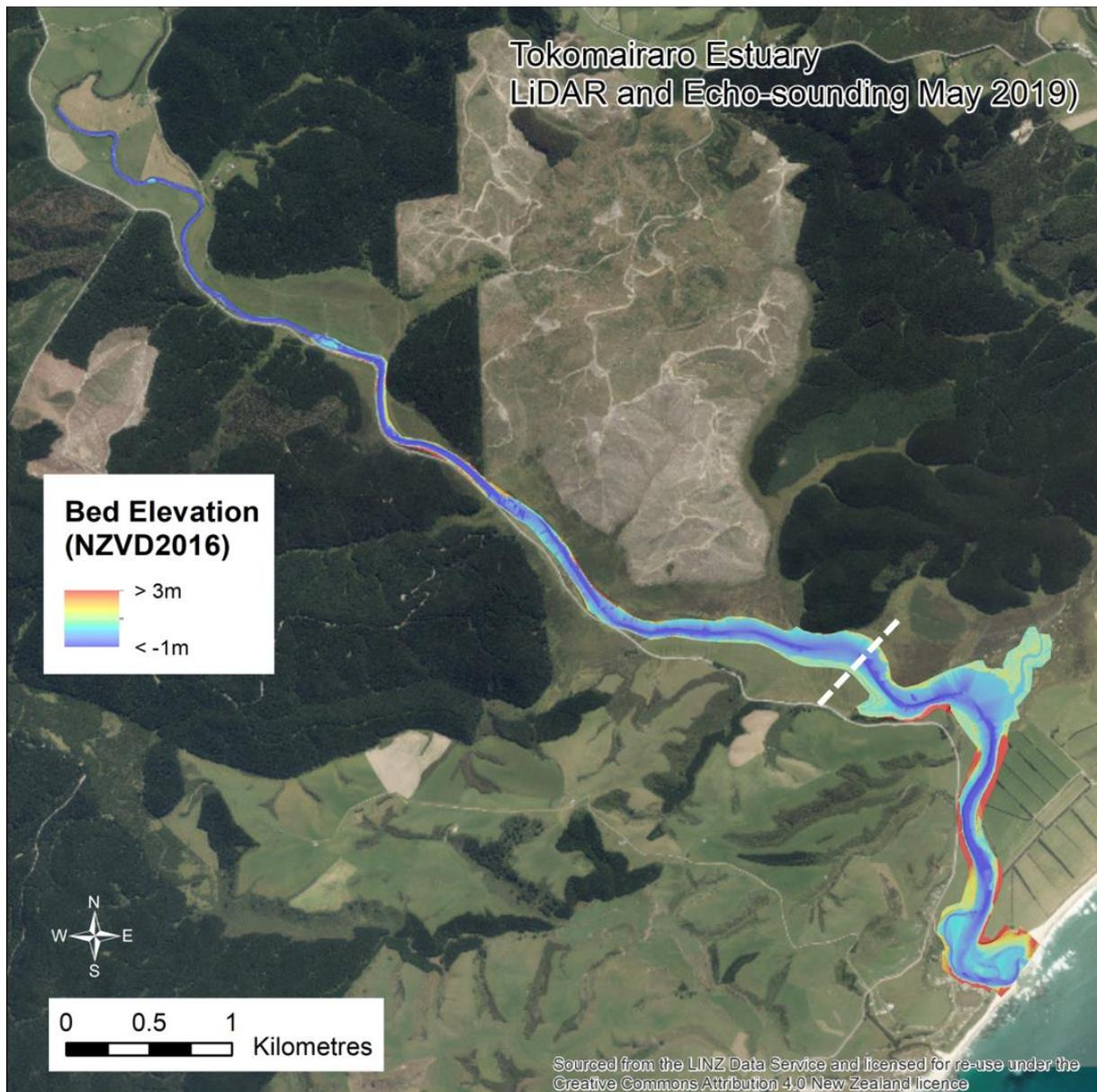
**Figure 3-2: Surveyed bathymetry of the Tokomairiro Estuary.** Bathymetry data compiled from echosounder and drone-based laser scan surveys conducted 30 April – 2 May 2019. Elevations are relative to NZVD 2016. The white dashed line shows where we have separated the upper and lower estuary when using the two-compartment dilution model in our analysis.
