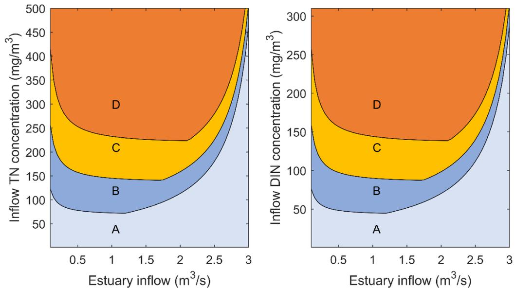
**Figure 8-1: ETI phytoplankton susceptibility bands in the upper Tokomairiro Estuary as a function of flow and inflow nutrient concentrations.** A ratio of DIN:TN = 0.62:1 is assumed, and the nitrogen to phosphorus ratio in the inflow is assumed to remain constant.
