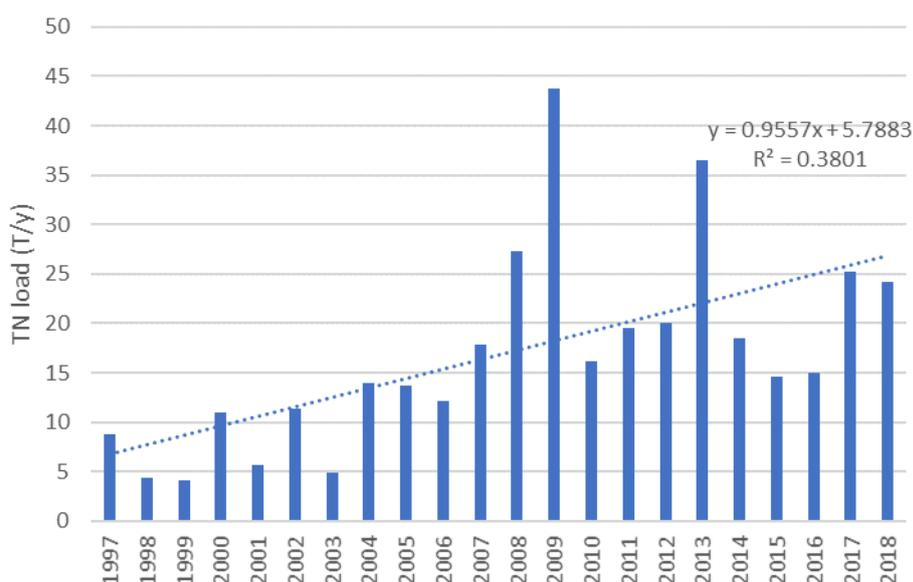
**Figure 2-1: Annual mean total nitrogen loads in the Tokomairiro River at West Branch Bridge.** Annual loads calculated from daily mean flows @ West Branch Bridge and TN concentrations interpolated from nutrient samples @ West Branch Bridge.
