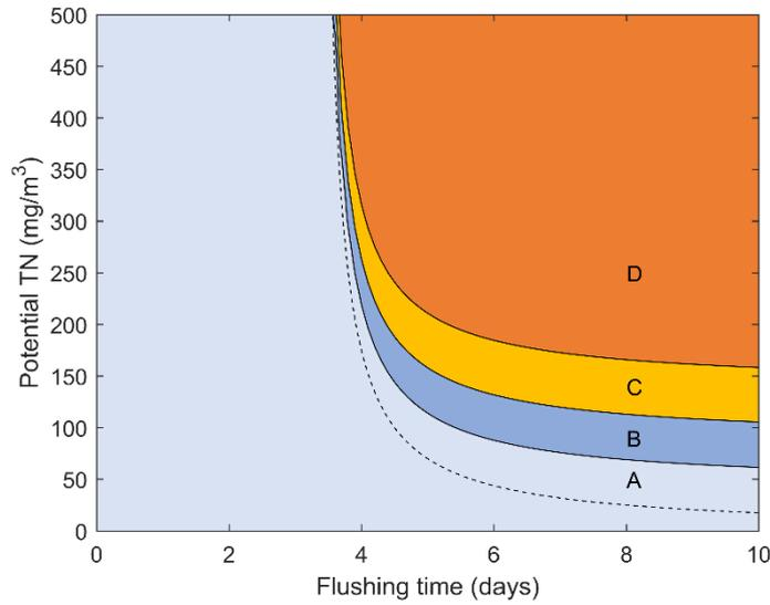
**Figure 6-1: ETI susceptibility bandings for phytoplankton based on flushing time and potential total nitrogen concentrations.** This graph shows model output based on an assumed half saturation coefficient of 35 mg/m<sup>3</sup> TN and a net specific growth rate of 0.3 day<sup>-1</sup>. The solid curves indicate thresholds between ETI bandings, and below the dashed line phytoplankton are flushed from the estuary faster than they grow.
