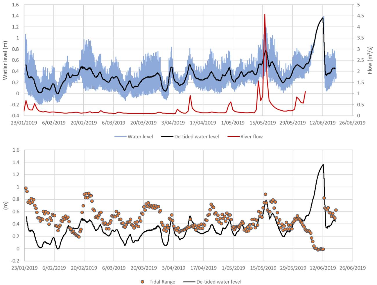
**Figure 3-4: (Upper plot) observed water levels, de-tided water levels in the Tokomairiro Estuary and flows in the Tokomairiro River at West Branch Bridge. (Lower plot) tidal range and de-tided water level in the Tokomairiro Estuary.**
