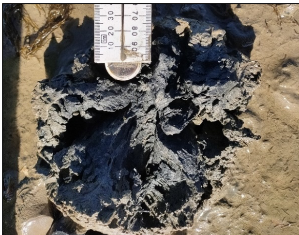
Example of distinct colour change with depth, brown oxygenated sediments are on the surface down to ~10mm
