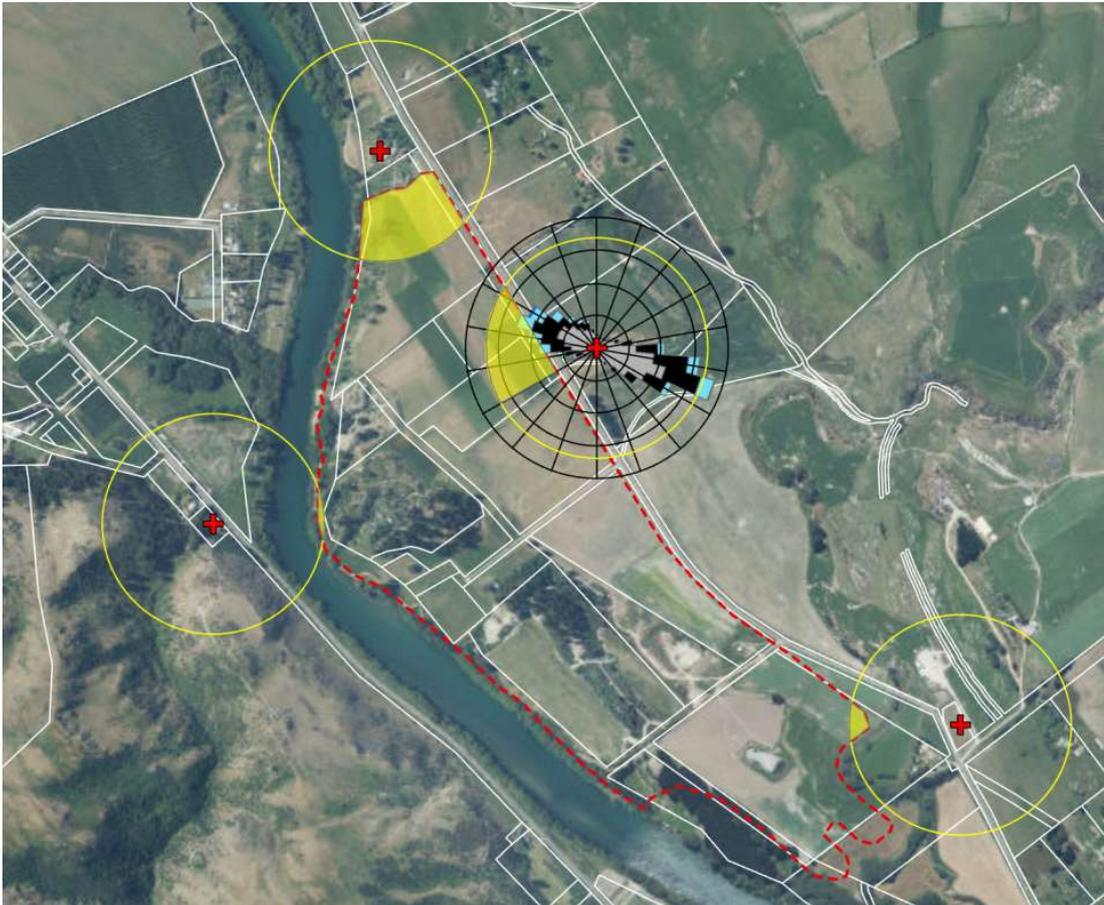
**Figure 5** Sensitive Receptor Management Zone, based on houses within 250m of the work area and within the prevailing wind direction. Wind rose imposed over 1403 Teviot Road, Millers Flat, to demonstrate how prevailing wind direction impacts on the extent of the Sensitive Receptor Management Zone.
