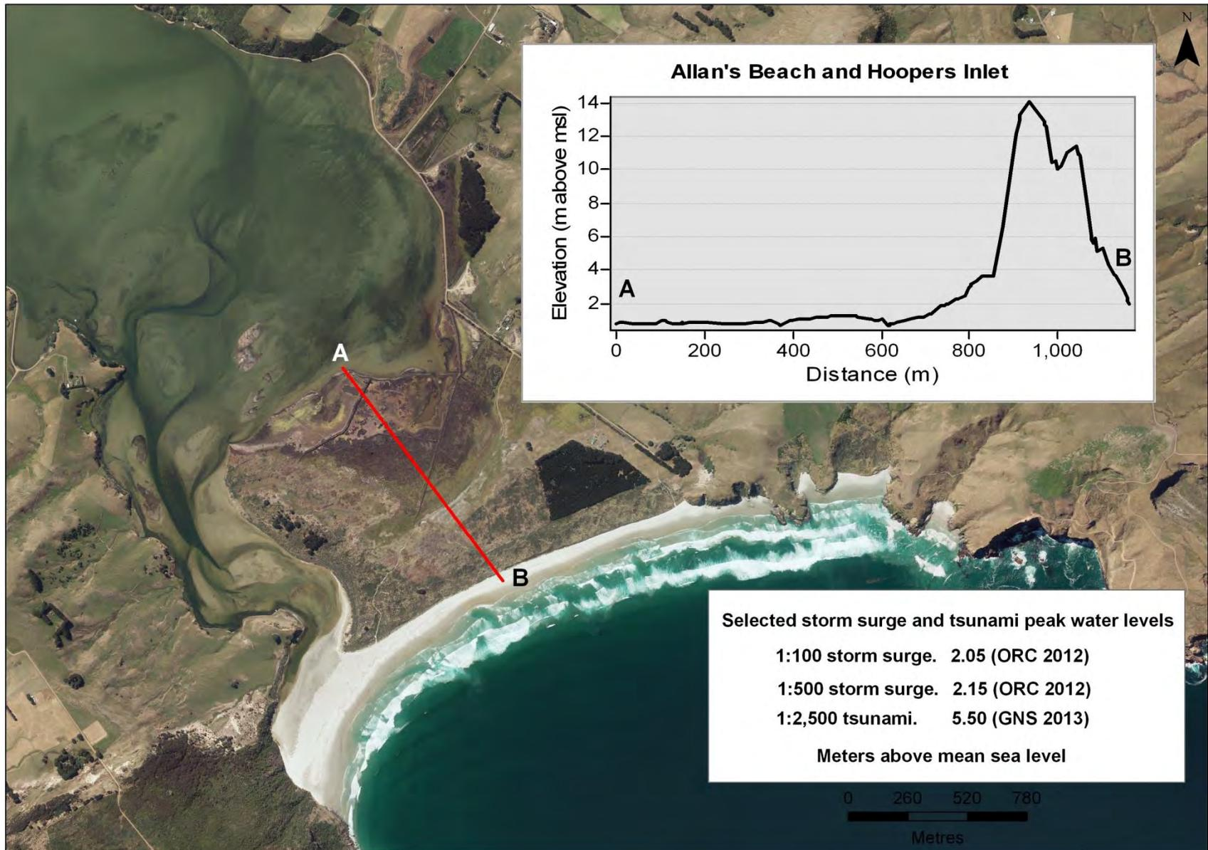
Figure 36. Cross section A-B through Allan's beach and Hoopers Inlet, and peak water levels associated with selected high magnitude storm surge and tsunami events
