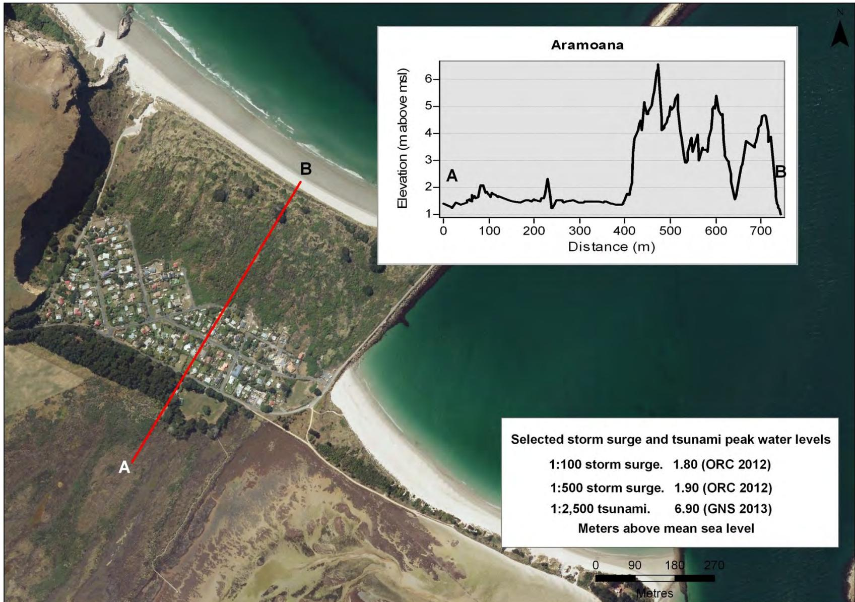
Figure 40. Cross section A-B through Aramoana, and peak water levels associated with selected high magnitude storm surge and tsunami events
