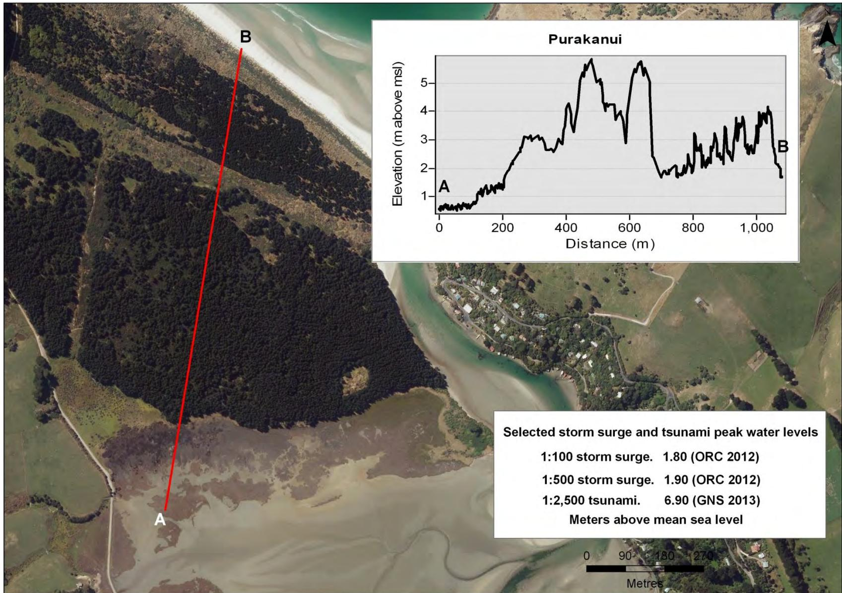
Figure 43. Cross section A-B through Purakanui, and peak water levels associated with selected high magnitude storm surge and tsunami events
