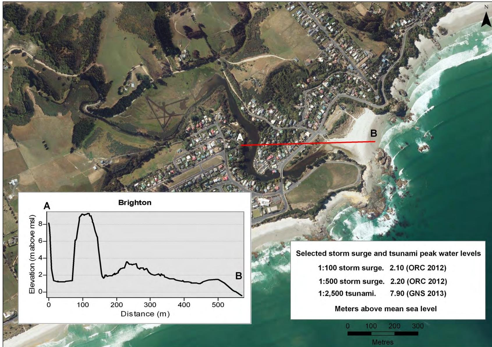
Figure 32. Cross section A-B through Brighton, and peak water levels associated with selected high magnitude storm surge and tsunami events
