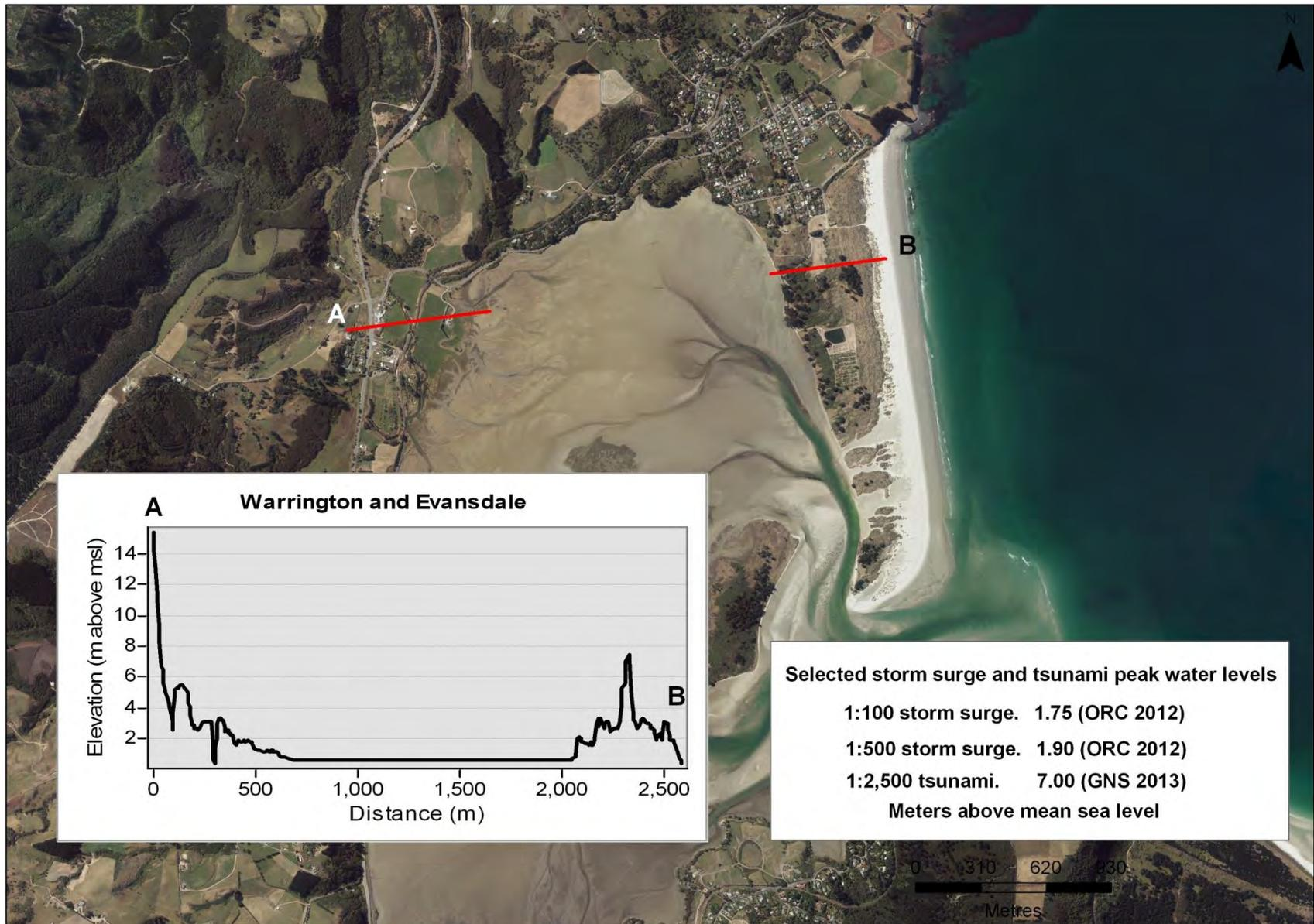
Figure 45. Cross section A-B through Warrington and Evansdale, and peak water levels associated with selected high magnitude storm surge and tsunami events
