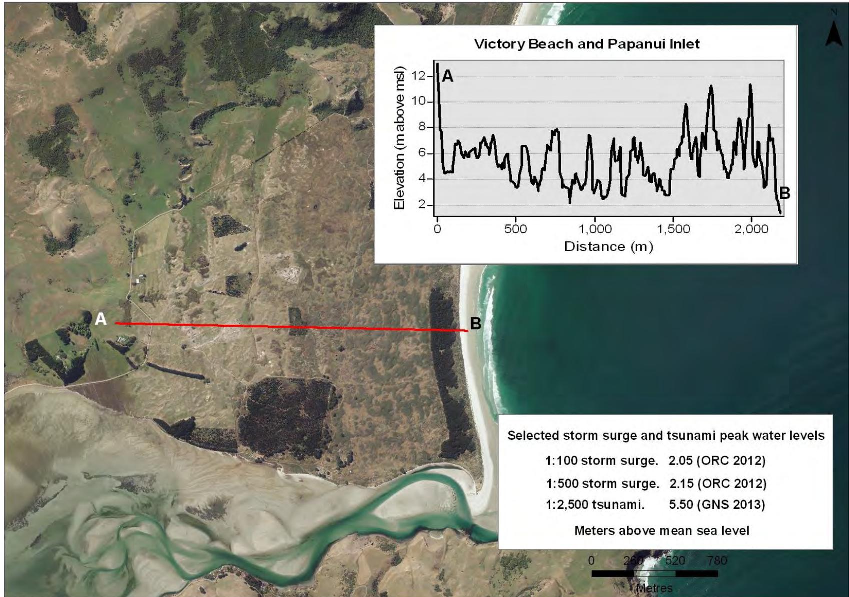
Figure 37. Cross section A-B through Victory Beach and Papanui Inlet, and peak water levels associated with selected high magnitude storm surge and tsunami events
