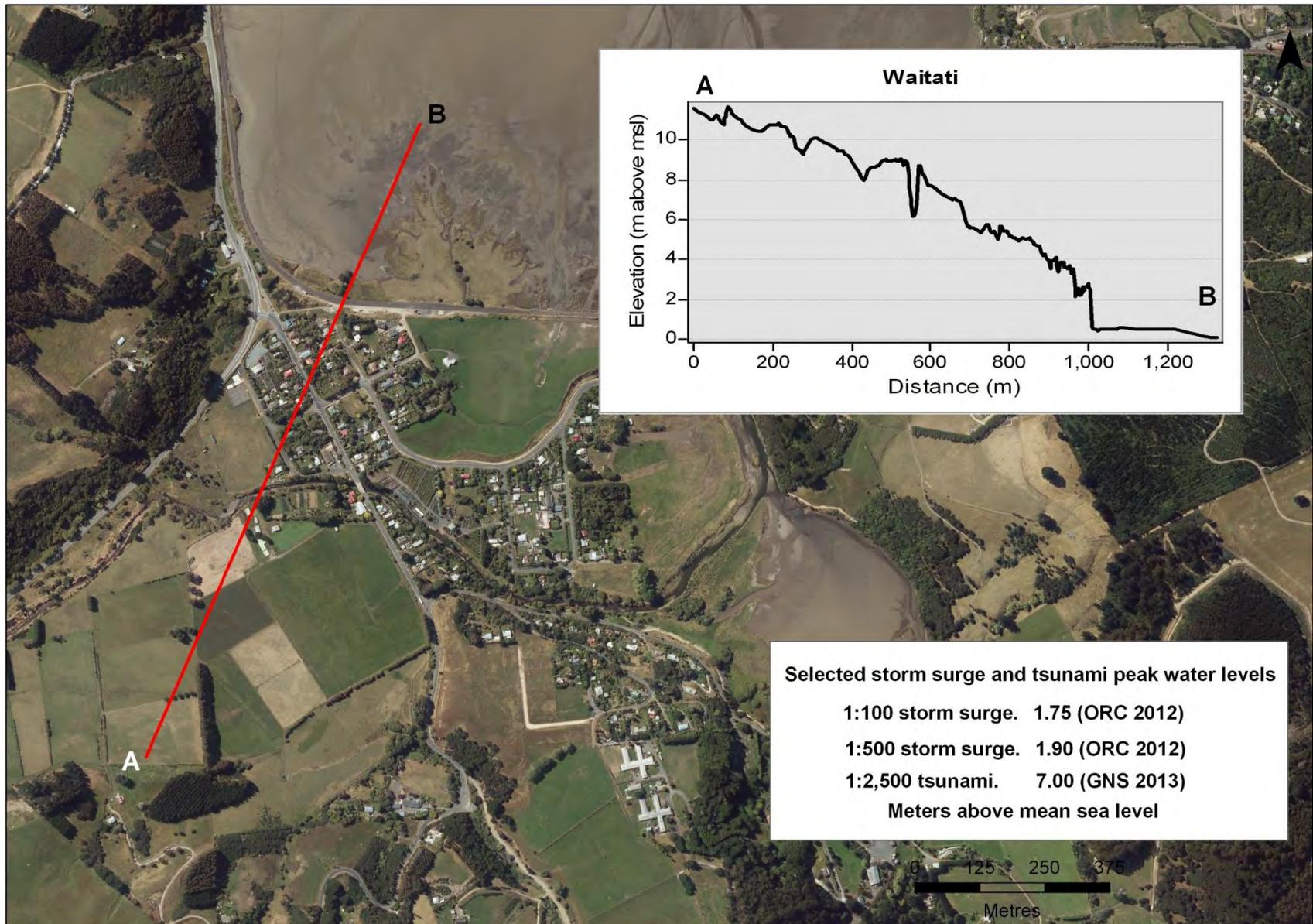
Figure 44. Cross section A-B through Waitati, and peak water levels associated with selected high magnitude storm surge and tsunami events
