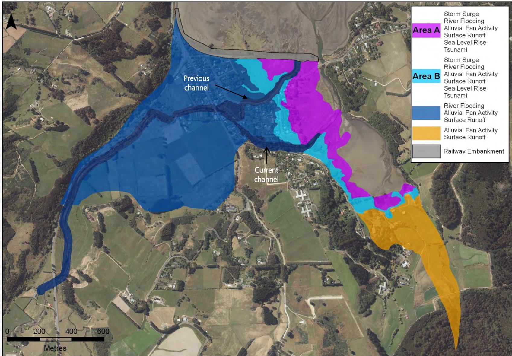
Figure 12: Mapped natural hazard areas in Waitati. The current channel of the Waitati River and the channel that existed prior to a flood event in the 1880's are shown as a darker blue.
