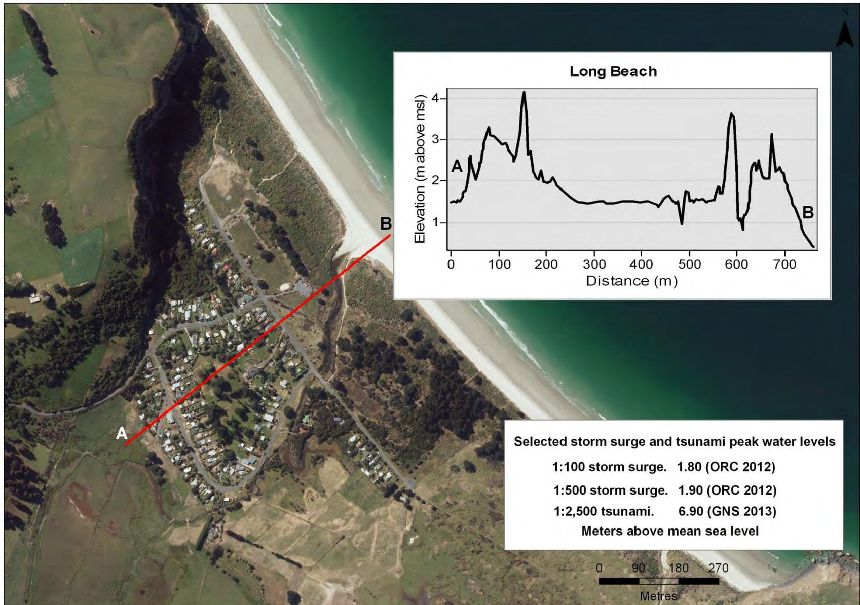
Figure 42. Cross section A-B through Long Beach, and peak water levels associated with selected high magnitude storm surge and tsunami events
