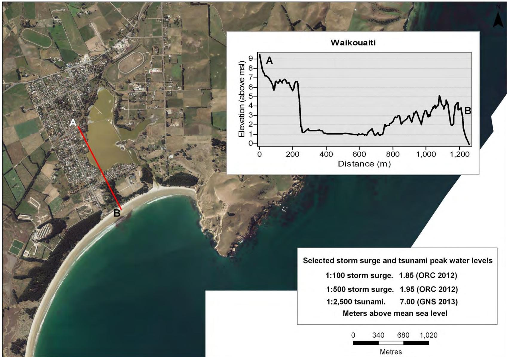
Figure 47. Cross section A-B through Waikouaiti, and peak water levels associated with selected high magnitude storm surge and tsunami events
