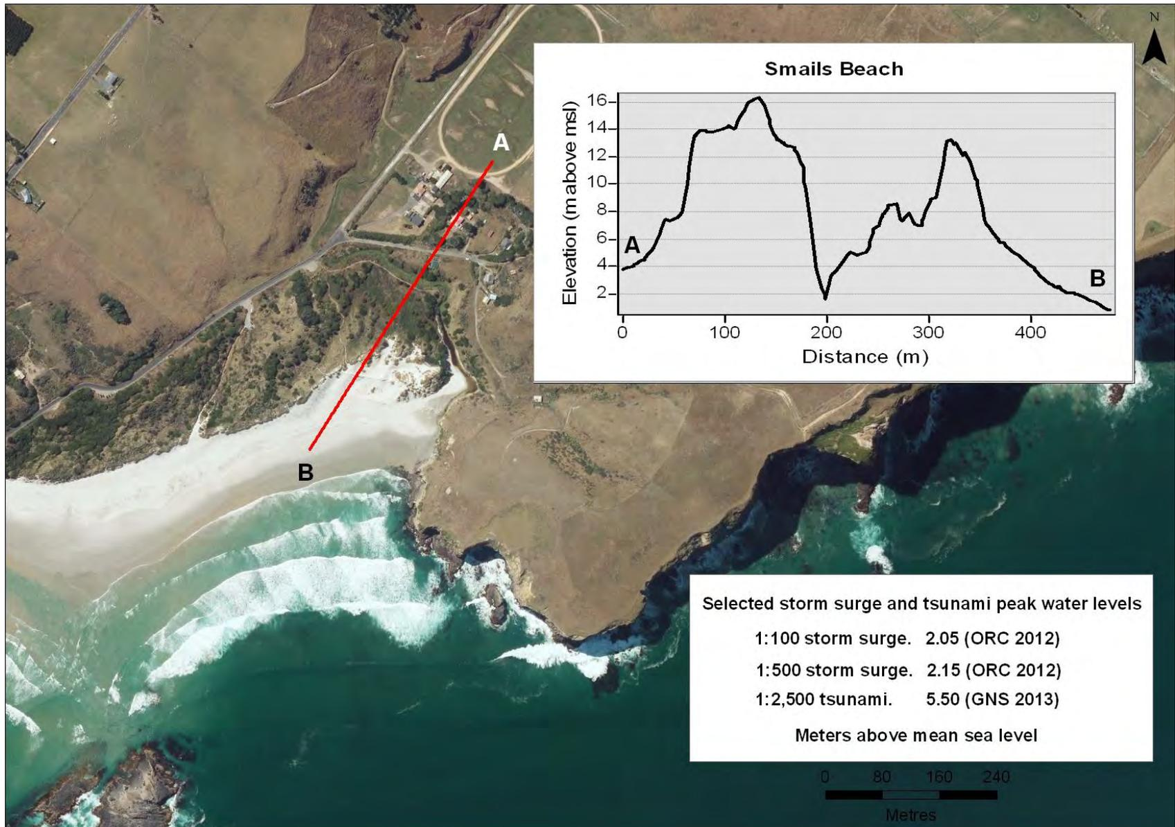
Figure 35. Cross section A-B through Smails Beach, and peak water levels associated with selected high magnitude storm surge and tsunami events
