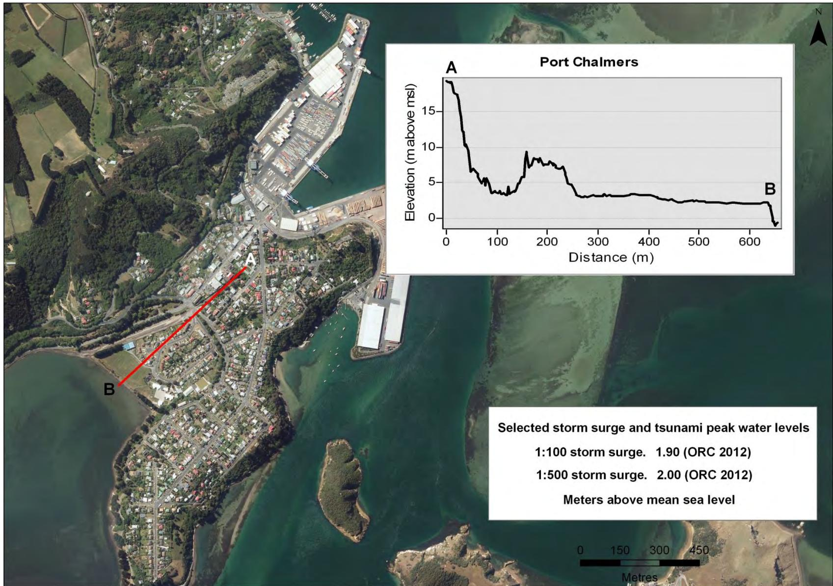
Figure 38. Cross section A-B through Port Chalmers, and peak water levels associated with selected high magnitude storm surge and tsunami events
