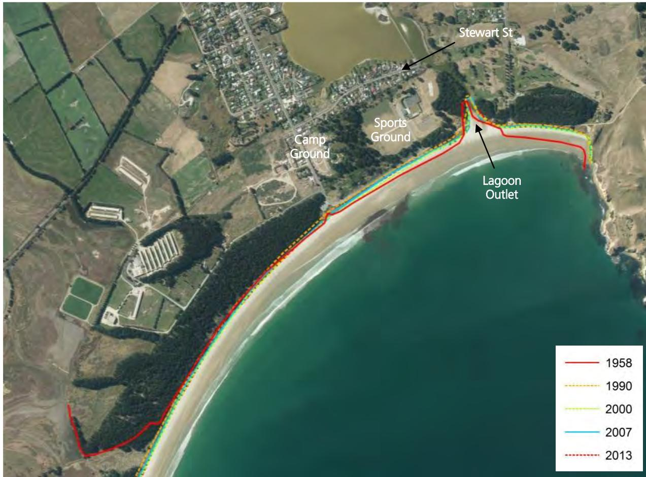
Figure 28. Changes in the Waikouaiti coastline between 1958 and 2013, overlaid on an aerial photograph collected in 2013 (Source: DCC)
