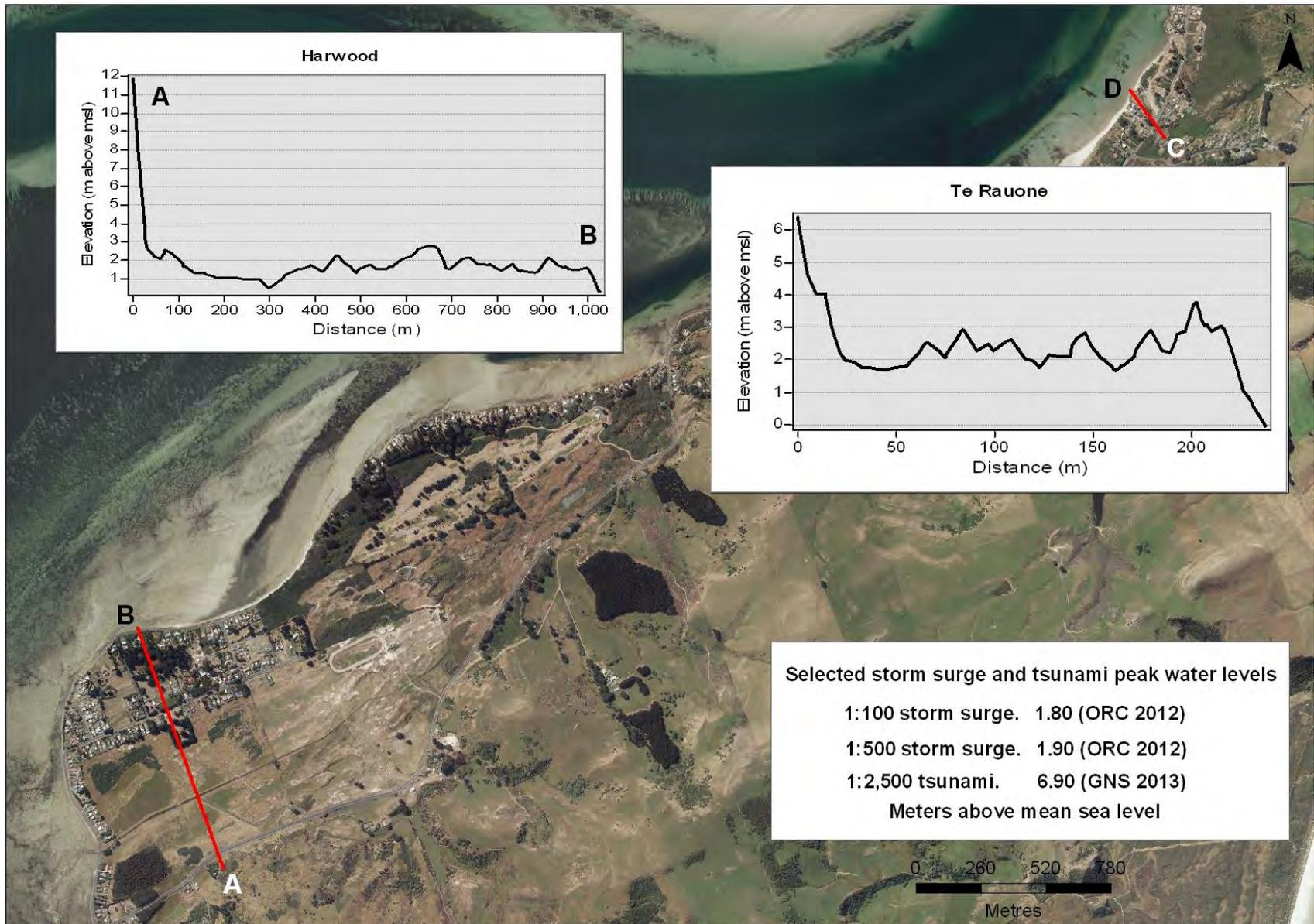
Figure 39. Cross section A-B through Harwood and C-D through Te Rauone, and peak water levels associated with selected high magnitude storm surge and tsunami events
