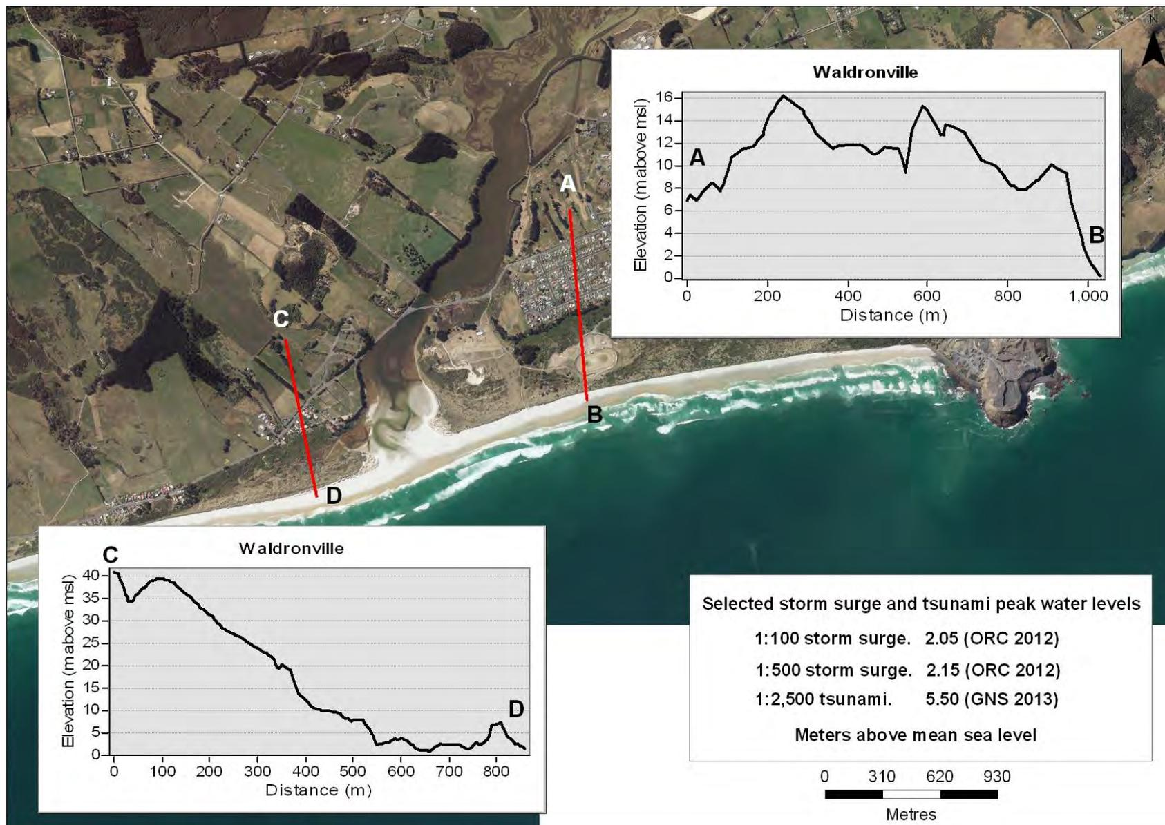
Figure 33. Cross section A-B and C-D through Waldronville, and peak water levels associated with selected high magnitude storm surge and tsunami events
