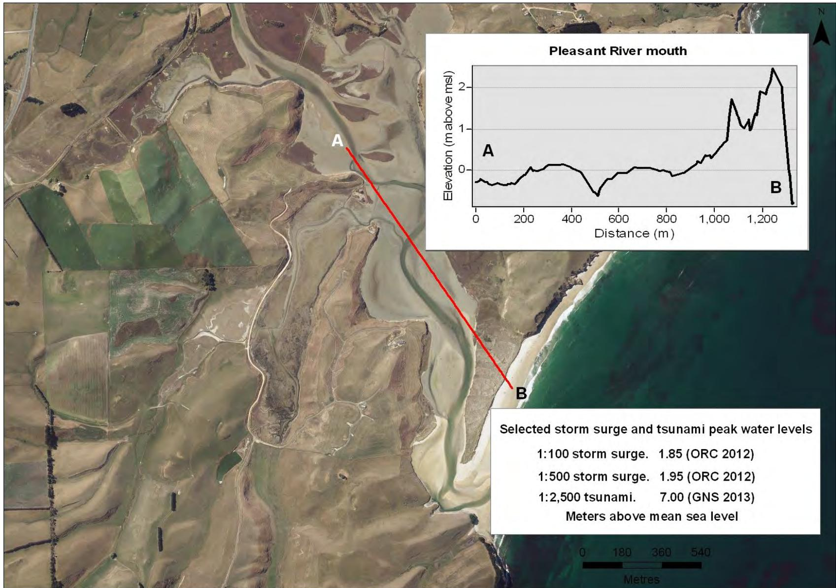
Figure 48. Cross section A-B through the Pleasant River mouth, and peak water levels associated with selected high magnitude storm surge and tsunami events
