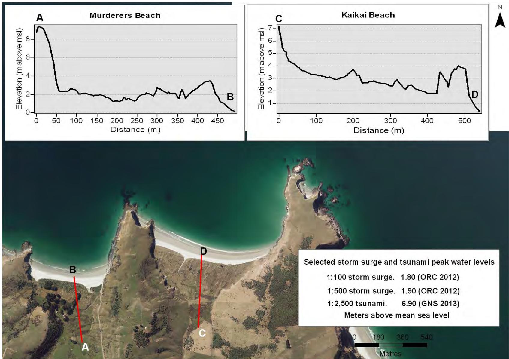
Figure 41. Cross sections A-B through Murdering Beach and C-D through Kaikai Beach, and peak water levels associated with selected high magnitude storm surge and tsunami events
