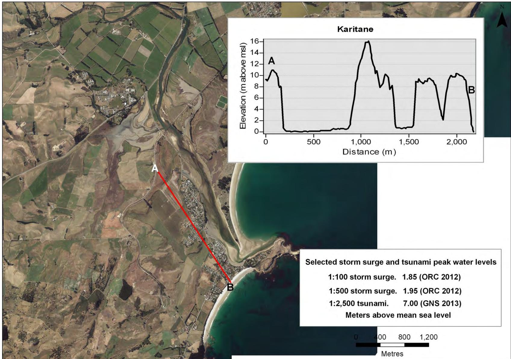
Figure 46. Cross section A-B through Karitane, and peak water levels associated with selected high magnitude storm surge and tsunami events
