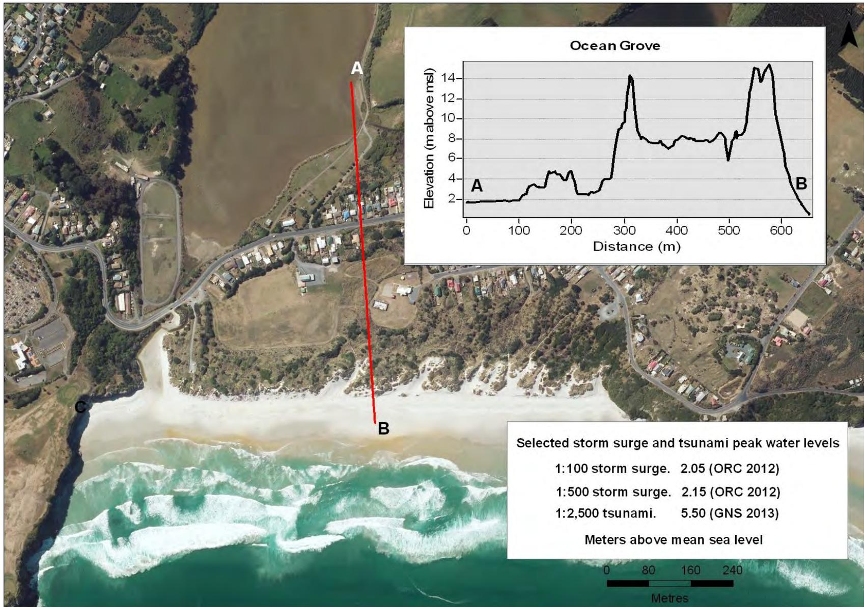
Figure 34. Cross section A-B through Ocean Grove, and peak water levels associated with selected high magnitude storm surge and tsunami events
