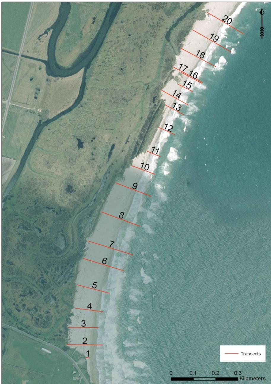
**Figure 64** Transects for erosion/accretion measurements between Kaka Point and Koau Mouth (aerial photograph date: March 2006)
