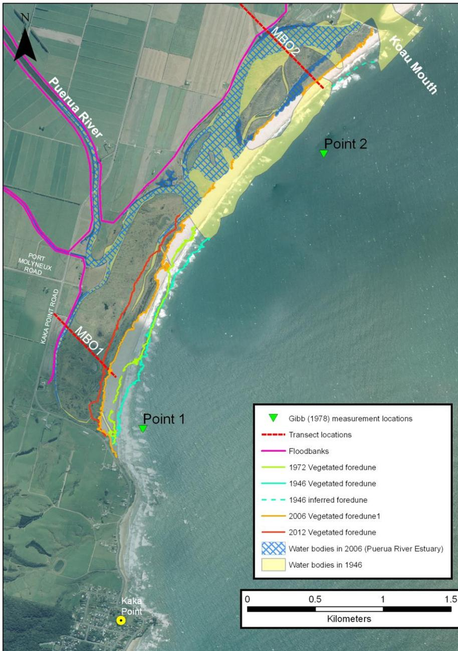
**Figure 21 Mapped shorelines from aerial photography between Kaka Point and the Koau Mouth of the Clutha River/Mata-Au (aerial photograph date: March 2006). The 1946 shoreline at the northern end of this reach is approximate due to the lack of vegetation at that time.**
