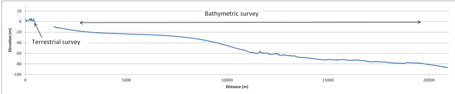
**Figure 46 Combined terrestrial and bathymetric profile of MB7 and MBO7**
