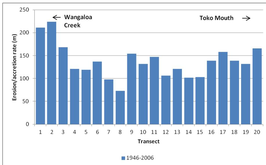
**Figure 43** Rates of coastal erosion/accretion at Measly Beach<sup>17</sup>
