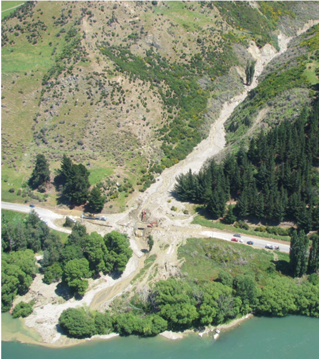
Figure 10: Impacts of the November 2017 debris flow event at Blackjacks Creek, showing the extensive deposition of sediment debris over State Highway 8.
