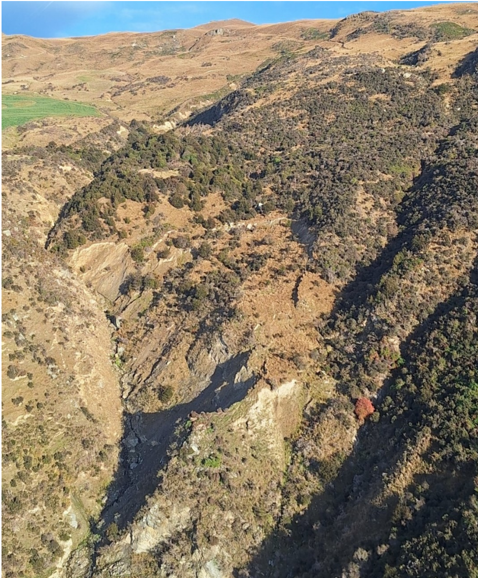
Figure 5: Example of a large active landslide in Golfcourse Creek, currently being undercut and eroded by the channel, which likely supplies sediment to a debris flow during an event. This is a typical situation in these catchments.
