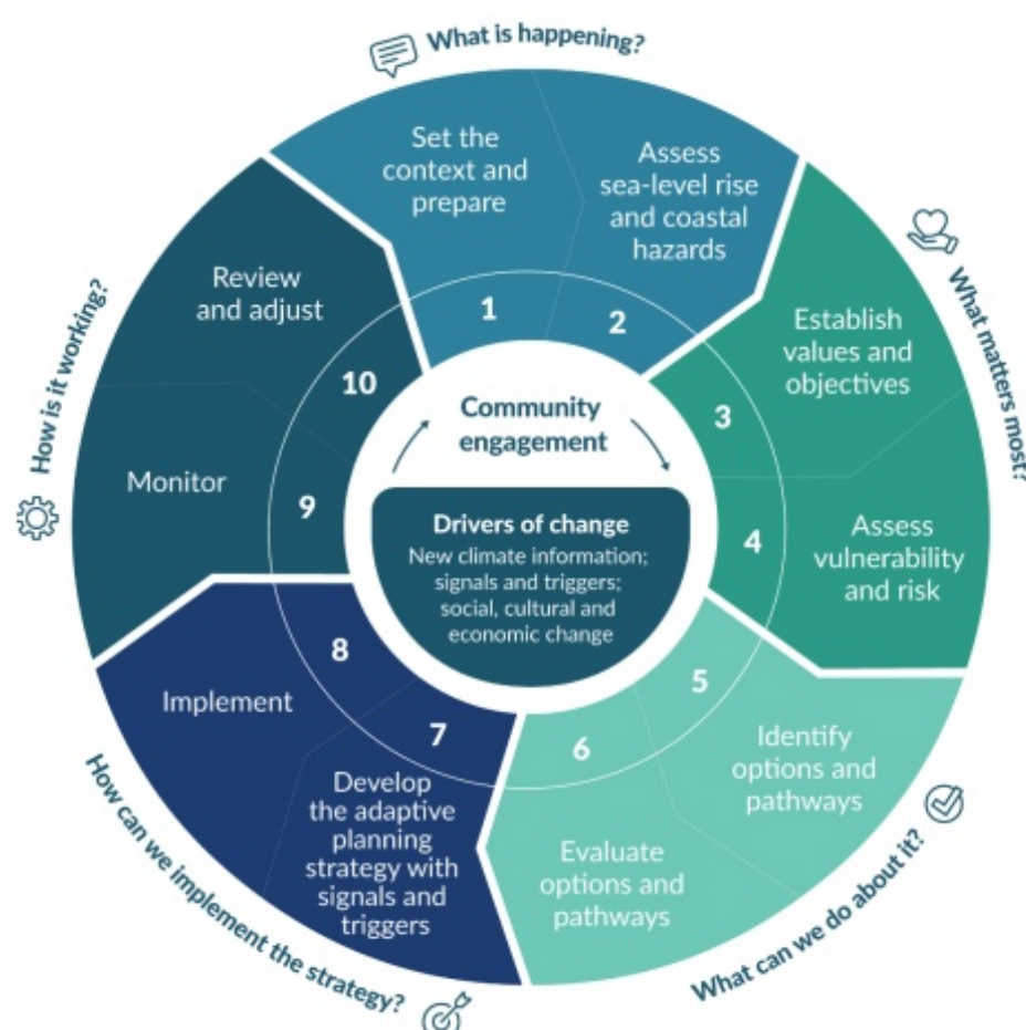
Figure 2: Overview of the 10-step decision cycle from Ministry for Environment (2024) guidance on coastal hazards and climate change.
