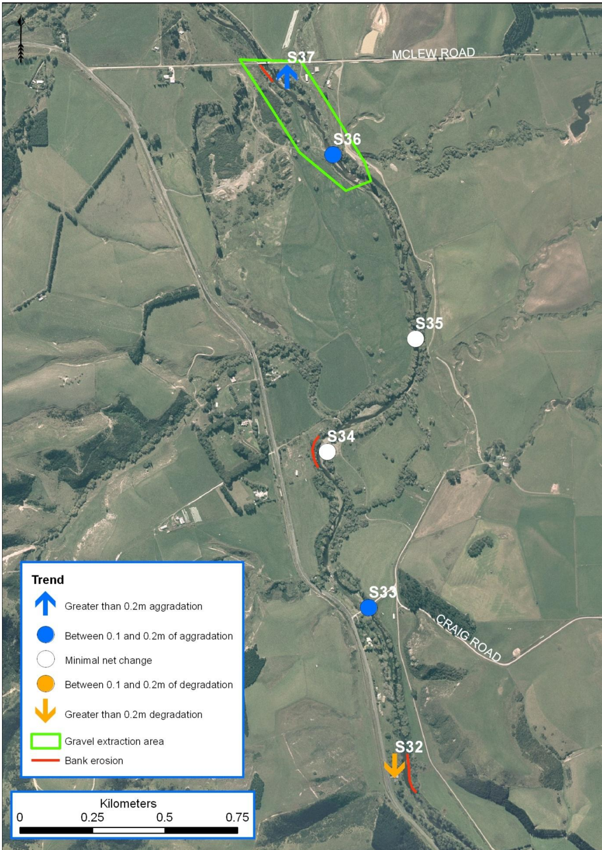
Figure 7. The location of cross-sections S37 to S32 on the Shag River/Waihemo. The white, orange, and blue symbols show the magnitude of MBL change at each cross-section between April 2009 and October 2013. Locations where significant bank erosion (>1m) was observed during this period are shown as red lines. Locations of historic gravel extraction are outlined in green.
