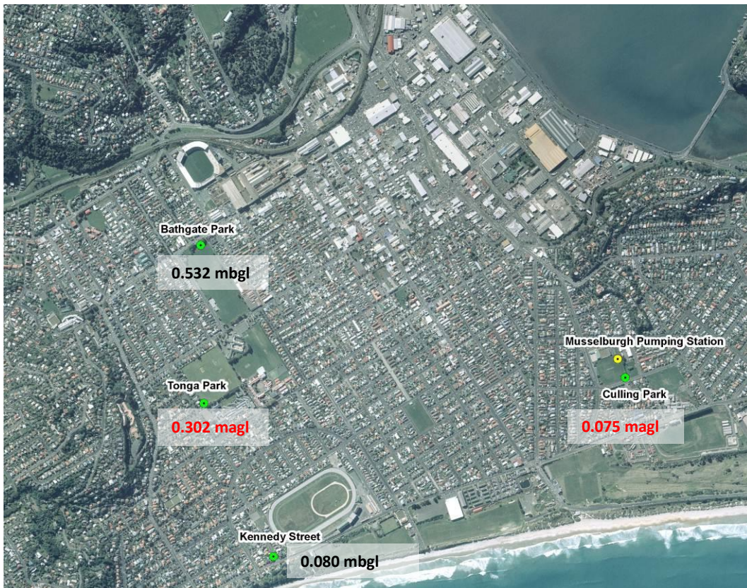
Figure 23: Location of groundwater above and below ground level in South Dunedin. Red – metres above ground level. Black – metres below ground level.
