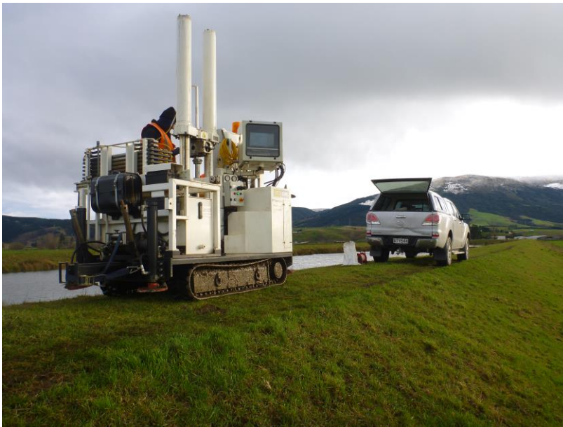
Photograph 1 Cone penetrometer testing of the Waipori floodbank (Lower Taieri Flood Protection Scheme) in June 2015
