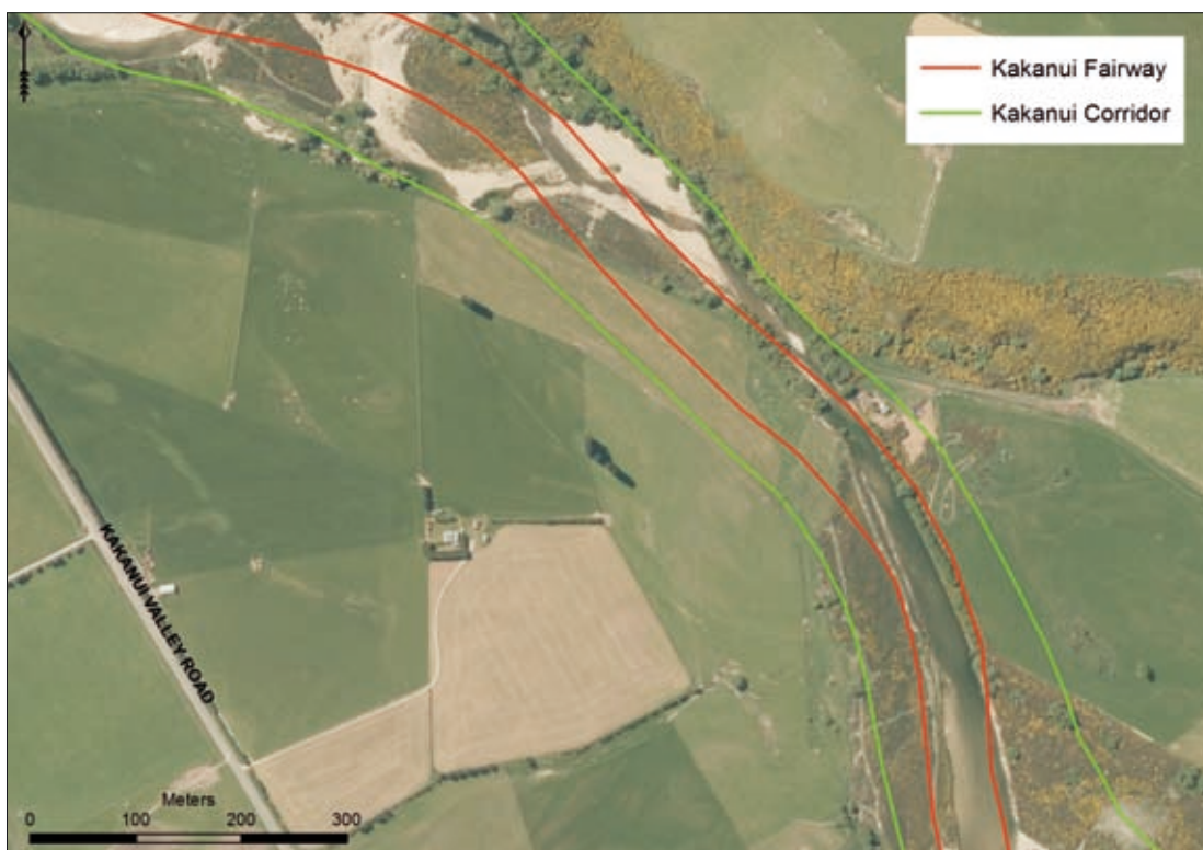
Figure 20. Kakanui River mapped fairway deviating from the current channel alignment (aerial photography collected in the summer of 2013/2014).
