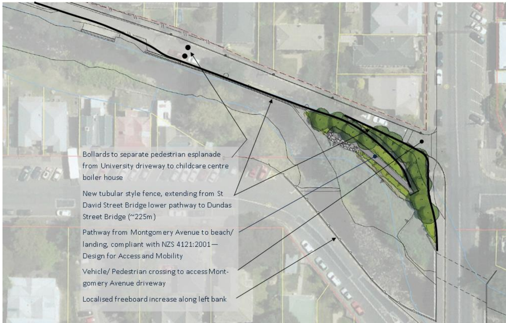
Figure 5 – Detailed View of the Dundas to St David Street Works – Dundas Street Bridge Work
