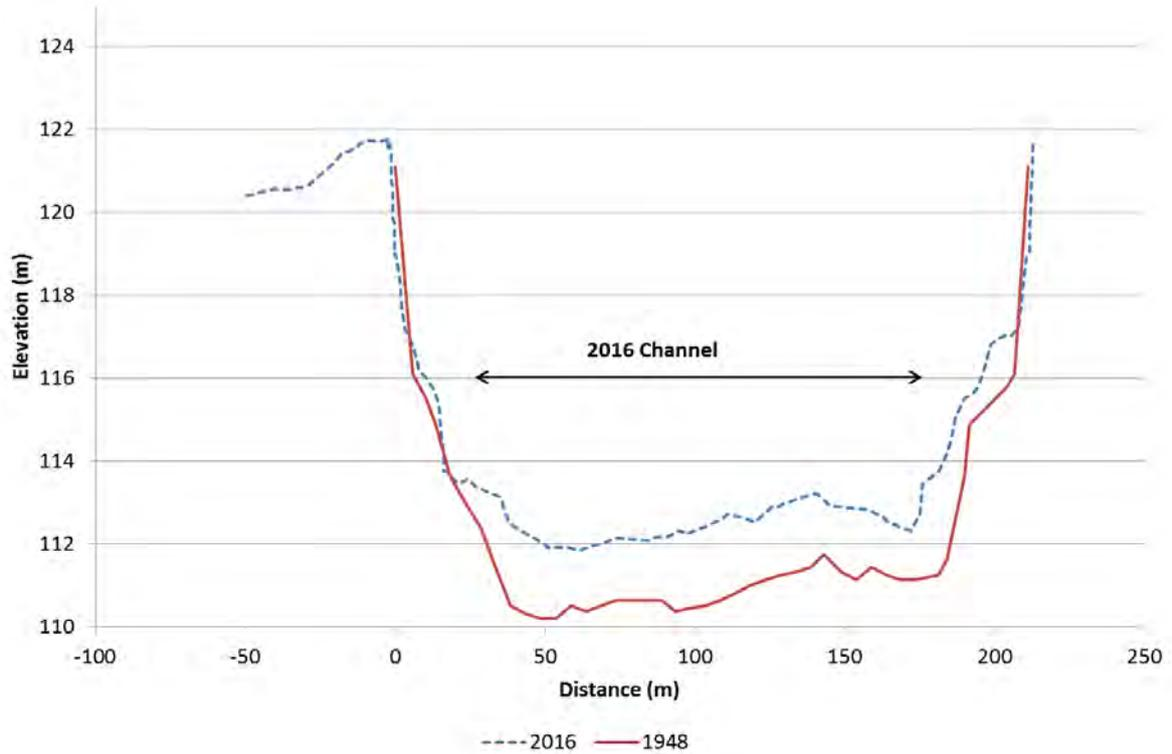
Figure 68. Clutha River/Mata-Au cross-section C22, looking downstream
