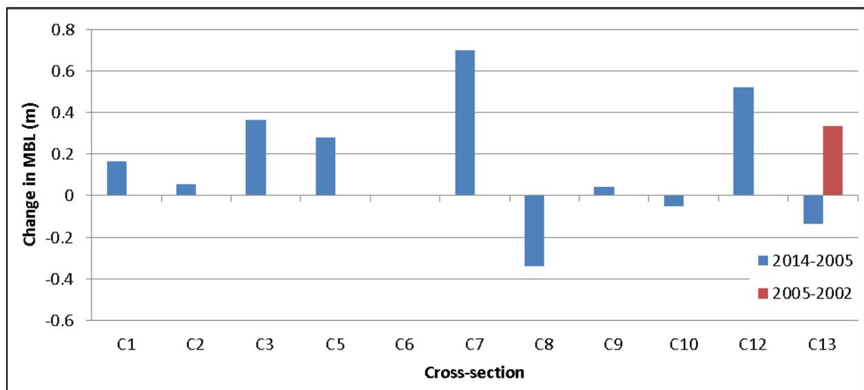
**Figure 7.** Change in MBL at cross-sections on the Clutha River/Mata-Au around Barnego between 2014 and 2005. MBL could not be calculated at all cross-sections in each year due to differing coverage.
