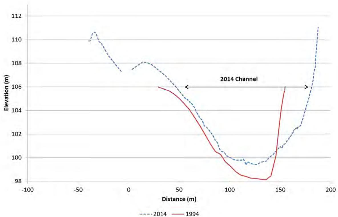
Figure 55. Clutha River/Mata-Au cross-section C9, looking downstream
