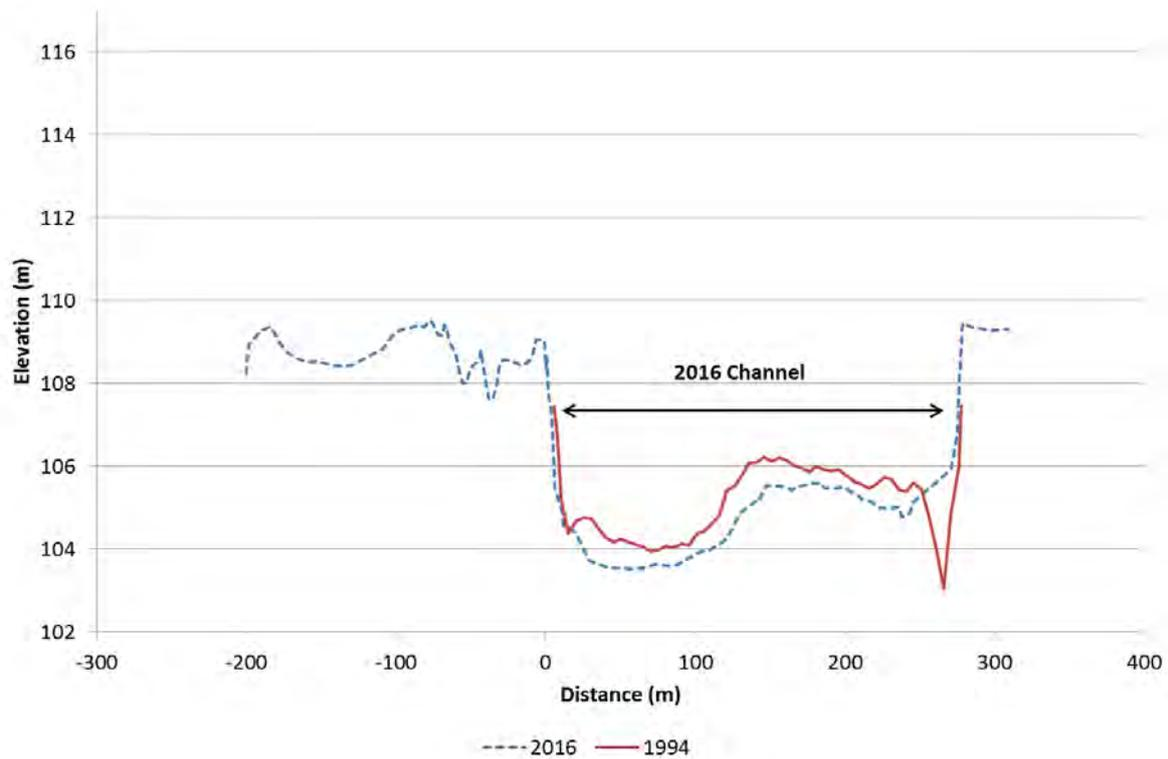
**Figure 62.** Clutha River/Mata-Au cross-section C16, looking downstream
