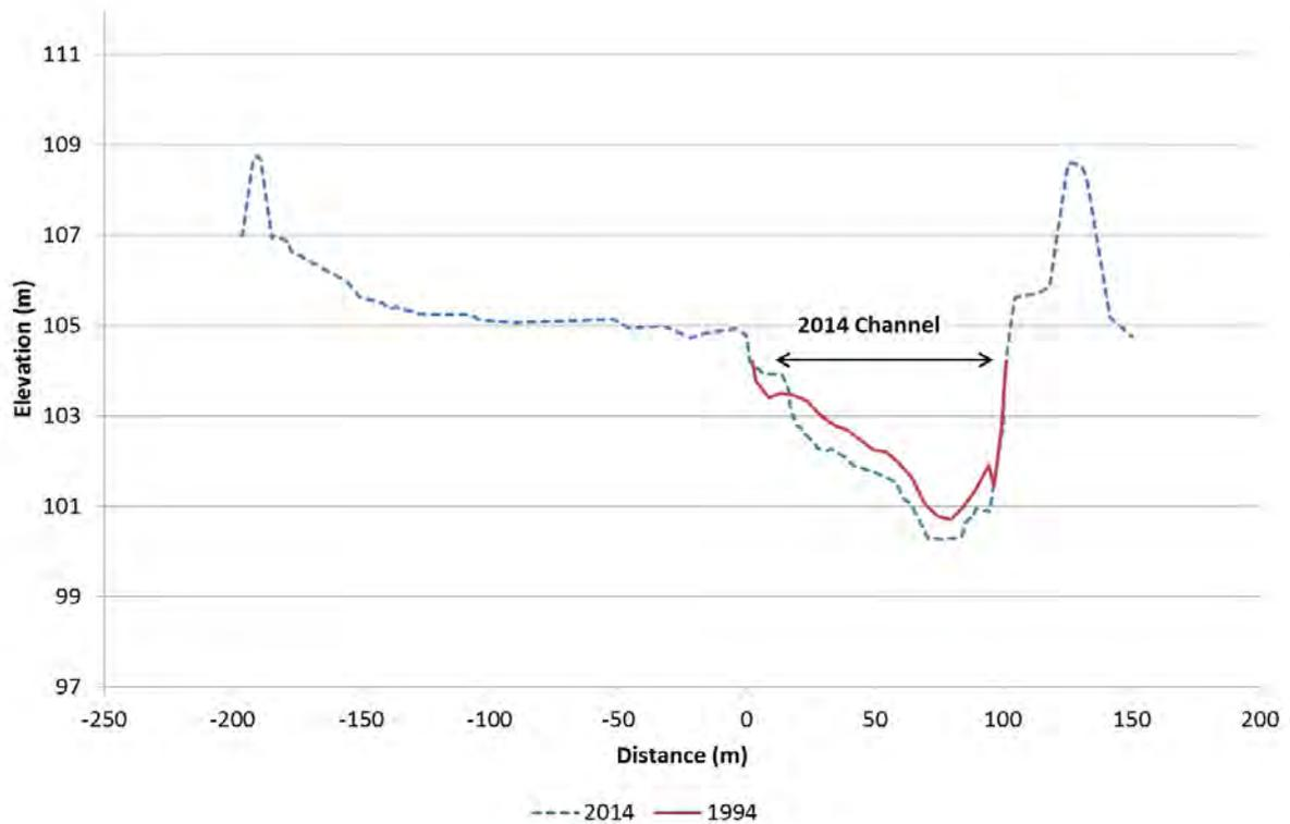
Figure 45. Clutha River/Mata-Au cross-section M10, looking downstream
