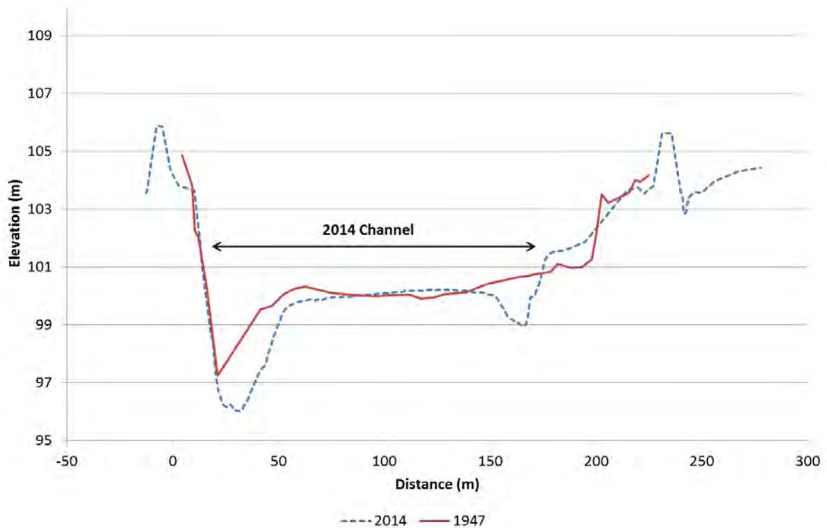
Figure 39. Clutha River/Mata-Au cross-section M94, looking downstream
