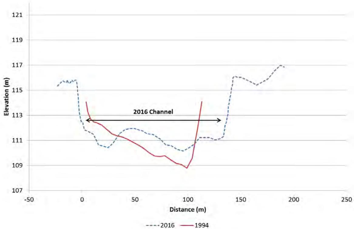
Figure 66. Clutha River/Mata-Au cross-section C20, looking downstream
