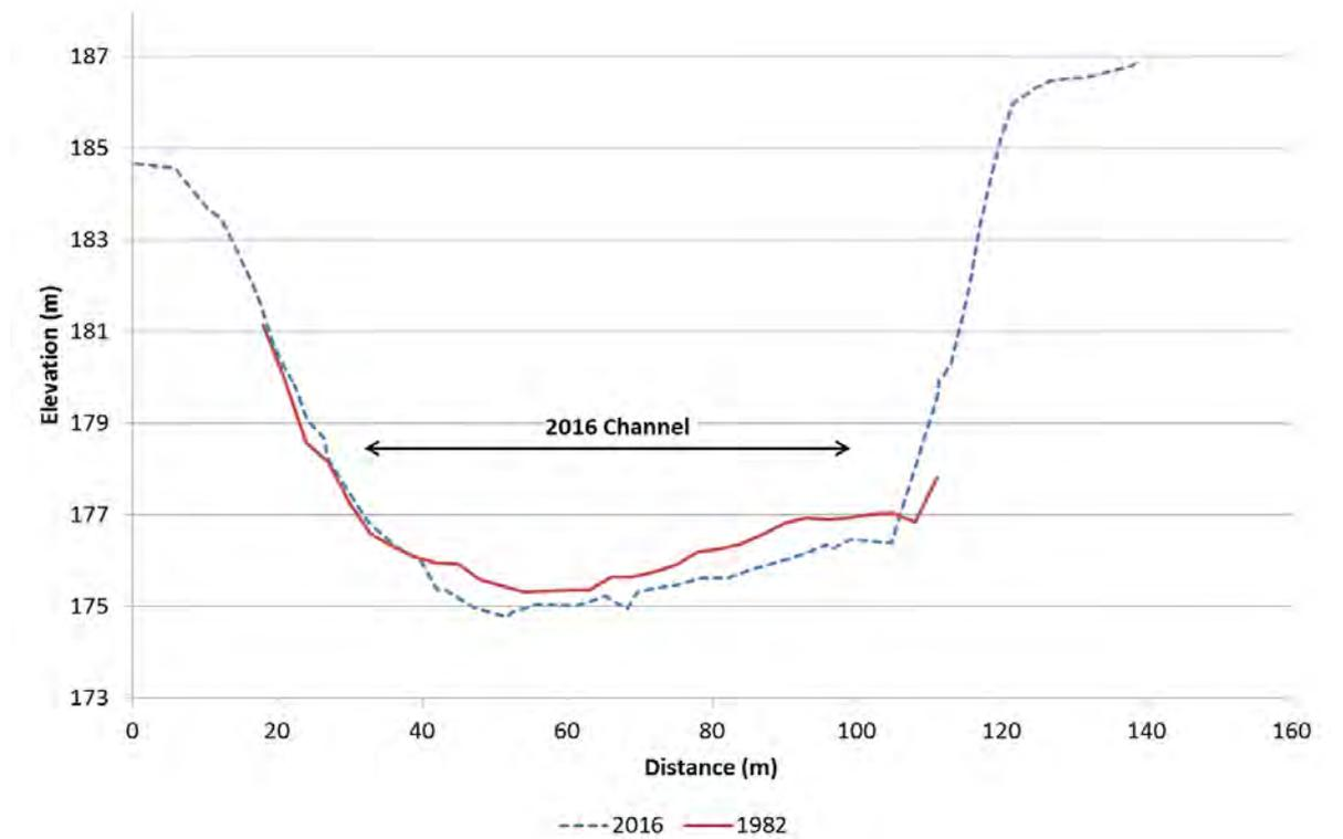
Figure 89. Clutha River/Mata-Au cross-section C42, looking downstream
