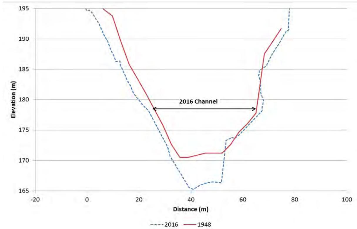
Figure 88. Clutha River/Mata-Au cross-section C41, looking downstream
