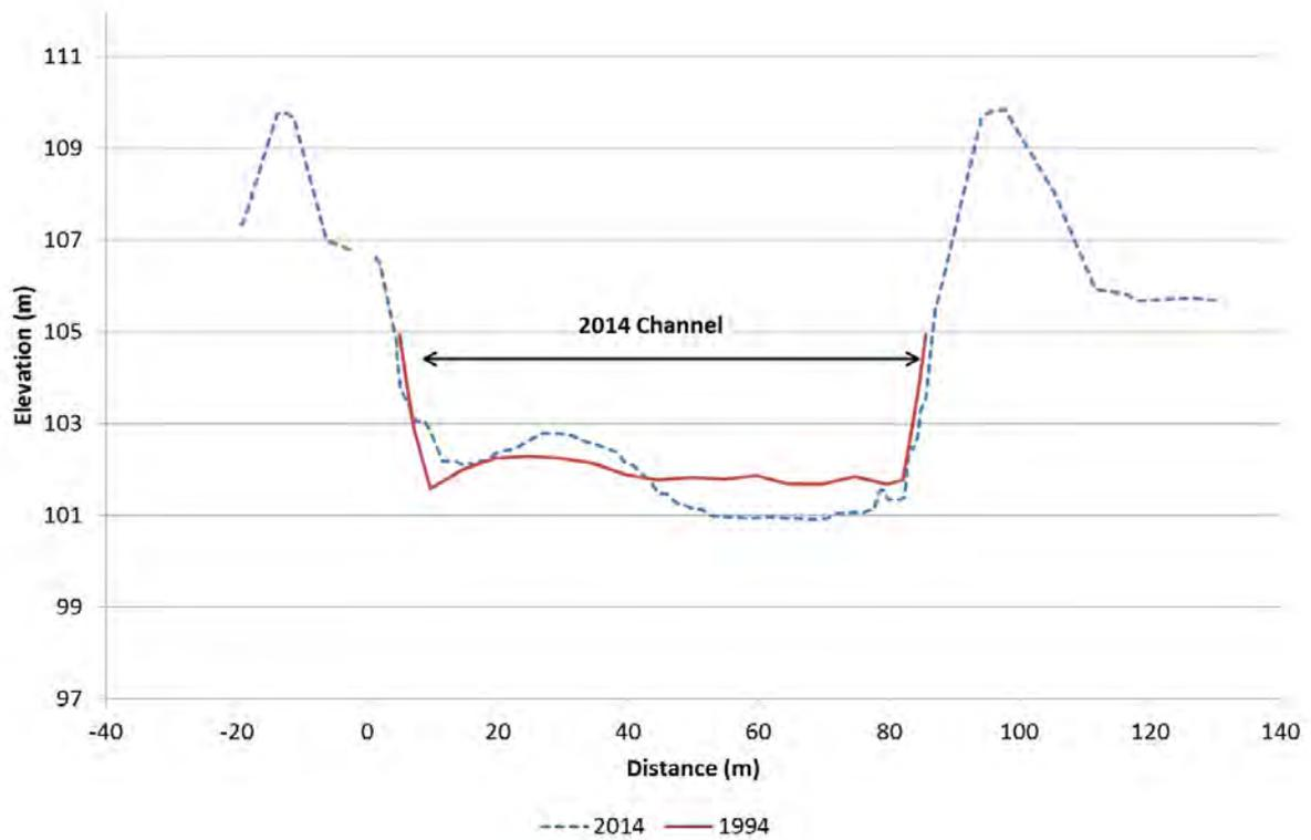
Figure 47. Clutha River/Mata-Au cross-section M12, looking downstream
