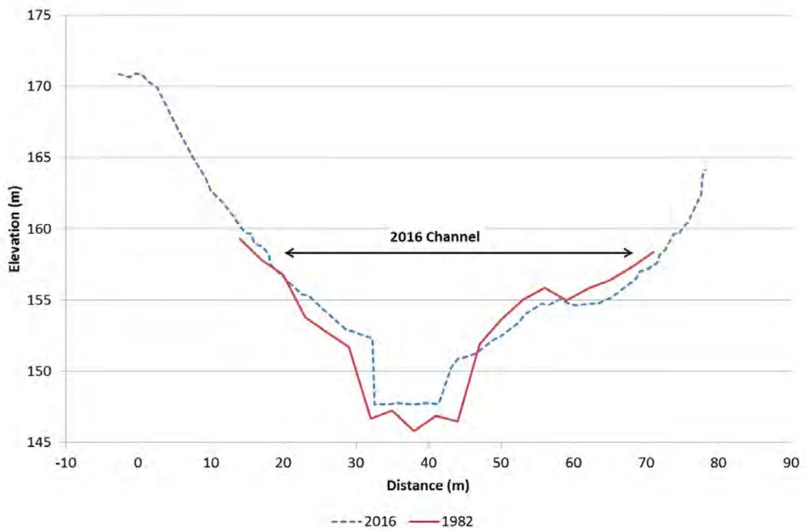
**Figure 79.** Clutha River/Mata-Au cross-section C31, looking downstream
