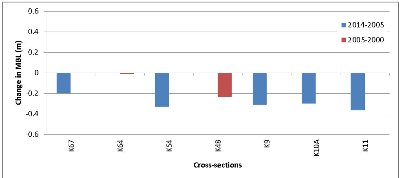
**Figure 6.** Change in MBL at cross-sections on the Koau branch of the Clutha River/Mata-Au between 2014 and 2005 and 2005 and 2000. MBL could not be calculated at all cross-sections in each year due to differing coverage.
