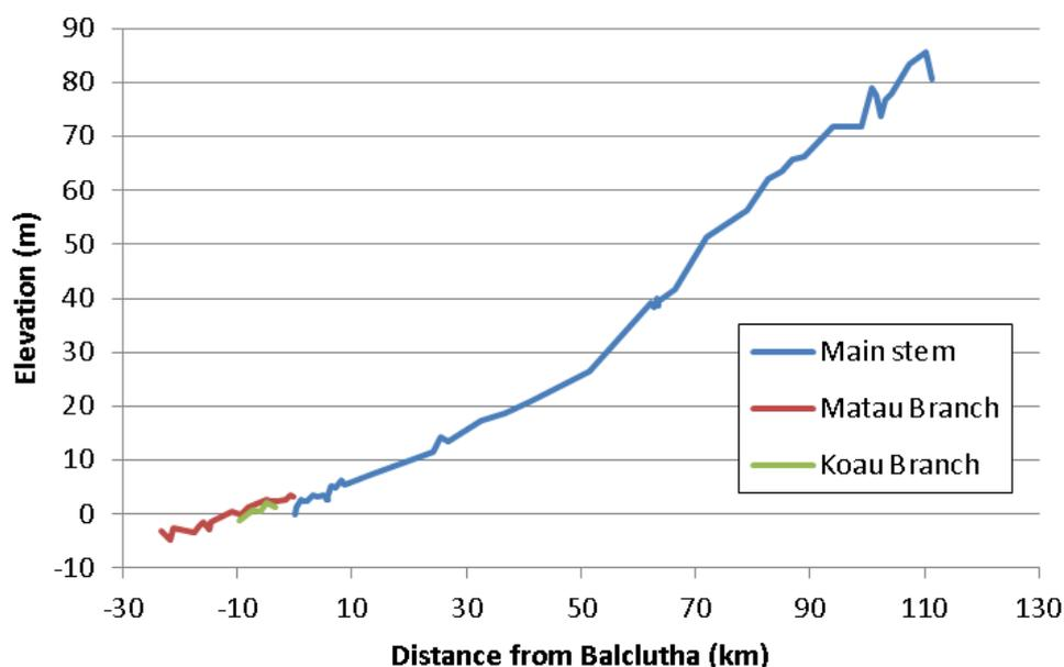
Figure 12. Longitudinal profile (showing the MBL) of the Clutha River/Mata-Au from the latest survey data (2014, 2016).
