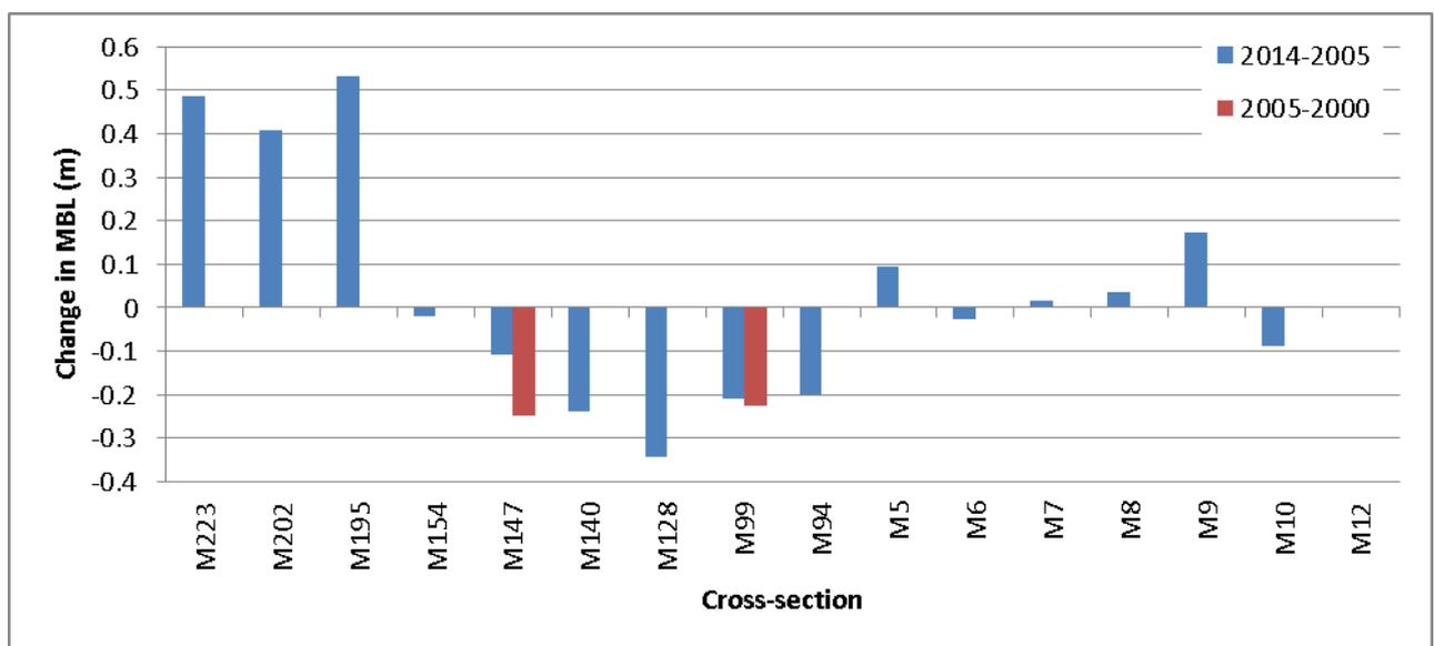
**Figure 4.** Change in MBL at cross-sections on the Matau branch of the Clutha River/Mata-Au between 2014 and 2005 and 2005 and 2000. MBL could not be calculated at all cross-sections in each year due to differing coverage.
