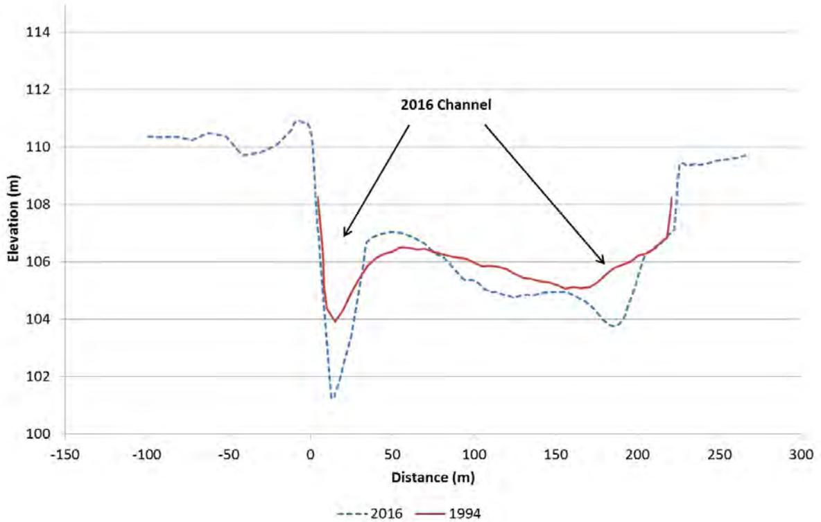
Figure 64. Clutha River/Mata-Au cross-section C18, looking downstream
