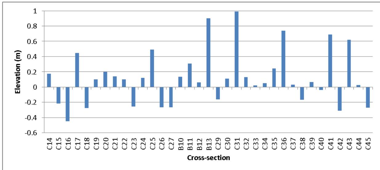
**Figure 9.** Change in MBL at cross-sections on the Clutha River/Mata-Au for the reach between Barnego and Roxburgh Dam between the years 2016 and 2007.
