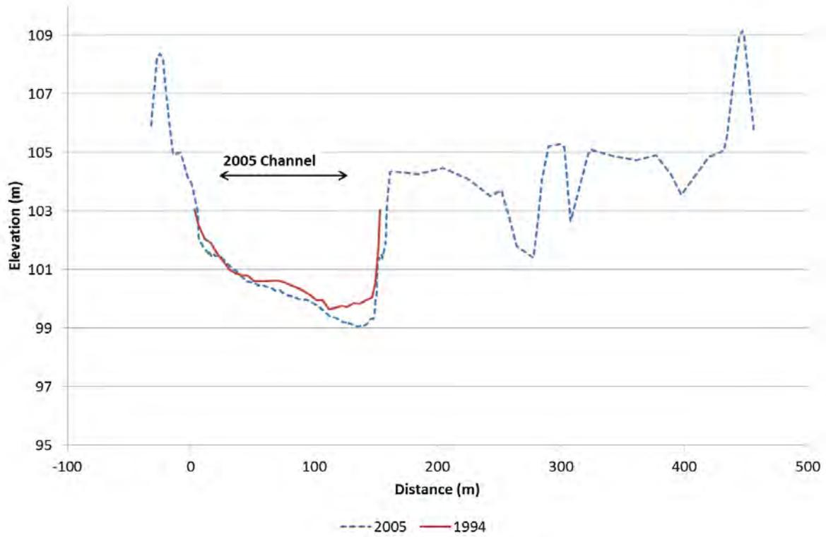
Figure 26. Clutha River/Mata-Au cross-section K10, looking downstream
