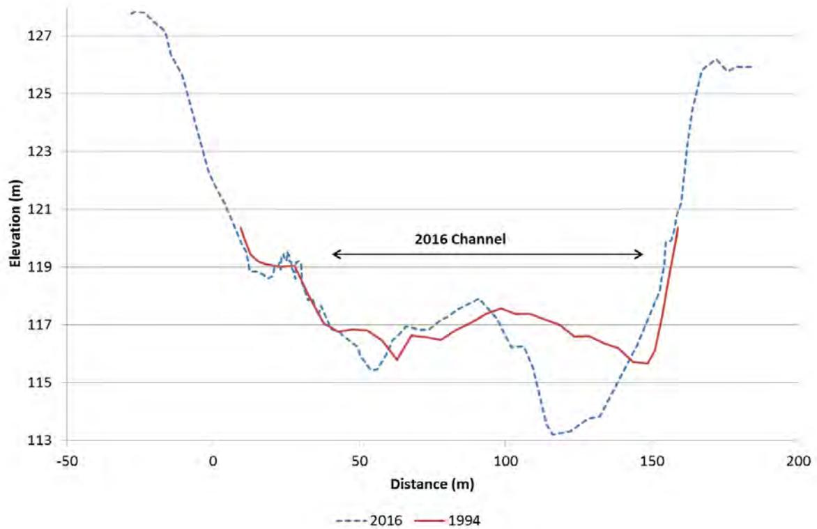
**Figure 70.** Clutha River/Mata-Au cross-section C24, looking downstream
