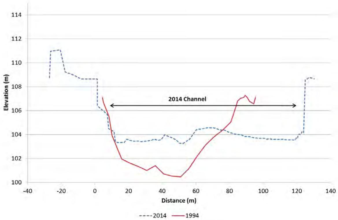
**Figure 58. Clutha River/Mata-Au cross-section C12, looking downstream**
