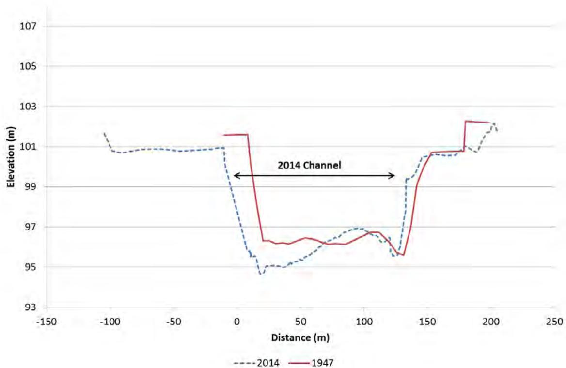
Figure 31. Clutha River/Mata-Au cross-section M223, looking downstream
