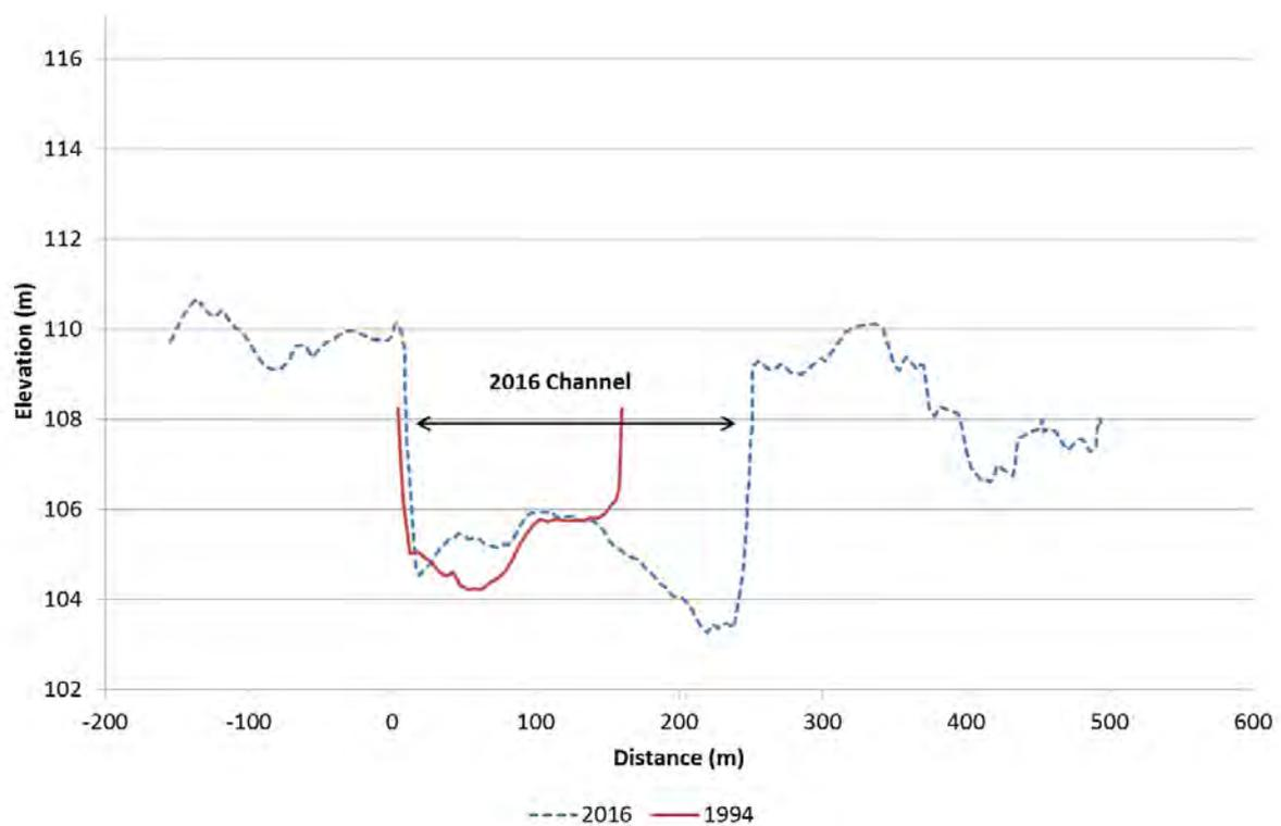
**Figure 63.** Clutha River/Mata-Au cross-section C17, looking downstream
