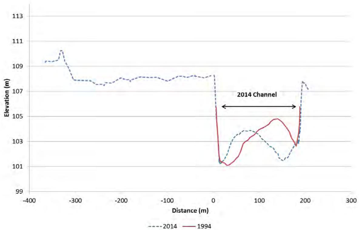
Figure 54. Clutha River/Mata-Au cross-section C8, looking downstream
