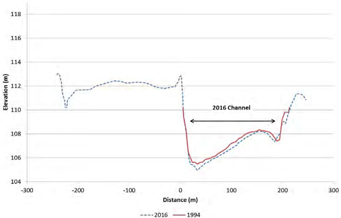
Figure 65. Clutha River/Mata-Au cross-section C19, looking downstream
