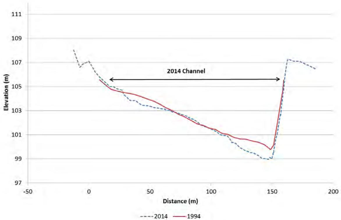
Figure 53. Clutha River/Mata-Au cross-section C7, looking downstream
