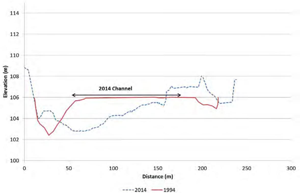
Figure 57. Clutha River/Mata-Au cross-section C11, looking downstream
