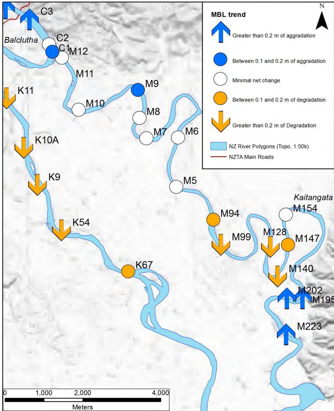
Figure 5. The location of cross-section on the Clutha River/Mata-Au delta. The white, orange, and blue symbols show the magnitude of MBLchange at each cross-section between the two recent cross-section surveys (2014 – 2005).
