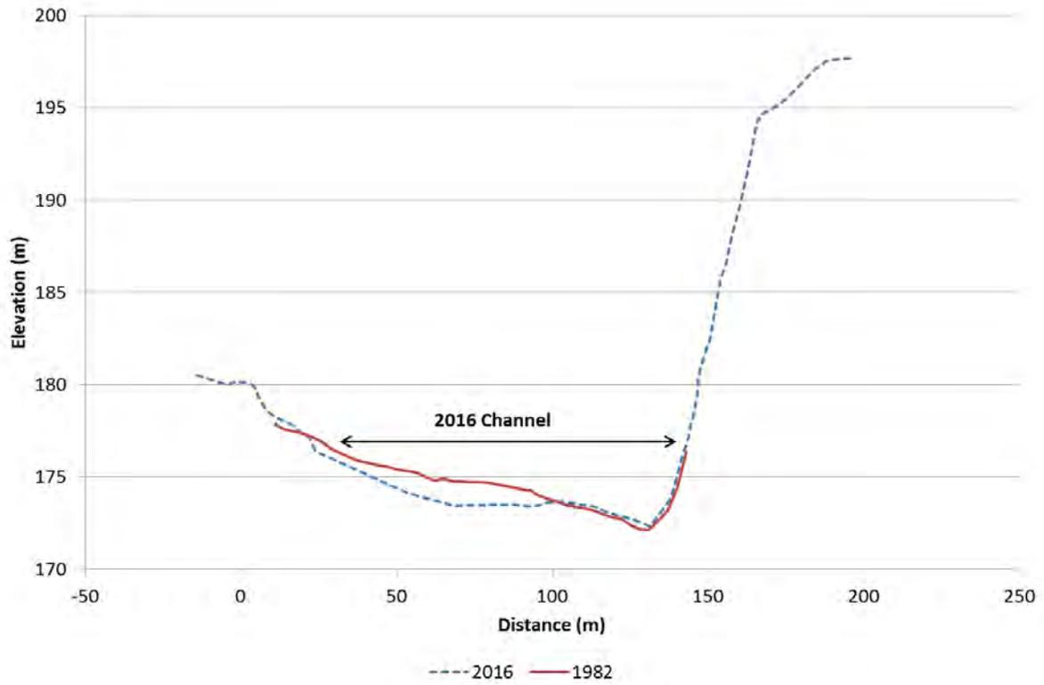
Figure 86. Clutha River/Mata-Au cross-section C38, looking downstream
