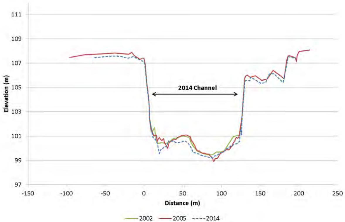
**Figure 104.** Clutha River/Mata-Au cross-section K11, looking downstream
