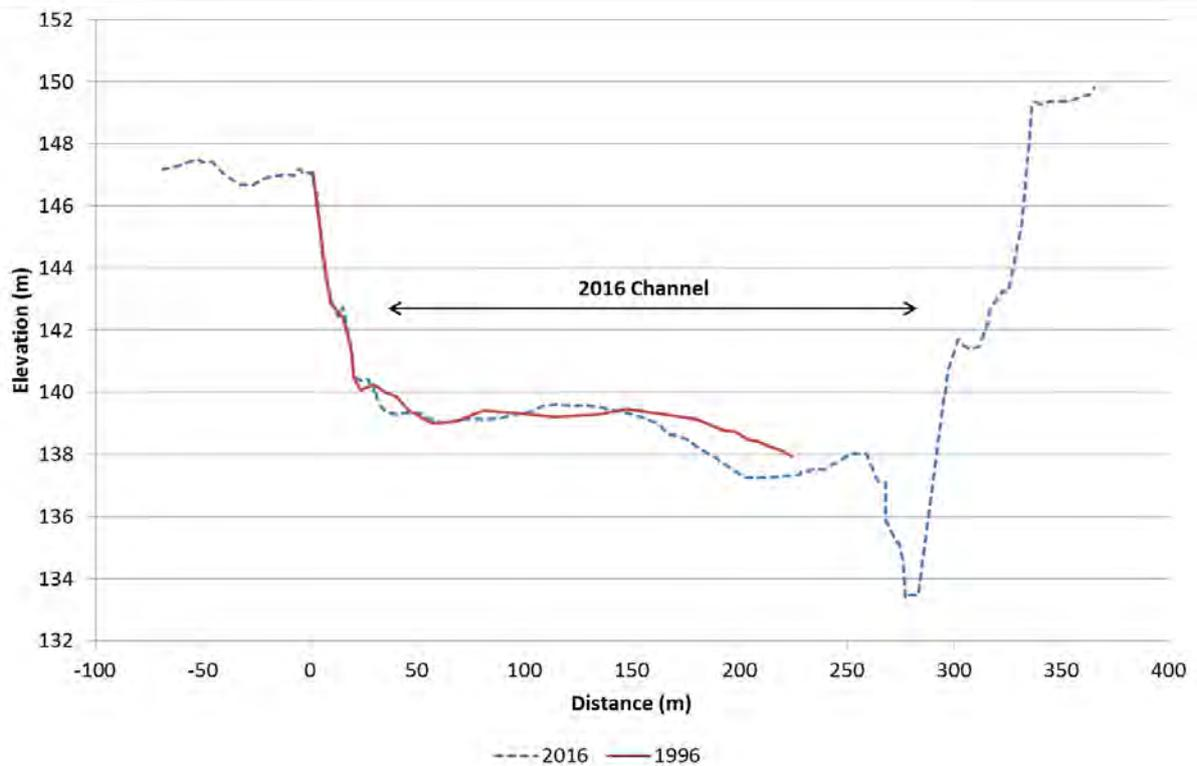
**Figure 77.** Clutha River/Mata-Au cross-section B13, looking downstream
