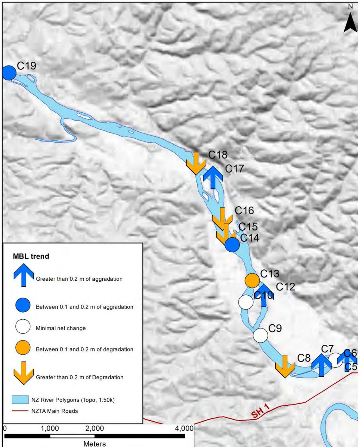
**Figure 8.** The location of cross-section on the Clutha River/Mata-Au upstream of Balclutha. The white, orange, and blue symbols show the magnitude of MBLchange at each cross-section between the two recent cross-section surveys (2014 – 2005, 2016 - 2007).
