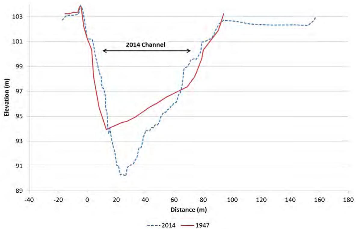
Figure 34. Clutha River/Mata-Au cross-section M154, looking downstream
