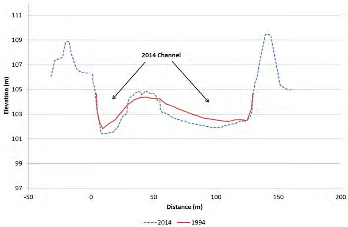
Figure 46. Clutha River/Mata-Au cross-section M11, looking downstream
