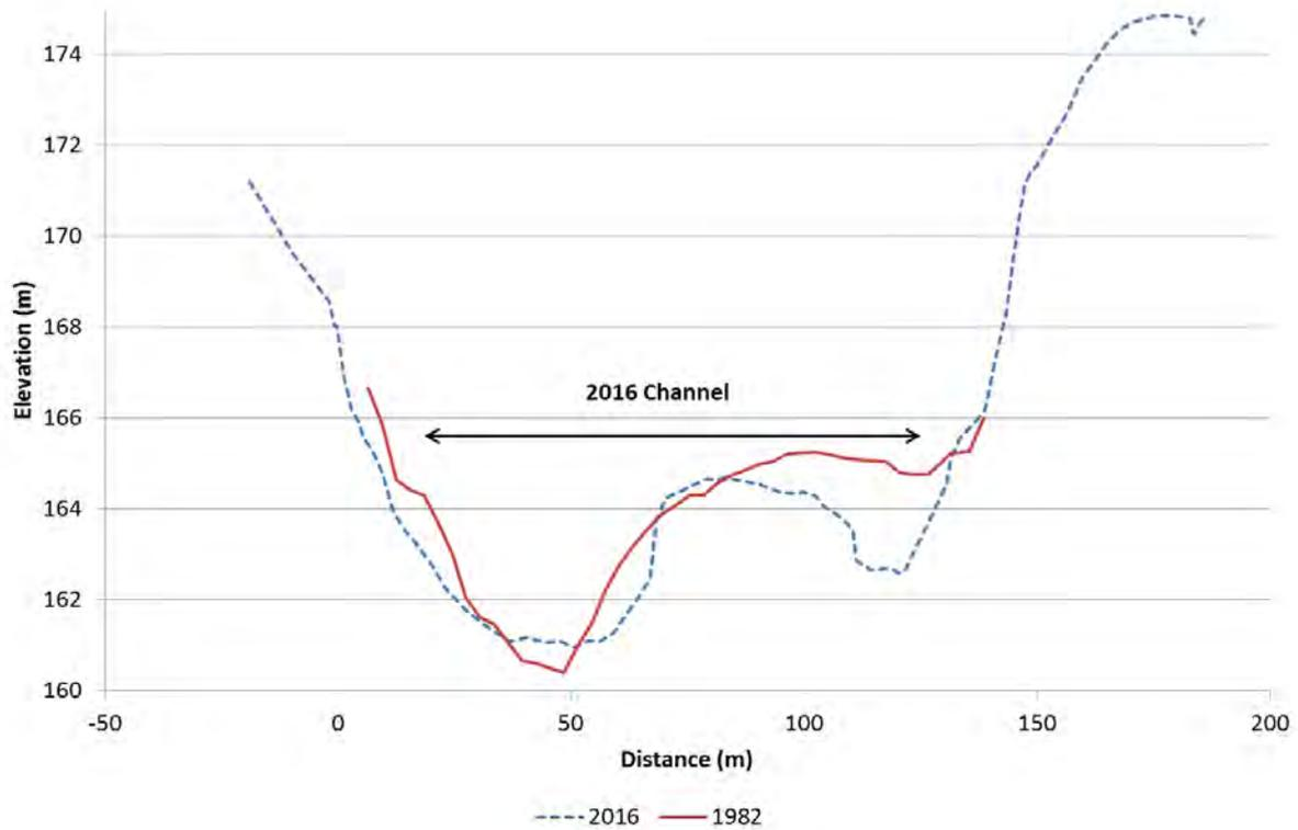
Figure 82. Clutha River/Mata-Au cross-section C34, looking downstream
