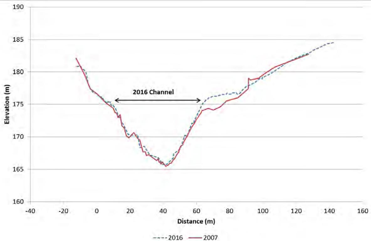
Figure 85. Clutha River/Mata-Au cross-section C37, looking downstream
