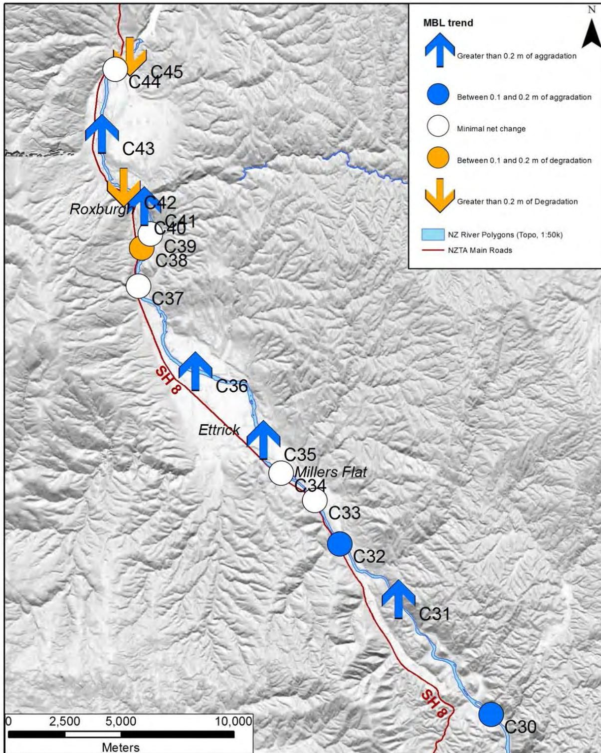
Figure 11. The location of cross-section on the Clutha River/Mata-Au between Beaumont and Roxburgh Dam. The white, orange, and blue symbols show the magnitude of MBLchange at each cross-section between the two recent cross-section surveys (2014 – 2005).
