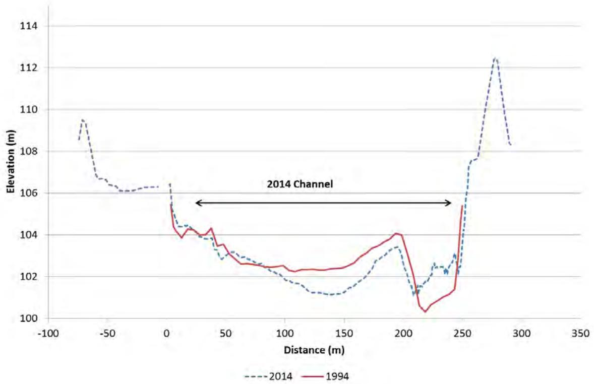
Figure 52. Clutha River/Mata-Au cross-section C6, looking downstream
