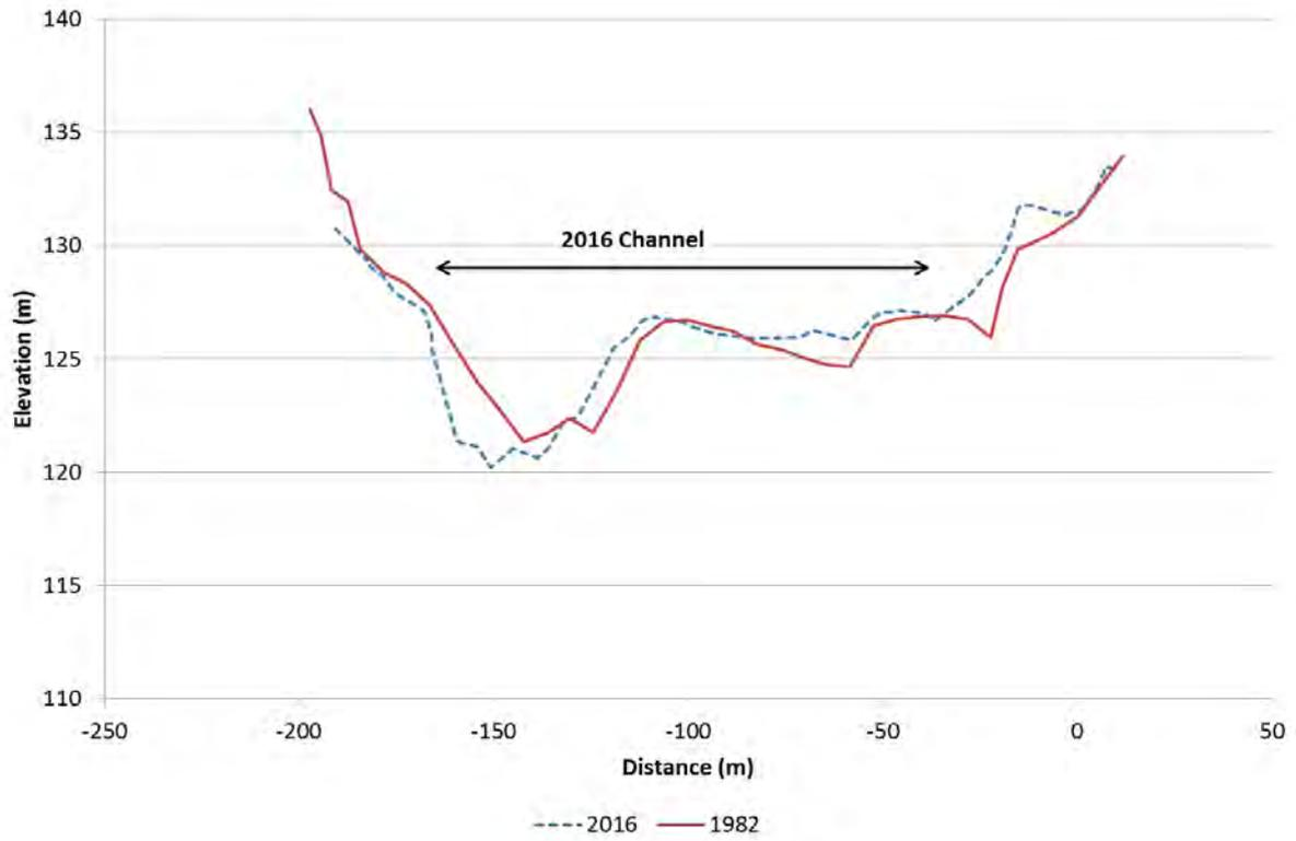
Figure 72. Clutha River/Mata-Au cross-section C26, looking downstream
