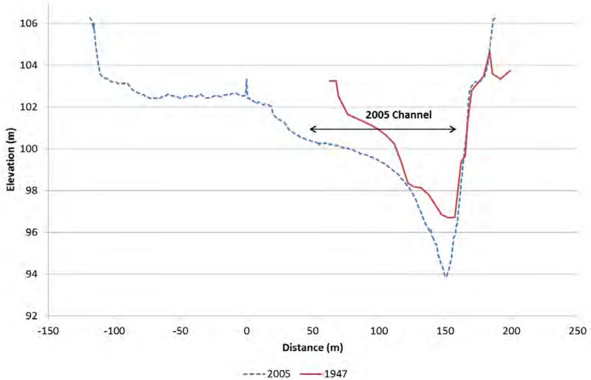
Figure 24. Clutha River/Mata-Au cross-section K64, looking downstream
