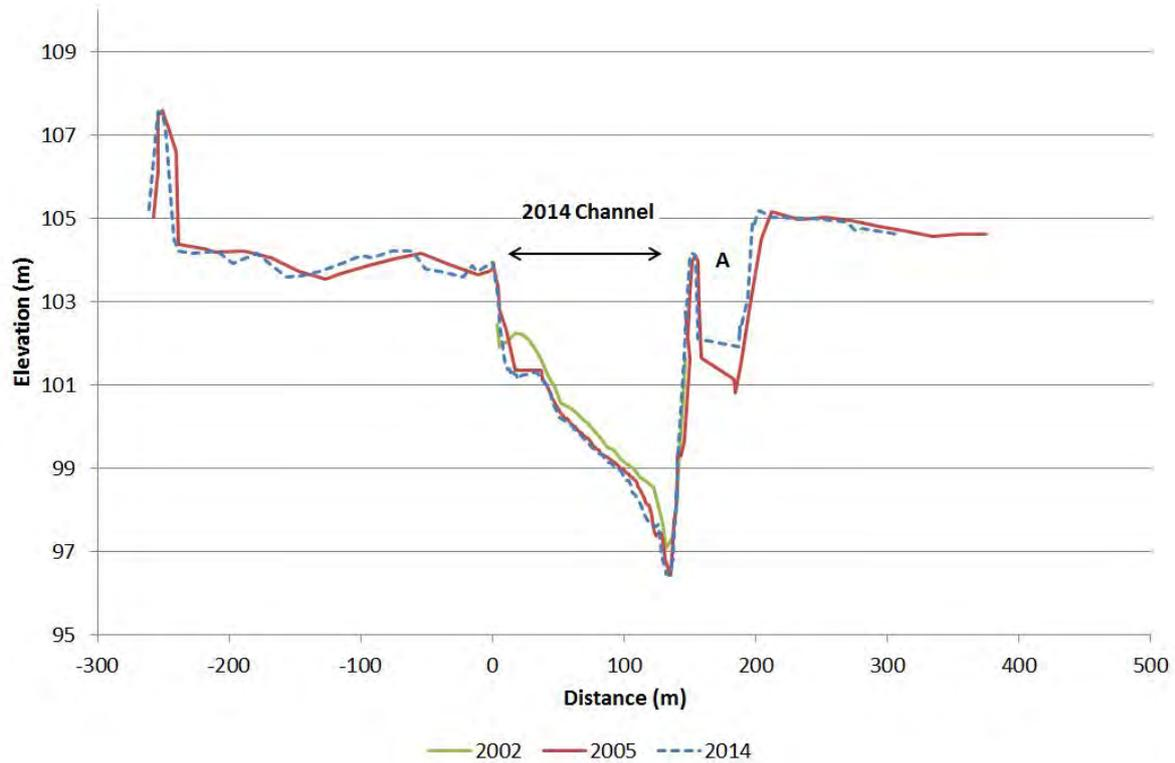
**Figure 99.** Clutha River/Mata-Au cross-section K9, looking downstream
