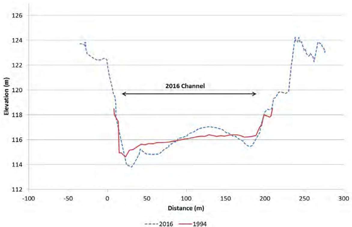
Figure 69. Clutha River/Mata-Au cross-section C23, looking downstream
