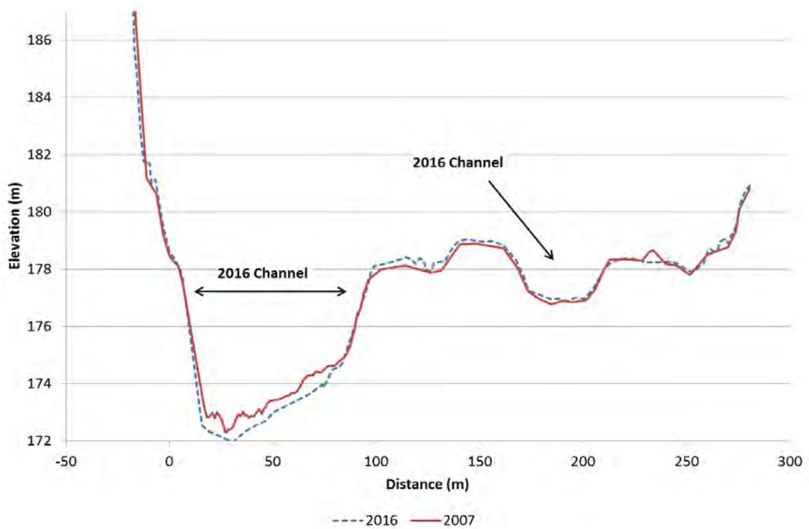
Figure 87. Clutha River/Mata-Au cross-section C39, looking downstream
