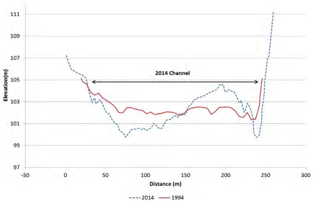
Figure 49. Clutha River/Mata-Au cross-section C2, looking downstream
