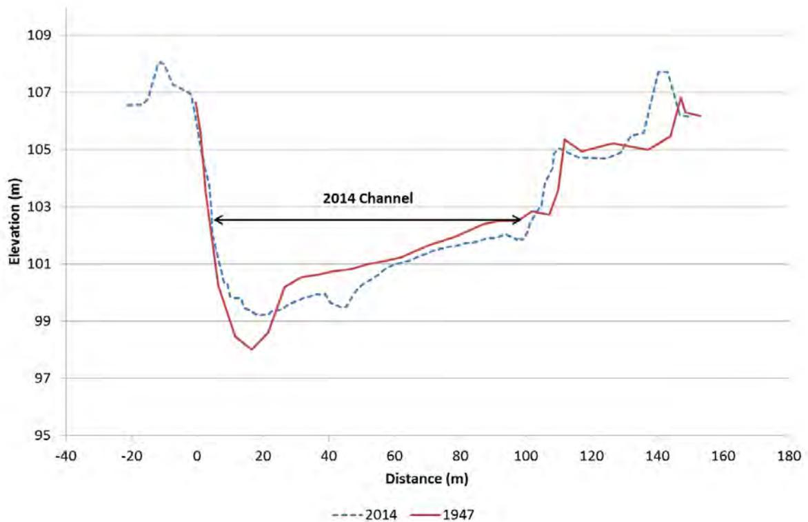
Figure 43. Clutha River/Mata-Au cross-section M8, looking downstream
