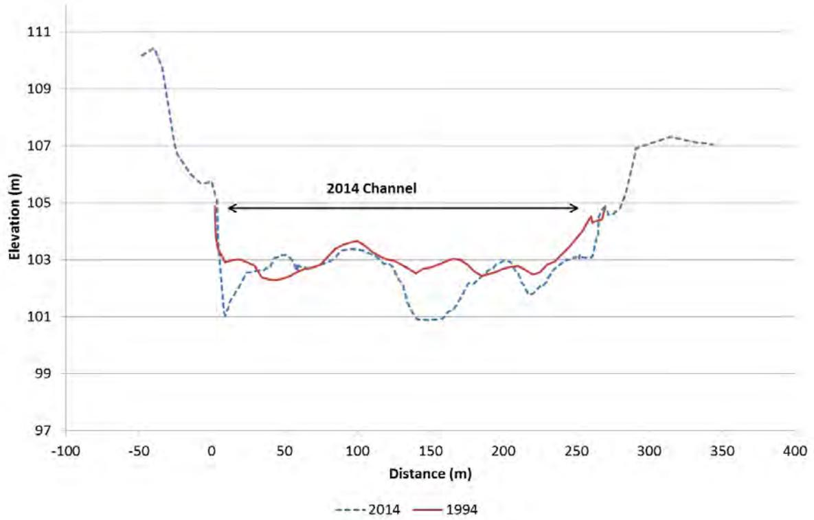
Figure 48. Clutha River/Mata-Au cross-section C1, looking downstream
