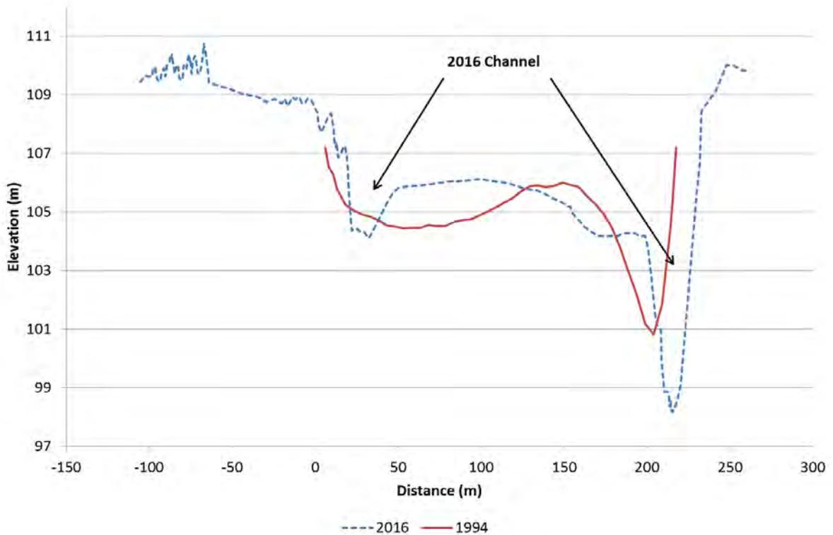
Figure 61. Clutha River/Mata-Au cross-section C15, looking downstream
