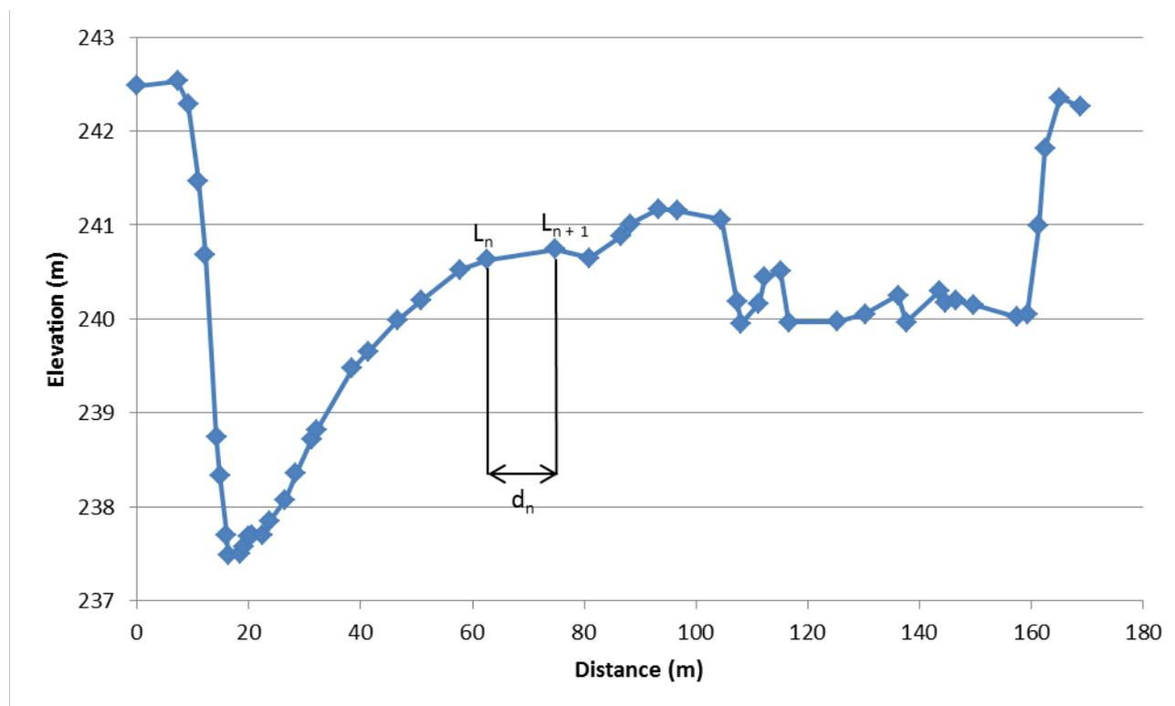
Figure 239. MBL calculation - definition of variables
