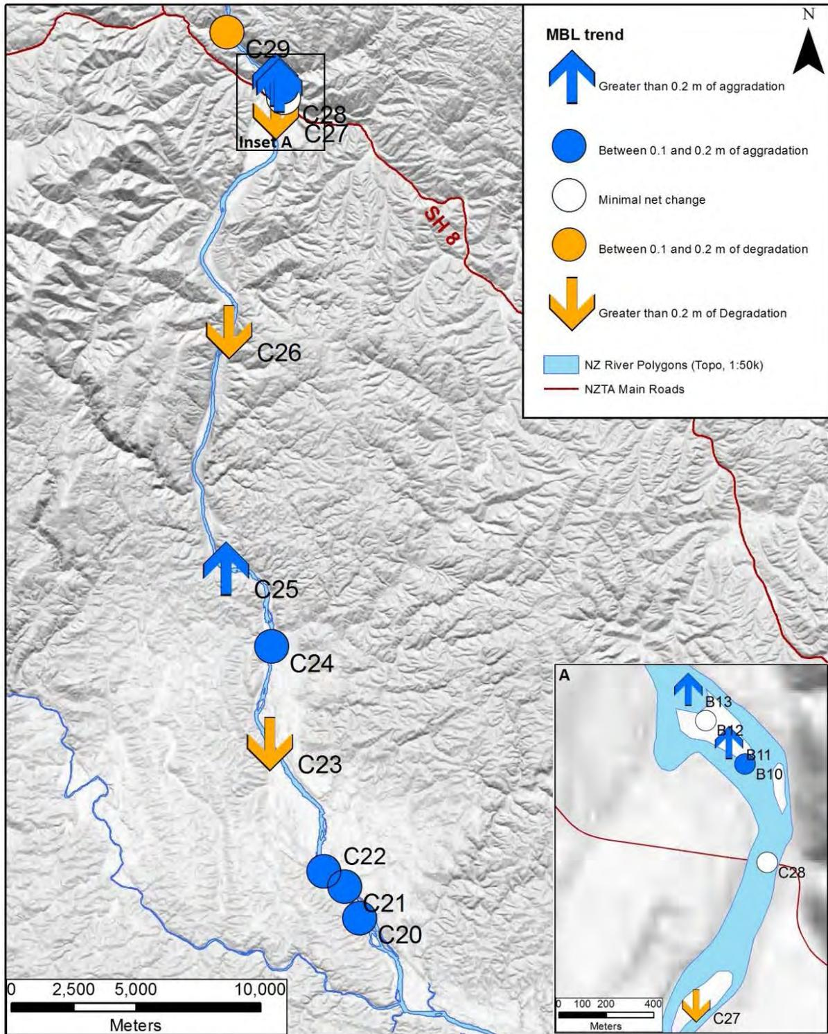
**Figure 10.** The location of cross-section on the Clutha River/Mata-Au between Clydevale and Beaumont. The white, orange, and blue symbols show the magnitude of MBLchange at each cross-section between the two recent cross-section surveys (2016 – 2007).
