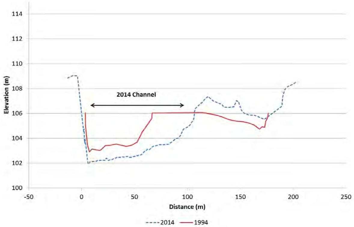
Figure 56. Clutha River/Mata-Au cross-section C10, looking downstream
