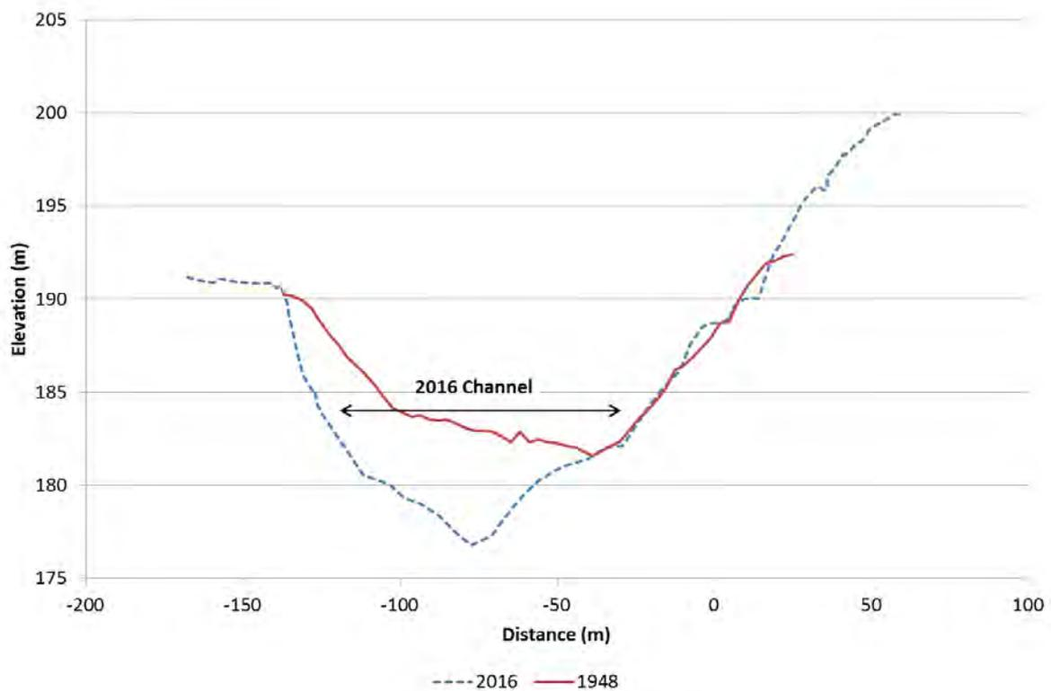
**Figure 91.** Clutha River/Mata-Au cross-section C44, looking downstream
