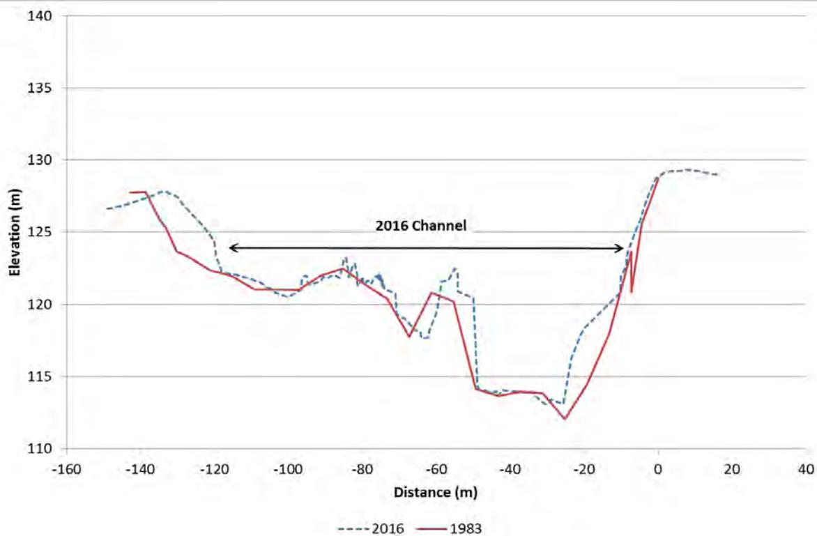
**Figure 71.** Clutha River/Mata-Au cross-section C25, looking downstream
