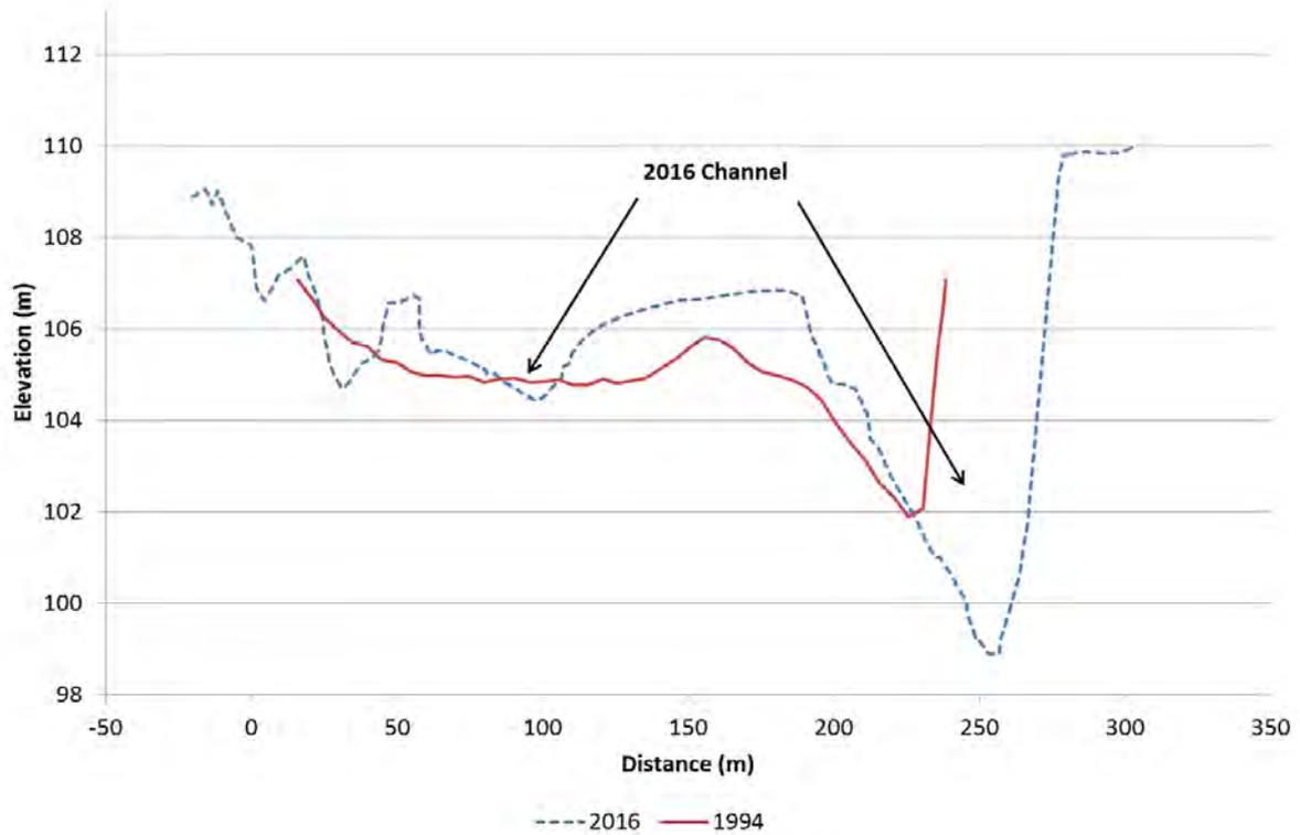
Figure 60. Clutha River/Mata-Au cross-section C14, looking downstream
