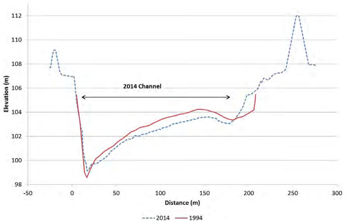
Figure 51. Clutha River/Mata-Au cross-section C5, looking downstream
