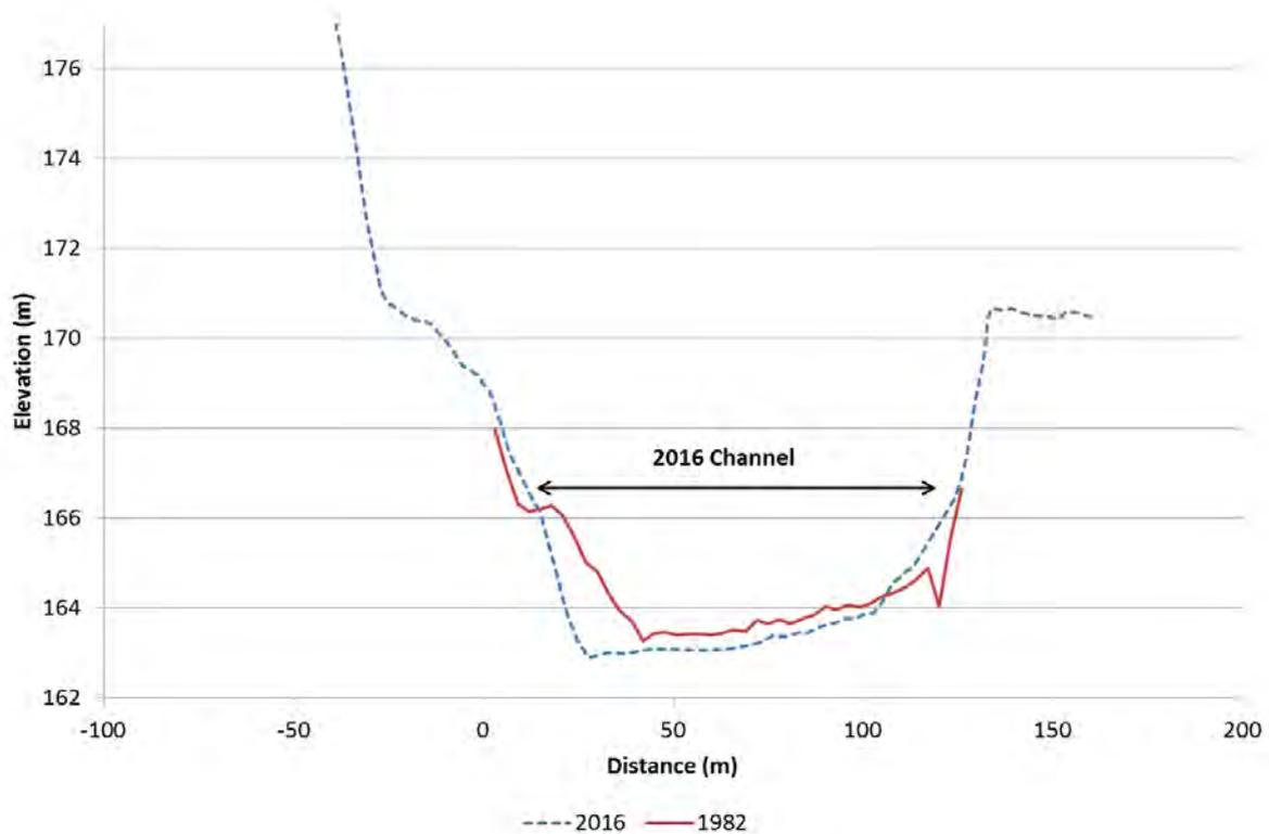
Figure 83. Clutha River/Mata-Au cross-section C35, looking downstream
