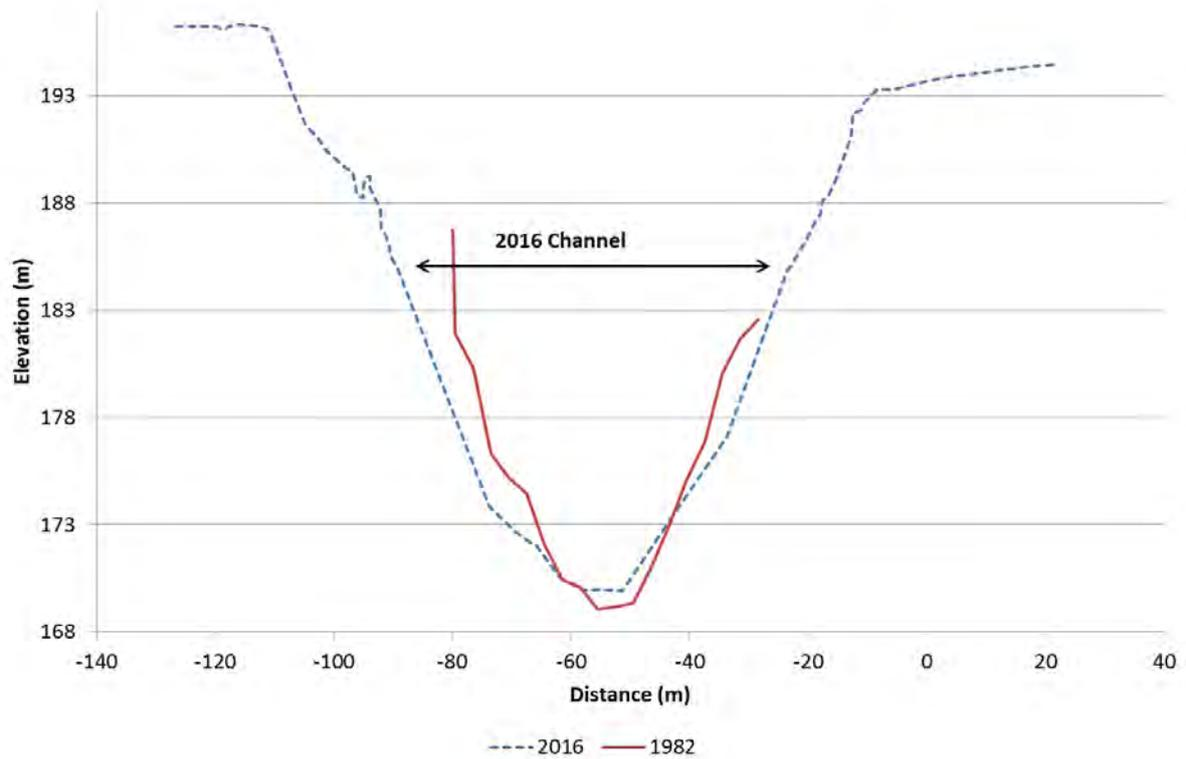
Figure 92. Clutha River/Mata-Au cross-section C45, looking downstream
