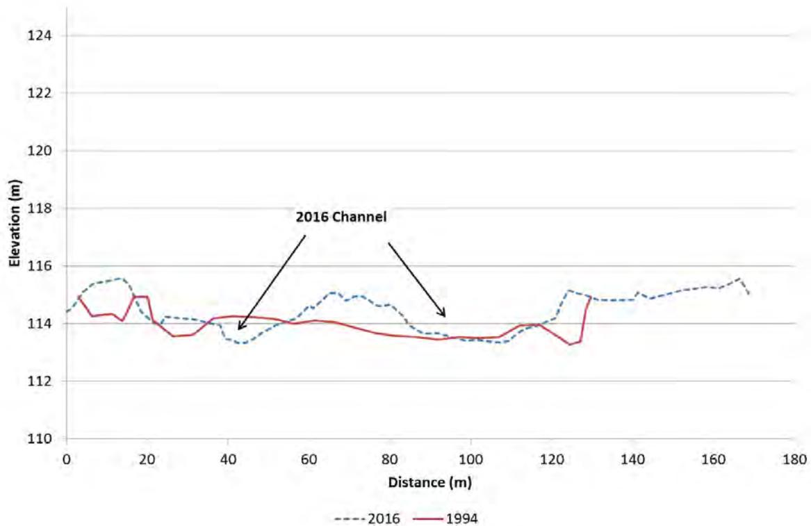
Figure 67. Clutha River/Mata-Au cross-section C21, looking downstream
