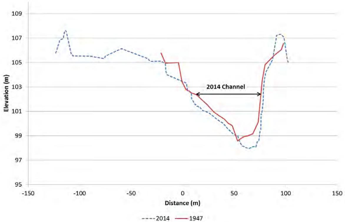
Figure 42. Clutha River/Mata-Au cross-section M7, looking downstream
