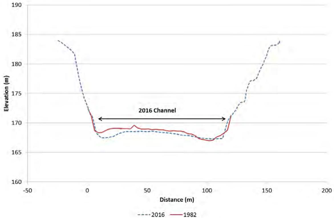
Figure 84. Clutha River/Mata-Au cross-section C36, looking downstream
