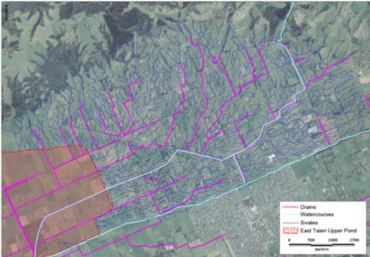
**Figure 3.6** Watercourses, drains and swales on the East Taieri Plain. Swales also cross the plain on the south side of the Silver Stream (including through parts of Mosgiel), although these features are not shown.
