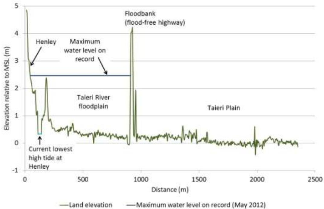
**Figure 3.10** Cross section from Henley to West Taieri Plain (as shown in Figure 3.11), showing the maximum water level observed between October 2002 and April 2012. The water level in the Taieri River at Henley is shown as the current lowest high tide (Figure 3.15).
