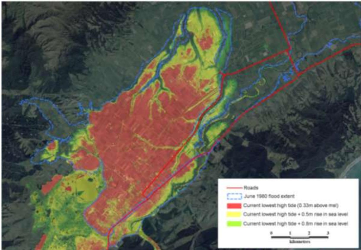
**Figure 3.15 Potential landward extent of inundation during a 'flood banks down' scenario on the West Taieri Plain. Note the correlation with the June 1980 flood (Figure 4.1), where numerous breaches in the flood banks occurred along the Waipori River and Contour Channel.**
