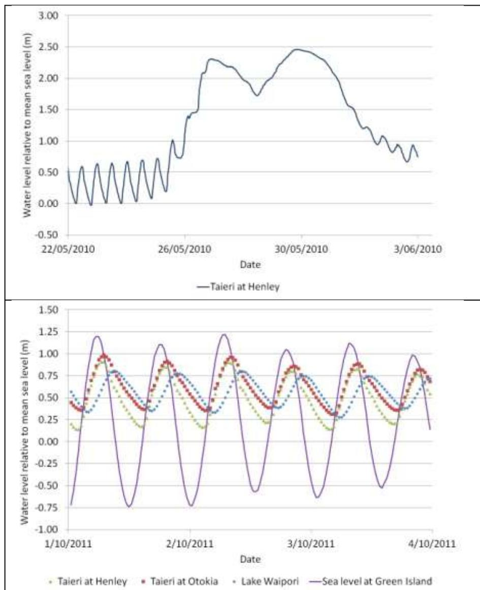
**Figure 3.12 Water level in the Taieri River at Henley during the May 2010 flood (top). Fluctuations in water level on the lower Taieri and Waipori rivers under normal, low flows and in the Pacific Ocean at Green Island (bottom).**
