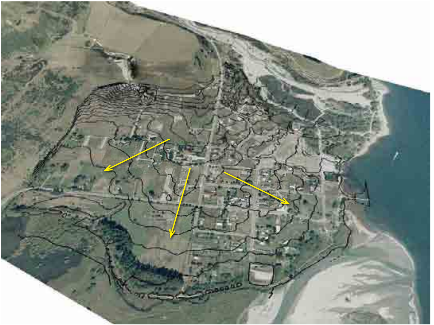
Figure 3: Digital Elevation Model and contour information representing the underlying topography of Glenorchy; yellow arrows indicate the slope of the land.
