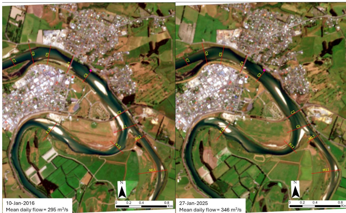
Figure 5-9: Satellite imagery of the Clutha River at Balclutha on two dates: January 10, 2016 (left) and January 27, 2025 (right). Imagery from Sentinel-2 satellite data. Red lines indicate the cross section locations. The flow monitoring site is shown with a magenta dot.
