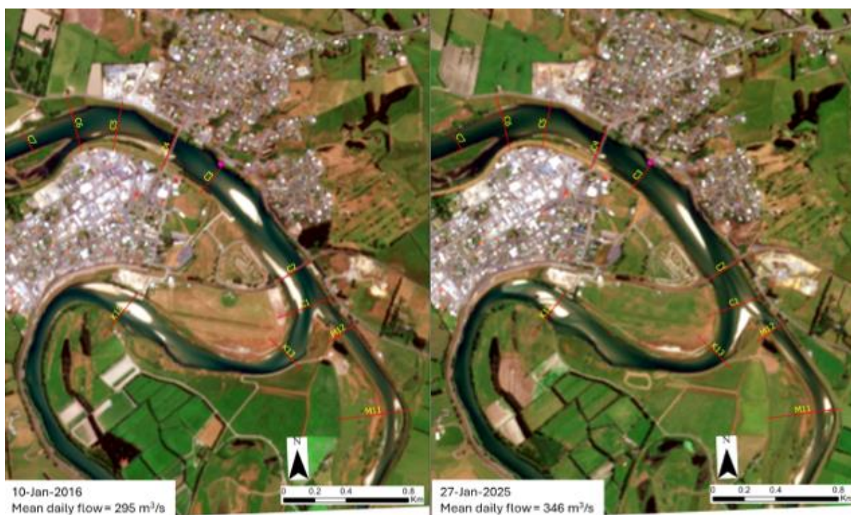
Figure 5-11: Satellite imagery of the Clutha River at Balclutha on two dates: January 10, 2016 (left) and January 27, 2025 (right). Imagery from Sentinel-2 satellite data. Red lines indicate the cross-section locations. The flow monitoring site is shown with a magenta dot.
