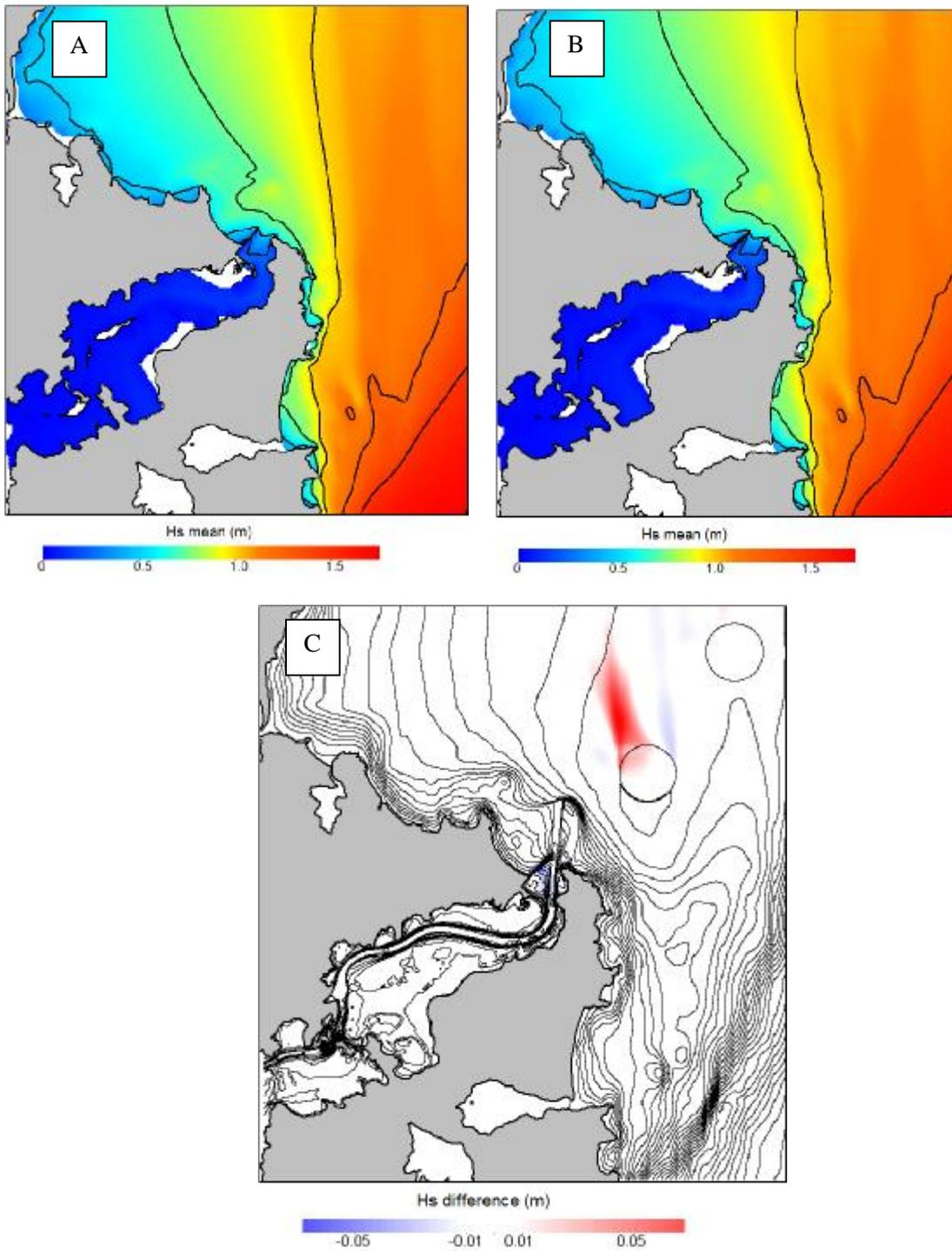
**Figure 3.7** Mean significant wave height (m) over 2003–2007 for the existing (A) and modified (B) bathymetries, plus the predicted differences in mean wave height (C) (Source: Bell *et al.* 2009, Figure 8.9).
