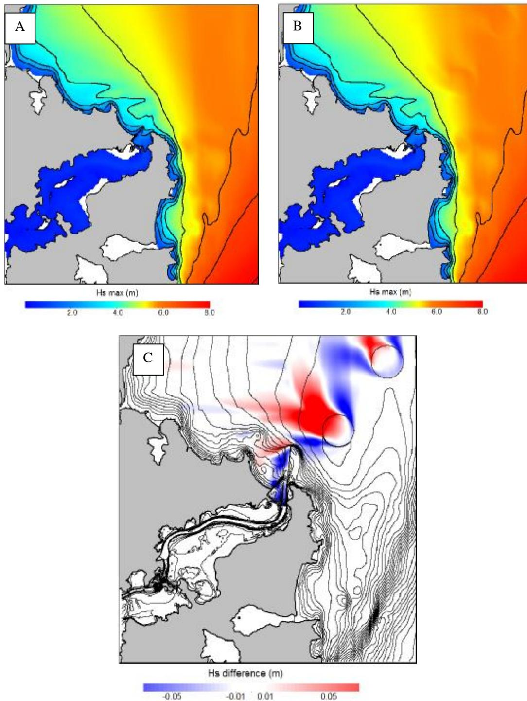
**Figure 3.8** Maximum significant wave height (m) for 2003–2007 for the existing (A) and modified (B) bathymetries, plus the differences in maximum wave height (C) (Source: Bell *et al.* 2009, Figure 8.10).
