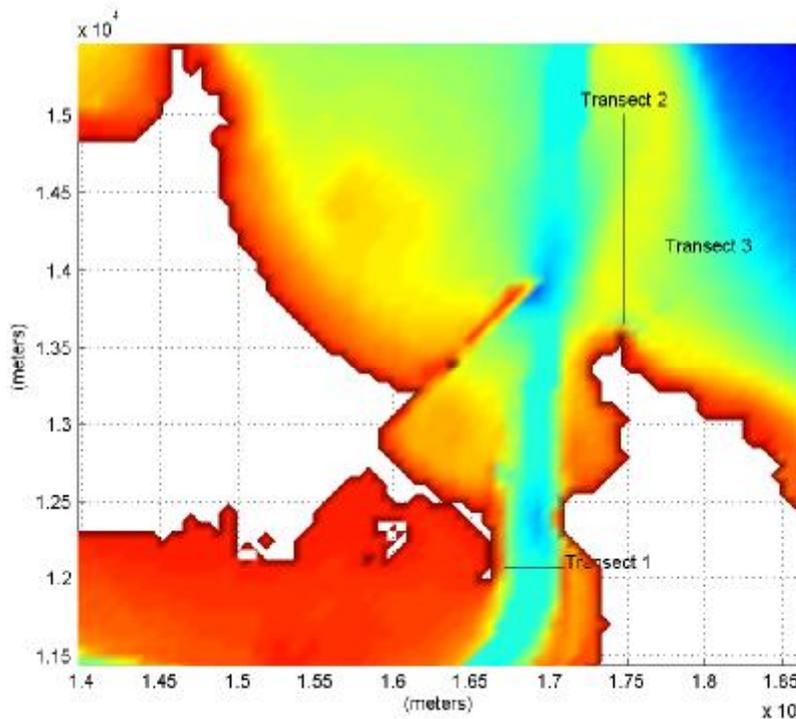
**Figure 3.5** Depth shading of the Entrance Channel area, showing locations of transects modelled for currents before and after dredging (Source: Bell *et al.* 2009, Figure 5.9).
