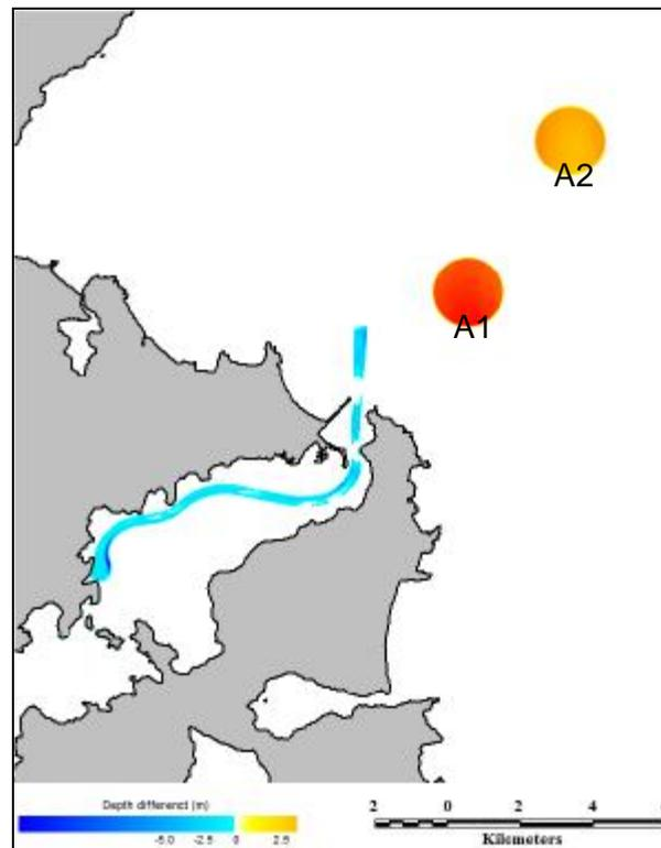
**Figure 3.6** Bathymetry difference between the existing bathymetry and proposed modifications (dredged 15-m option and two disposal area options, A1 and A2) (Source: Bell *et al.* 2009, Figure 8.8).
