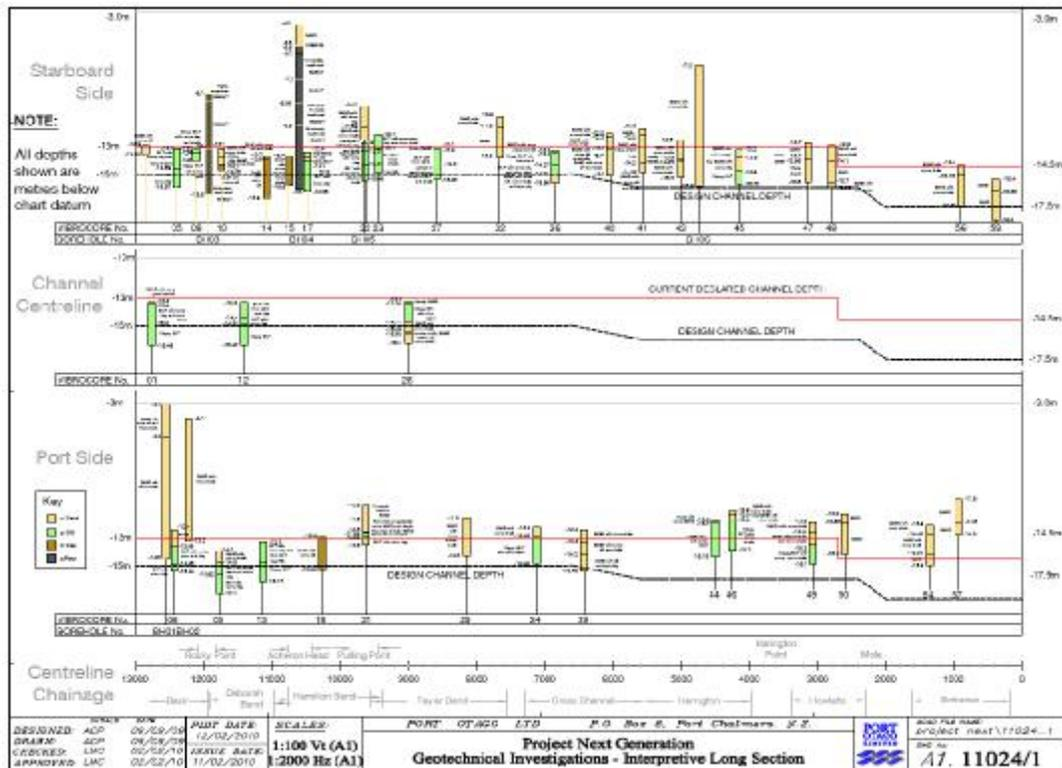
Figure 2.18 Description of sediments taken from bores relative to channel position (Port Otago Drawing 11024).
