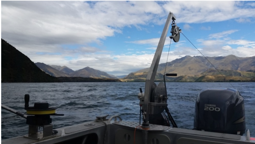
Figure 1 BioFish tow and communication cable. The BioFish is towed at varying speeds approximately 90 meters behind the boat and ‘swims’ up and down through the water as determined by the controller standing in the boat. Lake Wanaka, 26 February 2017.
