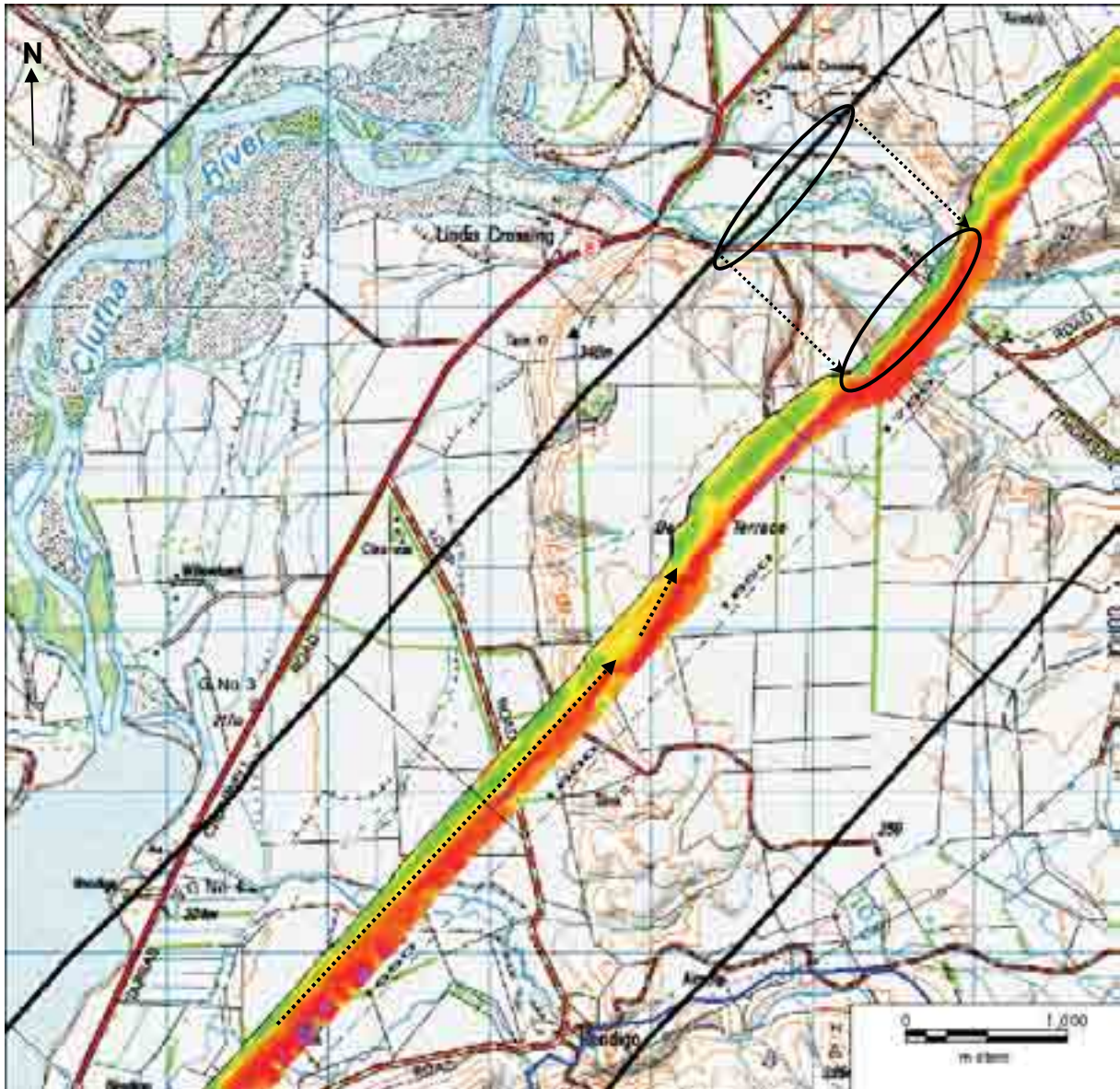
Figure 3.3 CDI profile along flight line 10700. Highlighted on the section are the dips seen in the underlying silt and the Lindis alluvial ribbon aquifer contained by the underlying silty sediments
