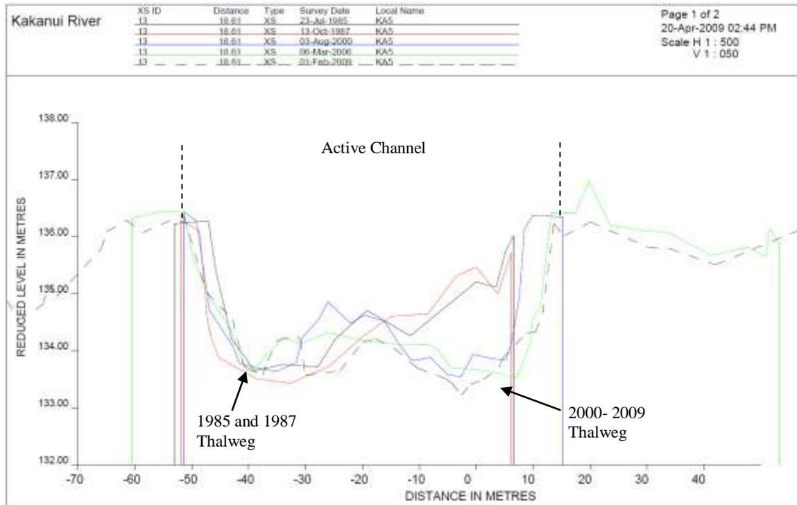
Figure 8.13 Cross-section KA5, looking downstream.
