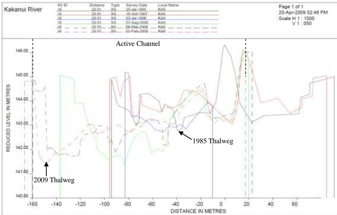
Figure 8.16 Cross-section KA8, looking downstream.
