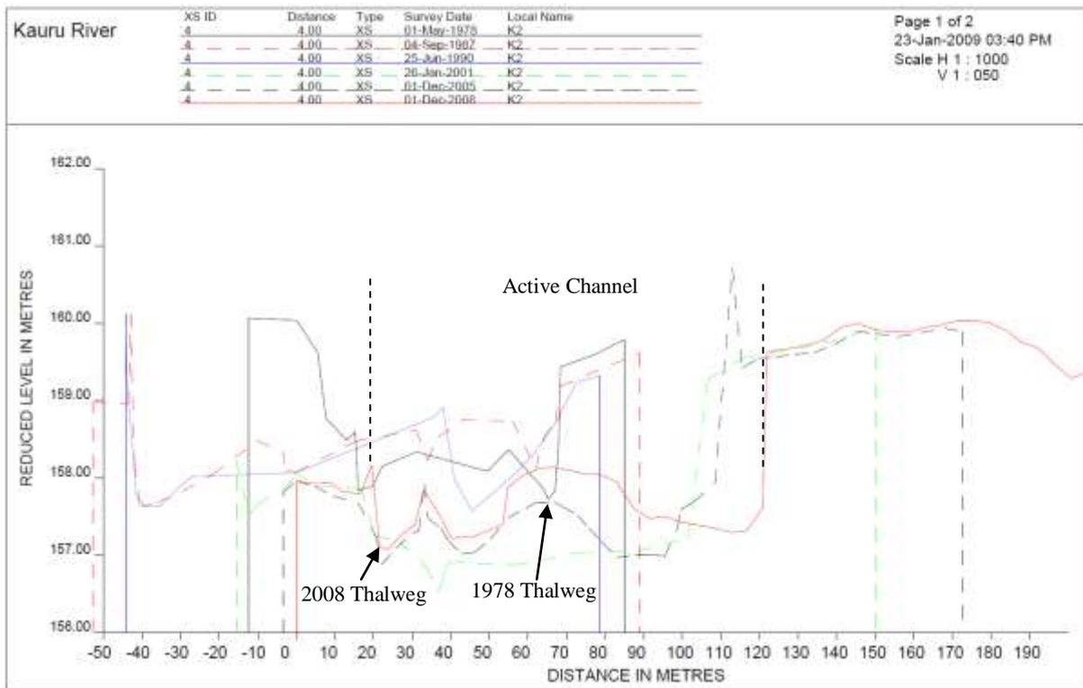
Figure 8.28 Cross-section K2, looking downstream.
