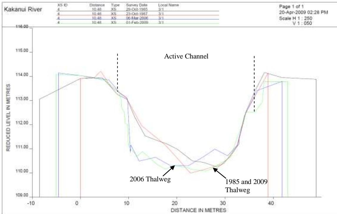
Figure 8.4 Cross-section 3/1, looking downstream.
