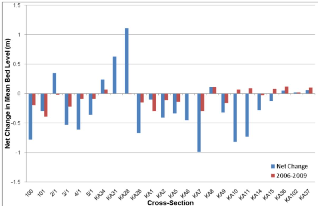
Figure 3.2 Graph showing net change in mean bed level across all survey periods and between the last two surveys (2006 and 2009) for each cross-section.
