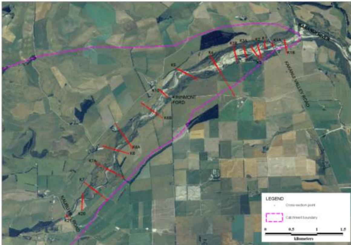
Figure 3.3 Location of surveyed cross-sections for the Kauru River superimposed on 2006 aerial photograph.
