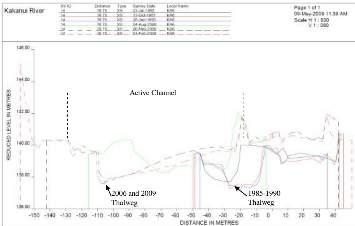
Figure 8.14 Cross-section KA6, looking downstream.
