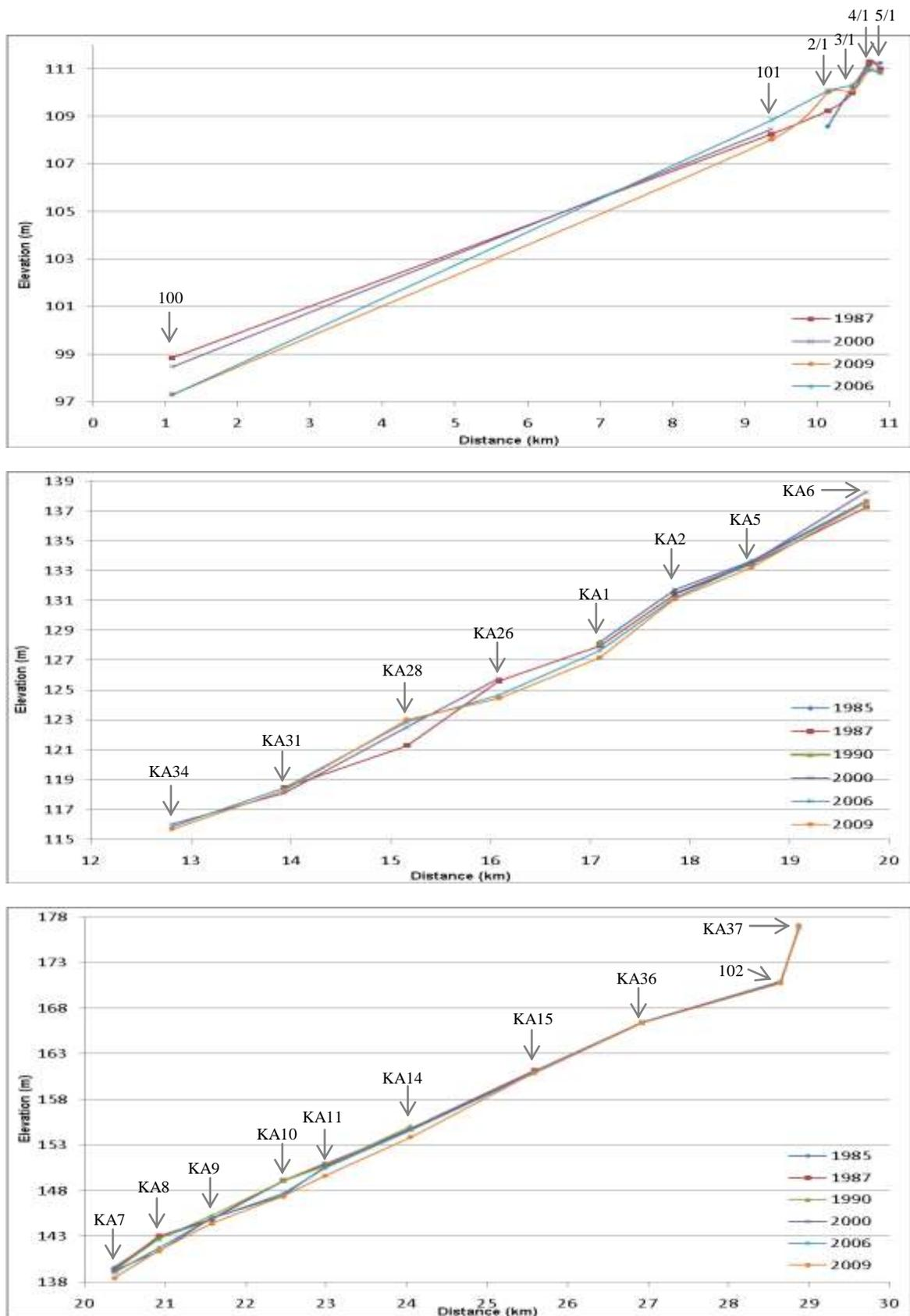
Figure 4.1 Longitudinal profile of the Kakanui River using minimum bed level. The river mouth is at 0km distance.
