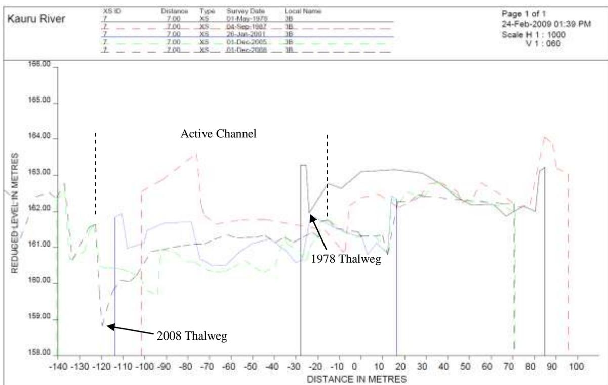
Figure 8.31 Cross-section K3B, looking downstream.
