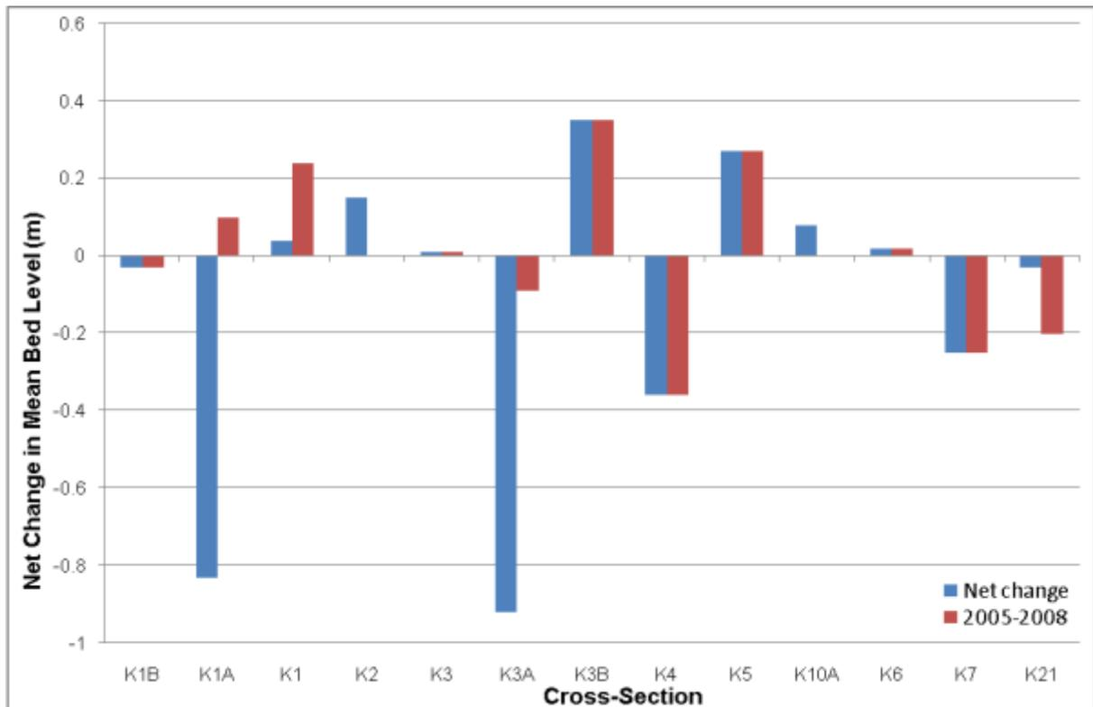
Figure 3.4 Graph showing net change in mean bed level across all survey periods and between the last two surveys (2005 and 2008) for each cross-section.
