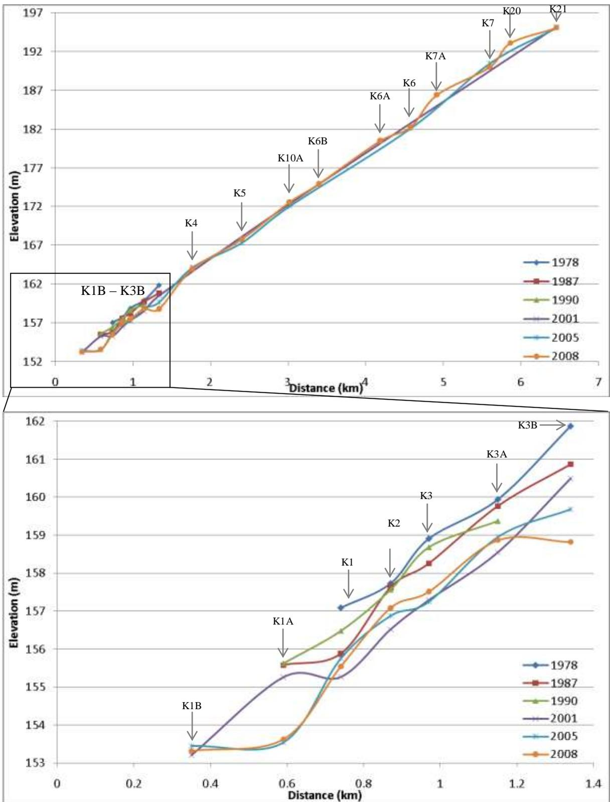
Figure 4.2 Longitudinal profile of the Kauru River, using minimum bed level. The river mouth is at 0km distance.
