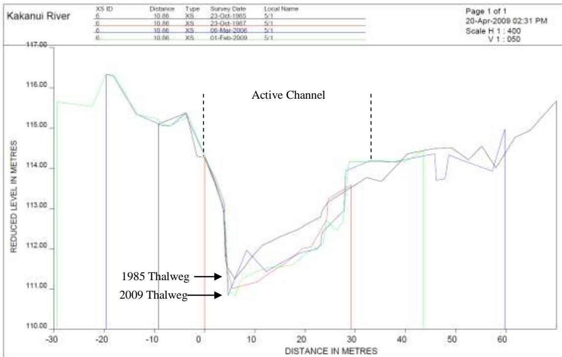
Figure 8.6 Cross-section 5/1, looking downstream.
