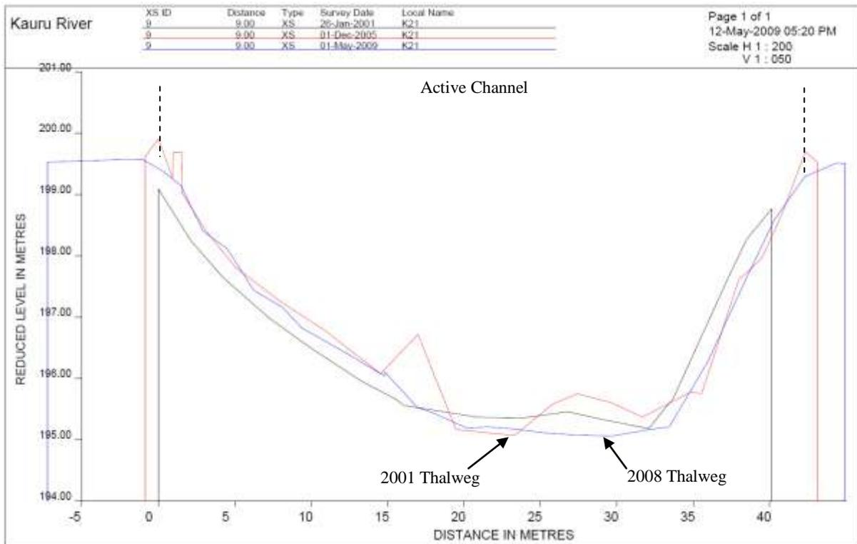
Figure 8.37 Cross-section K21, looking downstream.
