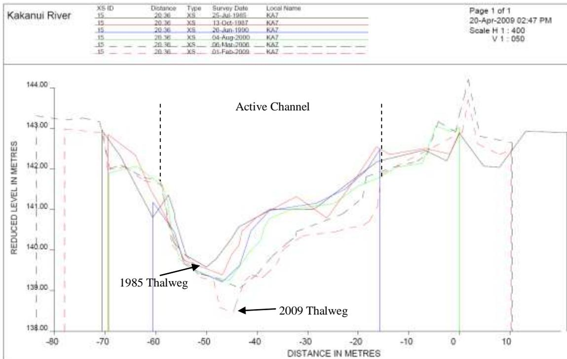
Figure 8.15 Cross-section KA7, looking downstream.
