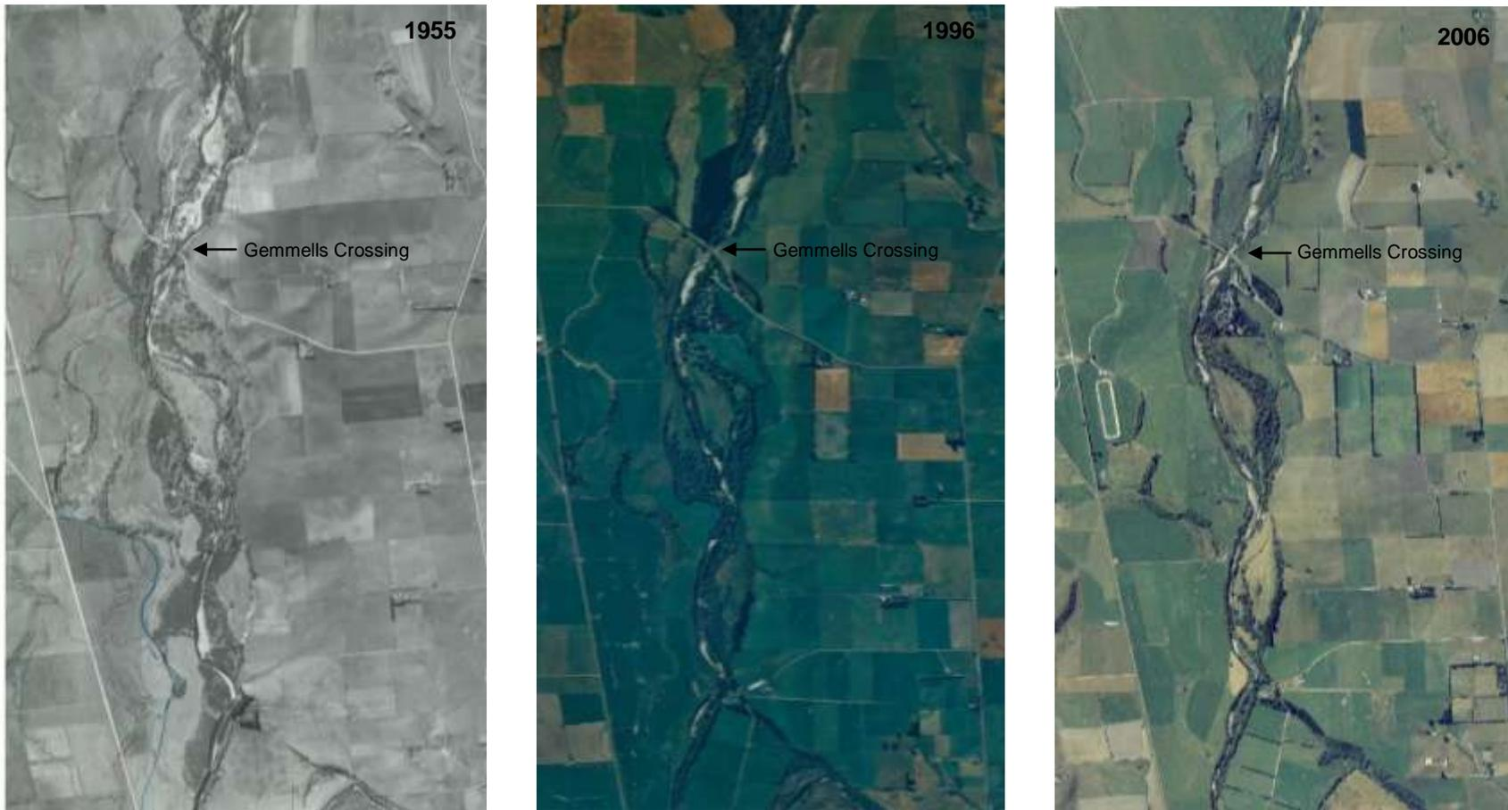
Figure 2.4C Aerial photographs of Kakanui River in 1955, 1996 and 2006 from 12 to 19km upstream of the river mouth.
