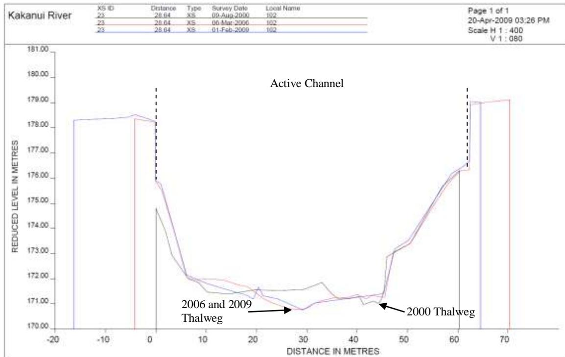
Figure 8.23 Cross-section KA102, looking downstream.
