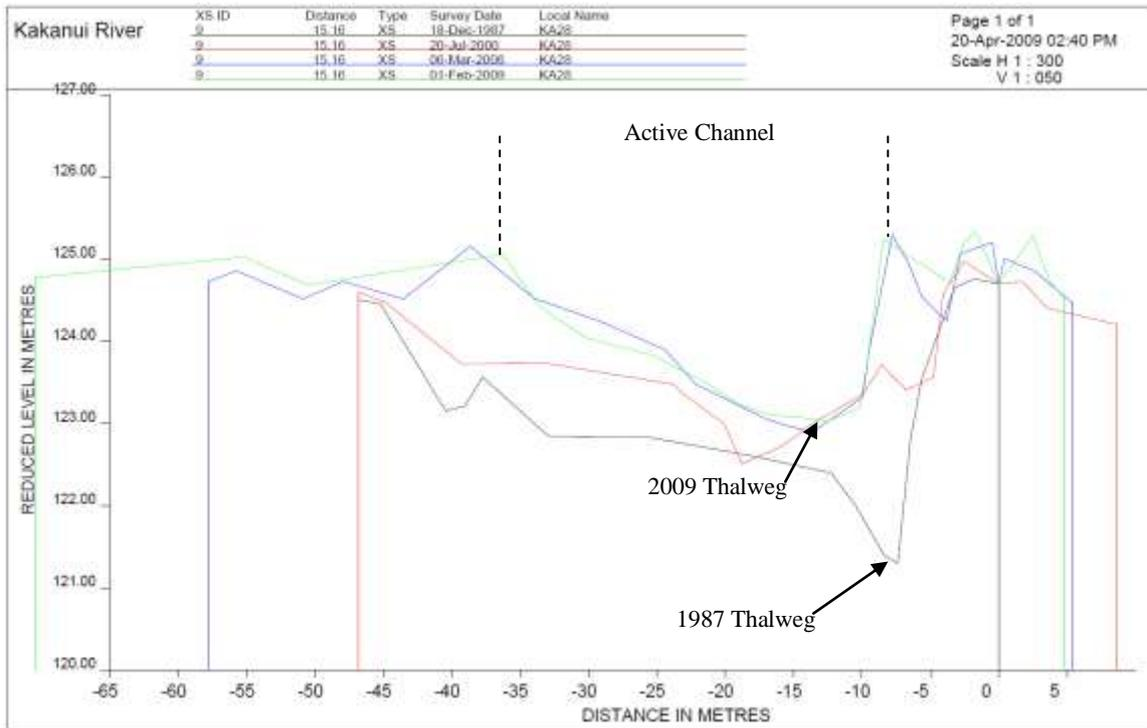
Figure 8.9 Cross-section KA28, looking downstream.
