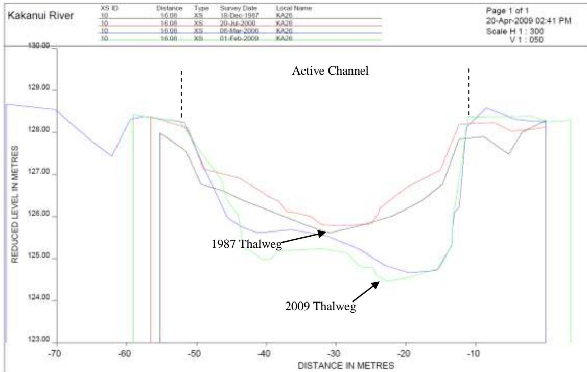
Figure 8.10 Cross-section KA26, looking downstream.
