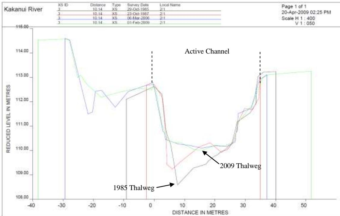
Figure 8.3 Cross-section 2/1, looking downstream.
