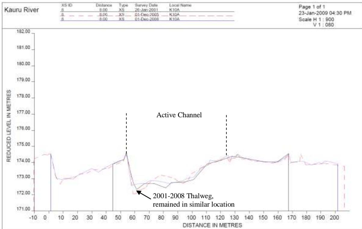
Figure 8.34 Cross-section K10A, looking downstream.
