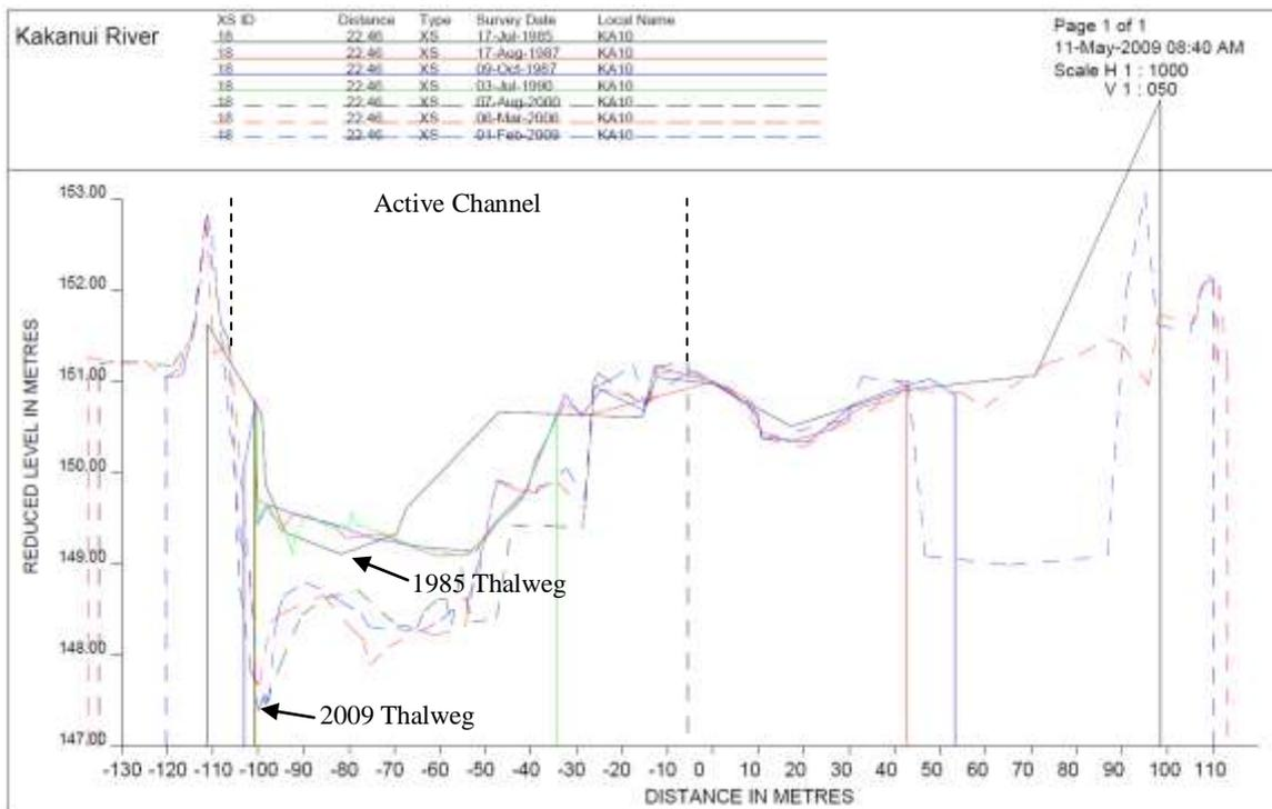
Figure 8.18 Cross-section KA10, looking downstream.
