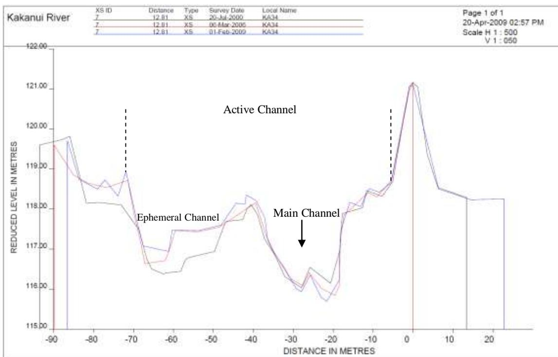
Figure 8.7 Cross-section KA34, looking downstream.
