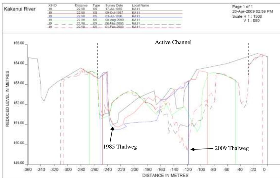
Figure 8.19 Cross-section KA11, looking downstream.
