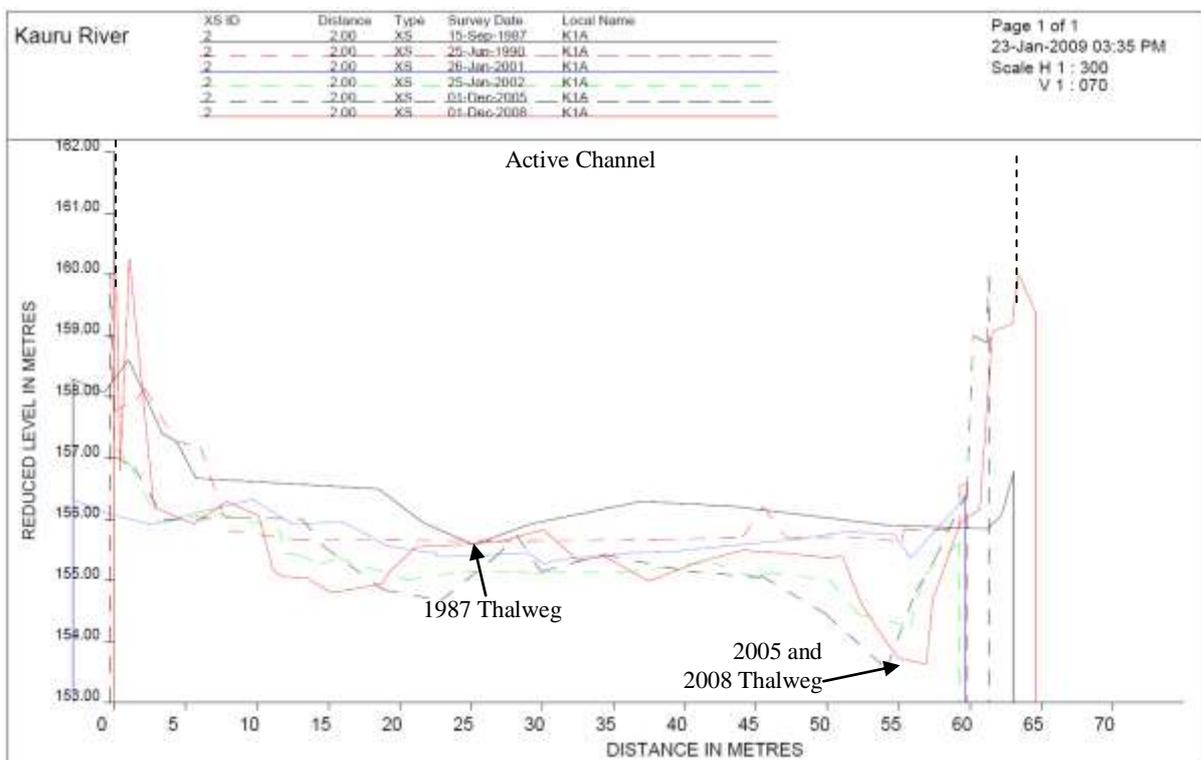
Figure 8.26 Cross-section K1A, looking downstream.
