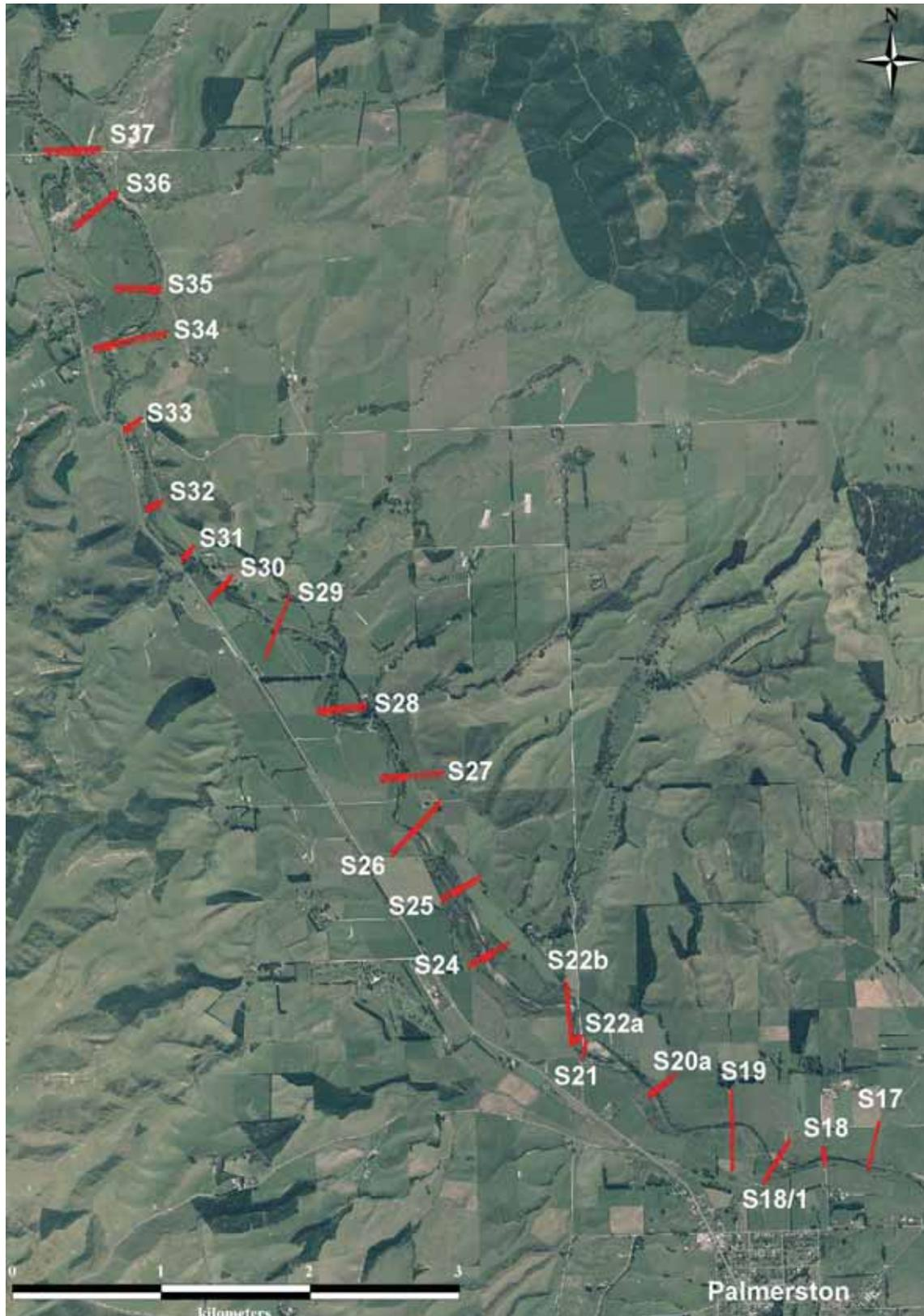
**Figure 3.1** Location of surveyed cross-sections for the Shag River superimposed on 2005 aerial photography
