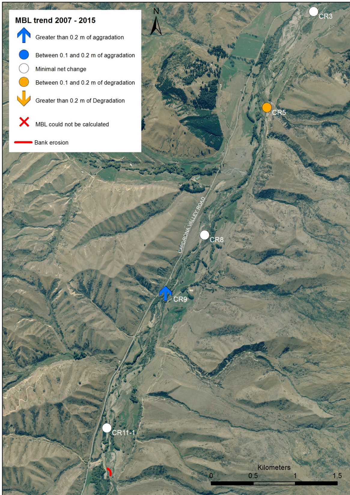
Figure 6. Location of Cardrona River cross-sections. The white, orange, and blue symbols show the magnitude of MBL change at each cross-section between 2007 and 2015. Locations where significant bank erosion has been observed are shown as red lines, a red cross indicates a cross-section where MBL could not be calculated. Individual cross-sections are shown in Appendix 3.
