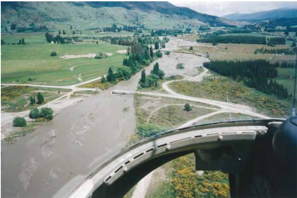
Figure B.14 Flood sedimentation at the Ballantyne Road Bridge looking upstream, November 1999
