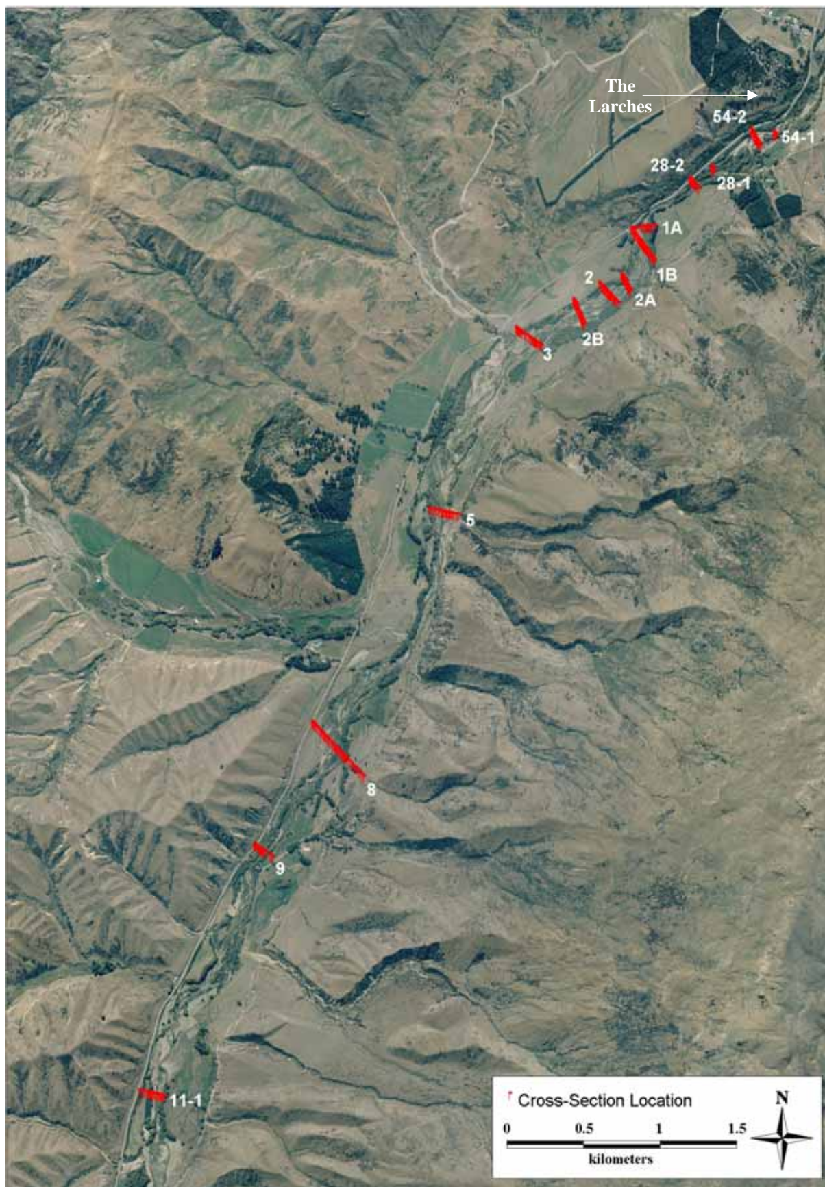
Figure 3.2 Location of surveyed cross sections for the Cardrona River mid-catchment superposed onto 2006 aerial photography
