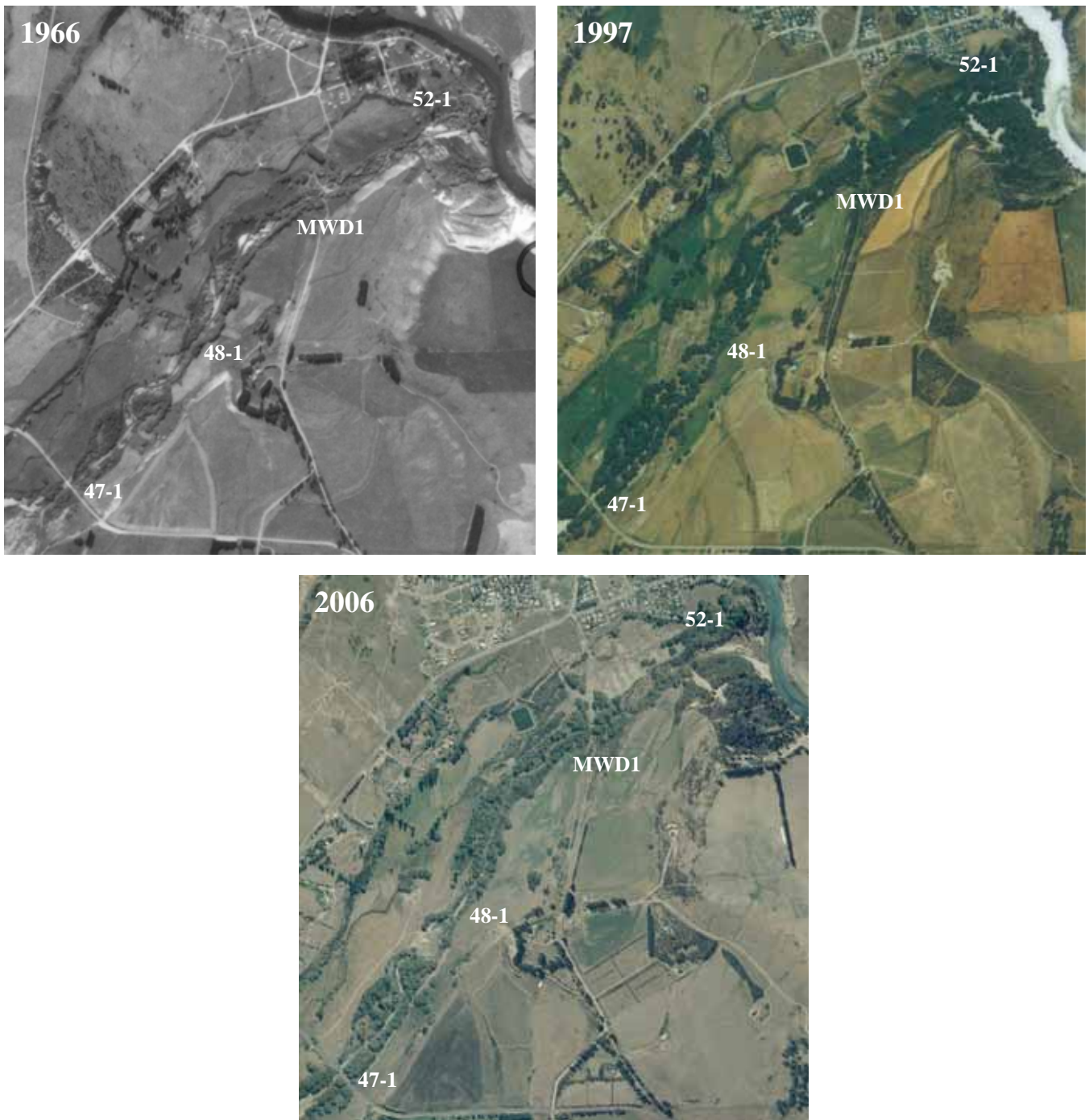
Figure 8.2.1 Aerial images of the Cardrona River in the vicinity of cross sections 52-1 to 47-1 for 1966, 1997 and 2006. These cross sections are located downstream of the State Highway 6 Bridge and between 0.25 and 2.5km upstream of the Clutha River/Mata-Au confluence
