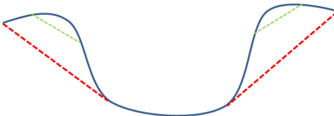
Figure 1: Cross section of water course with example of battering compared with bank/channel reshaping
