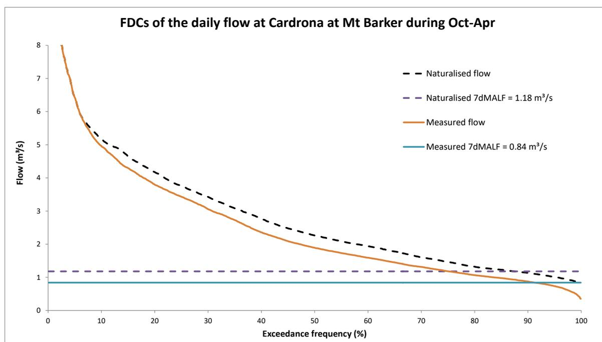
**Figure 3.1** Flow duration curves of the daily flow at Mt. Barker during the irrigation season (October-April).
