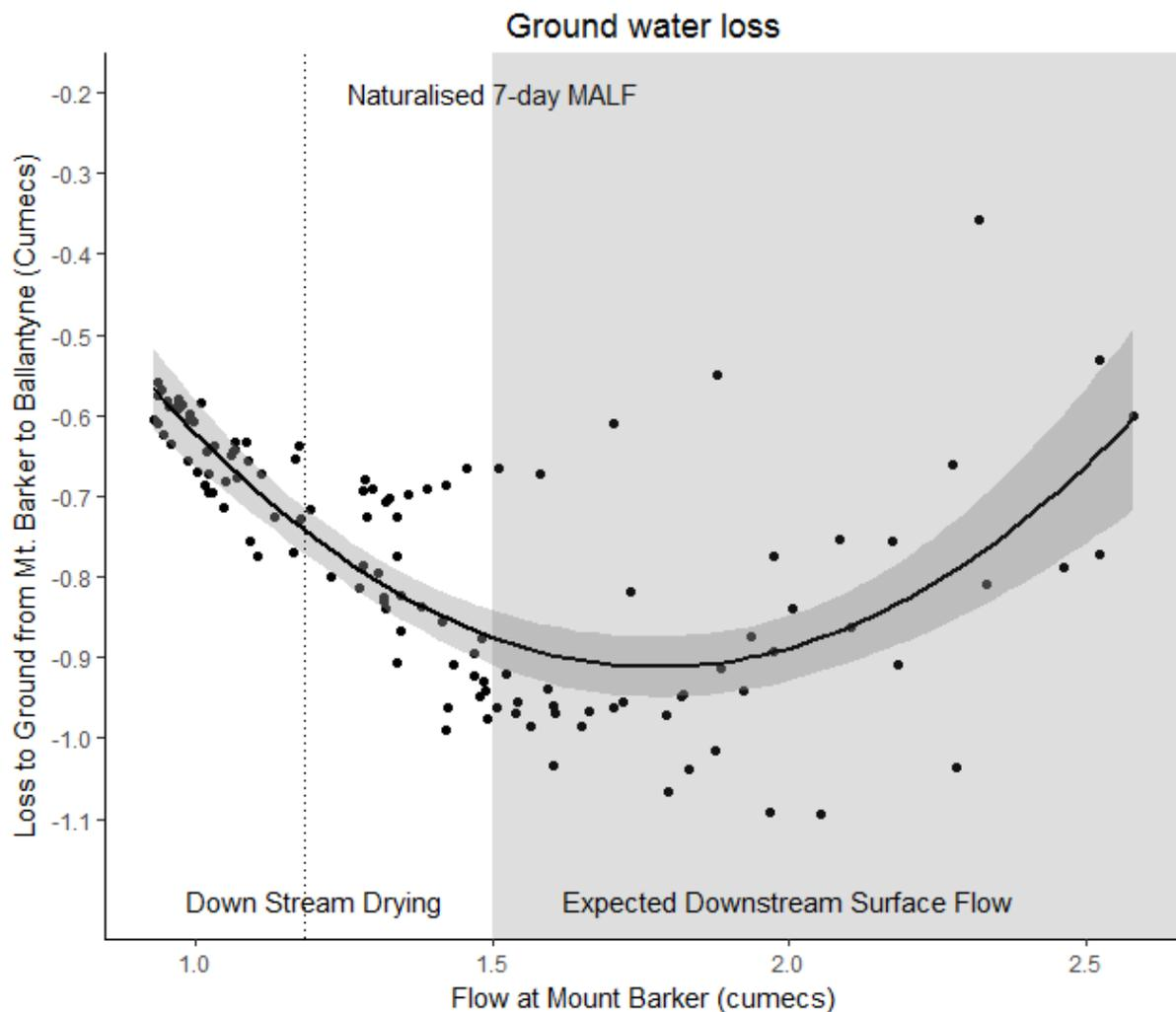
**Figure 3.5** Quadratic model fit of the relationship between flow at Mt. Barker and groundwater loss from Mt. Barker to Ballantyne Road with a shaded (grey) 99% confidence interval and naturalised minimum flow. Shaded expected downstream flow regions are based upon the inflection point of groundwater loss. When flow values exceed this point (1.5 cumeecs), downstream surface connectivity is more likely to be maintained.
