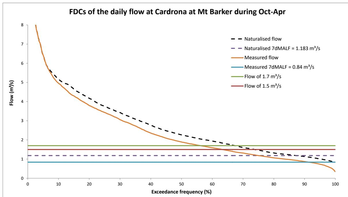
**Figure 3.10** Flow duration curves of the daily flow at Mt. Barker during the irrigation season (October-April).
