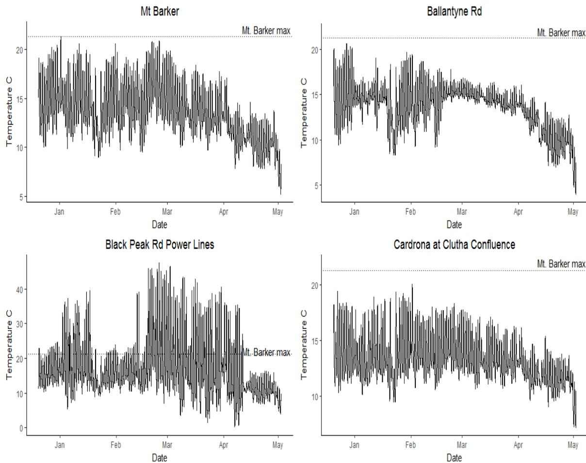
**Figure 3.6** Temperature graphs for four sites along the Cardrona River. Mt. Barker maintained flow and had a maximum daily temperature of 21.3 °C. Black Peak (note the greater y-axis scale) routinely exceeds this temperature by more than 10 °C suggesting a dry reach
