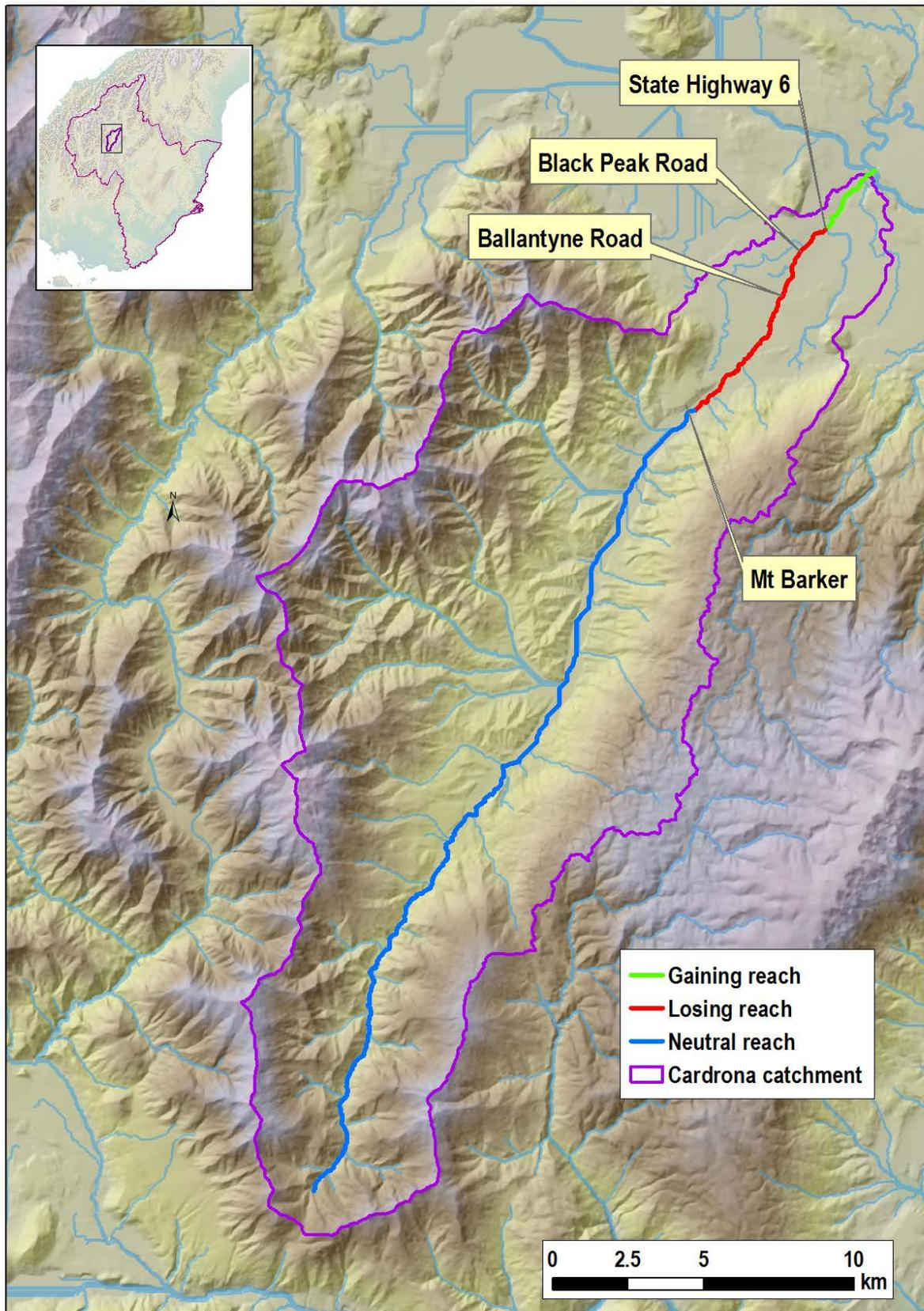
Figure 3.3 Location the three different hydrological reaches in the Cardrona River
