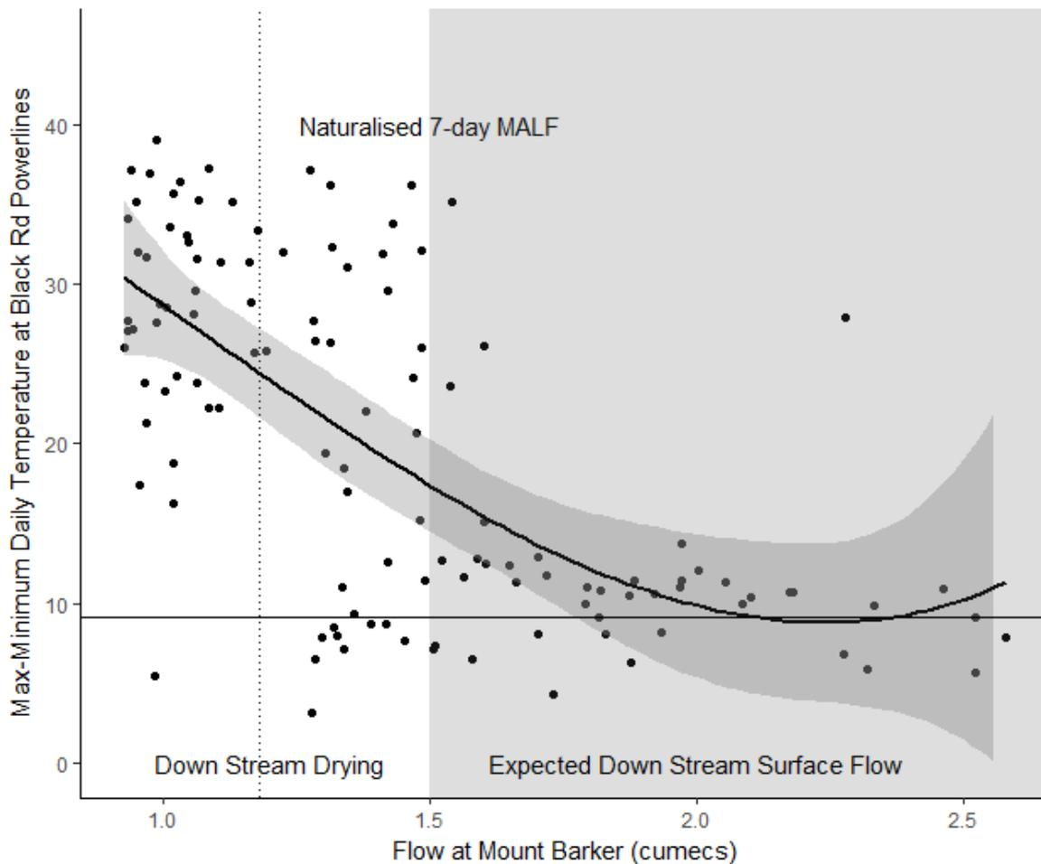
**Figure 3.8** Temperature range (daily maximum-daily minimum) at Black Peak Rd power lines and flow at Mt. Barker with 95% confidence interval. The shaded rectangle represents flows at which downstream connectivity is likely to occur based estimates from Figure 3.5
