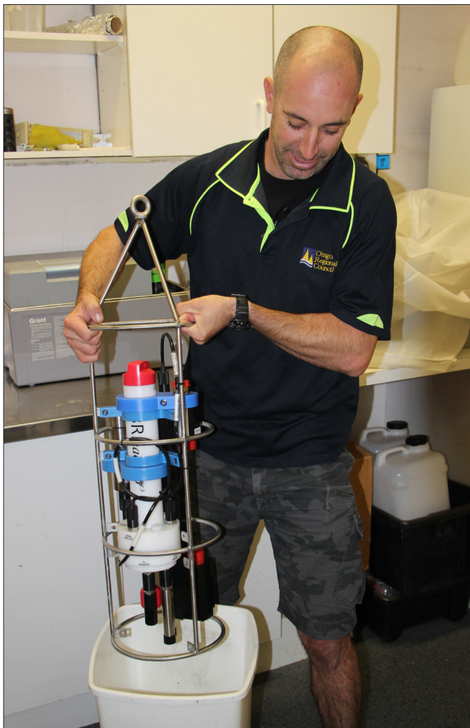
Environmental monitoring officer Nathan Manning tests the new sonde that will be used to record data from the depths of the Queenstown and Central Otago lakes
