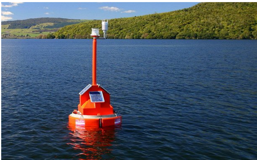
Fig. 10: An example lake monitoring buoy (photo c/o Chris McBride).
