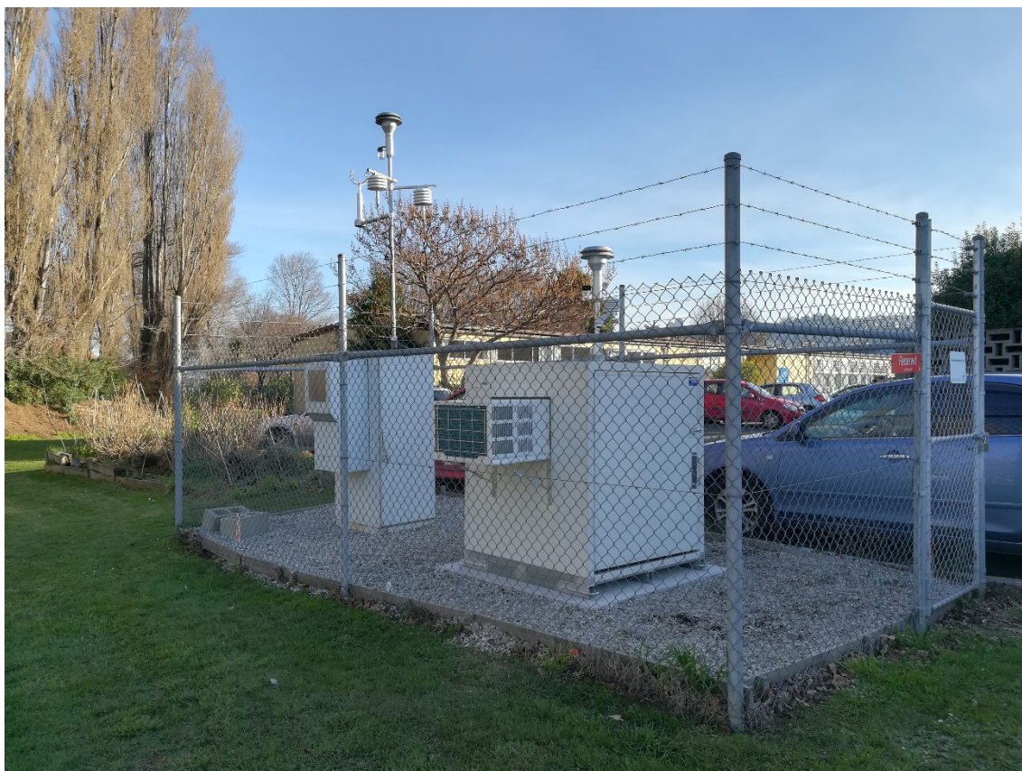
Figure 5. New PM 2.5 monitor in Central Dunedin is shown on the right along with the existing PM 10 monitor on the left.
