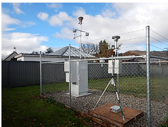
Figure 3: ORC's air quality monitoring site in Alexandra. The PM 2.5 monitor is on the right and the PM 10 monitor is on the left.
