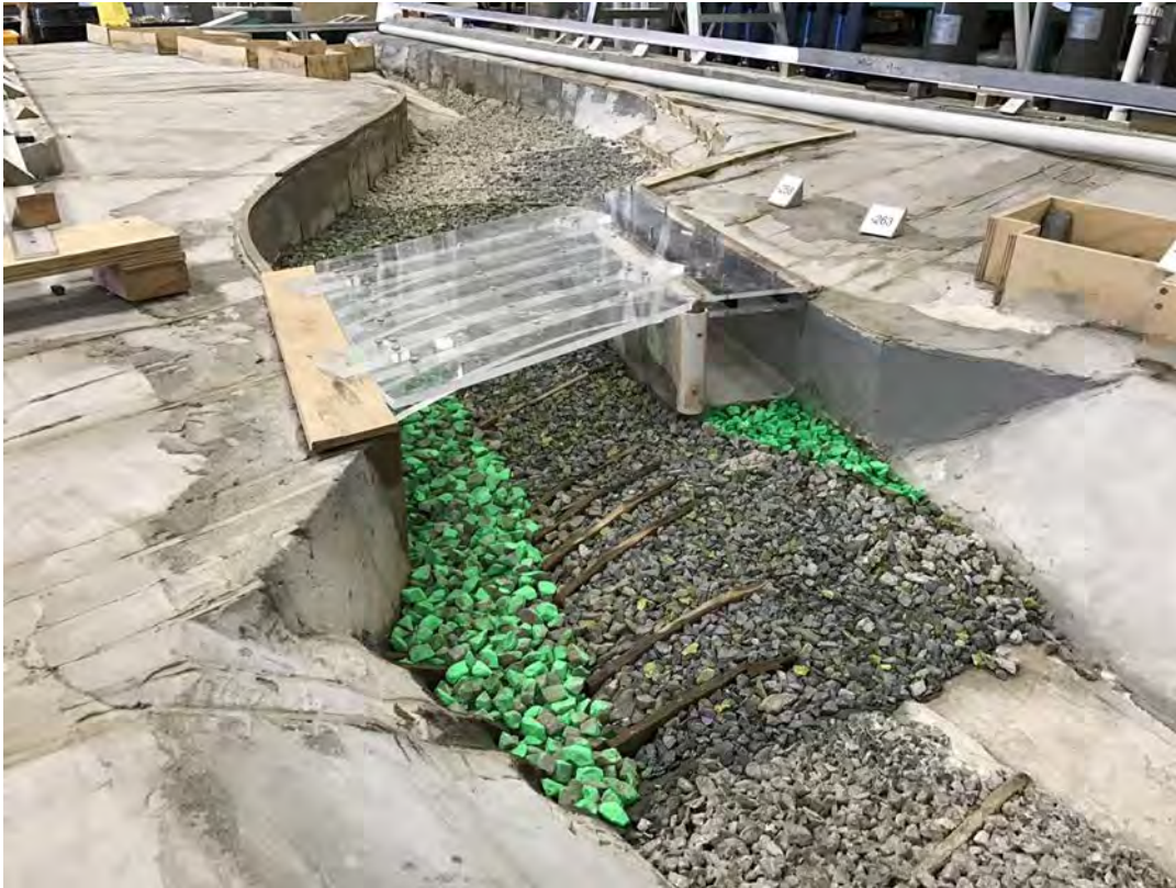
Figure 5. Scale physical model of Water of Leith at Dundas Street bridge, looking downstream. The proposed new culvert is at the right of the channel.
