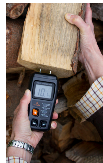
A moisture meter checking the wood dryness
