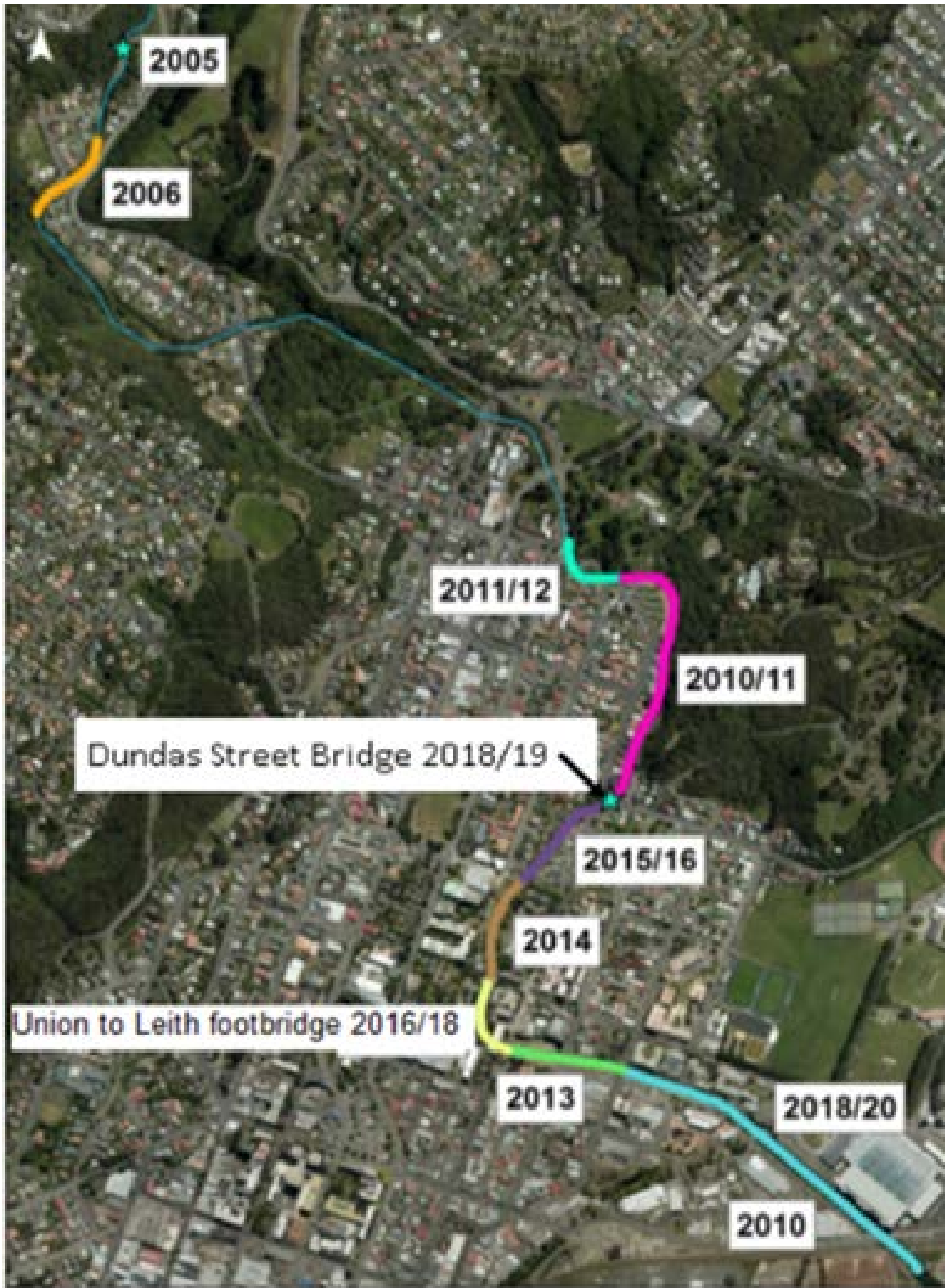
Figure 6. Staging of construction of the Leith Flood Protection Scheme.
