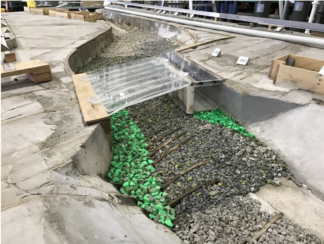
Figure 5. 1:25 scale physical model of the Water of Leith at Dundas Street bridge, looking downstream. The proposed new culvert is at the right of the bridge. The model was constructed at the Water Engineering Laboratory of the Department of Civil and Environmental Engineering, University of Auckland.
