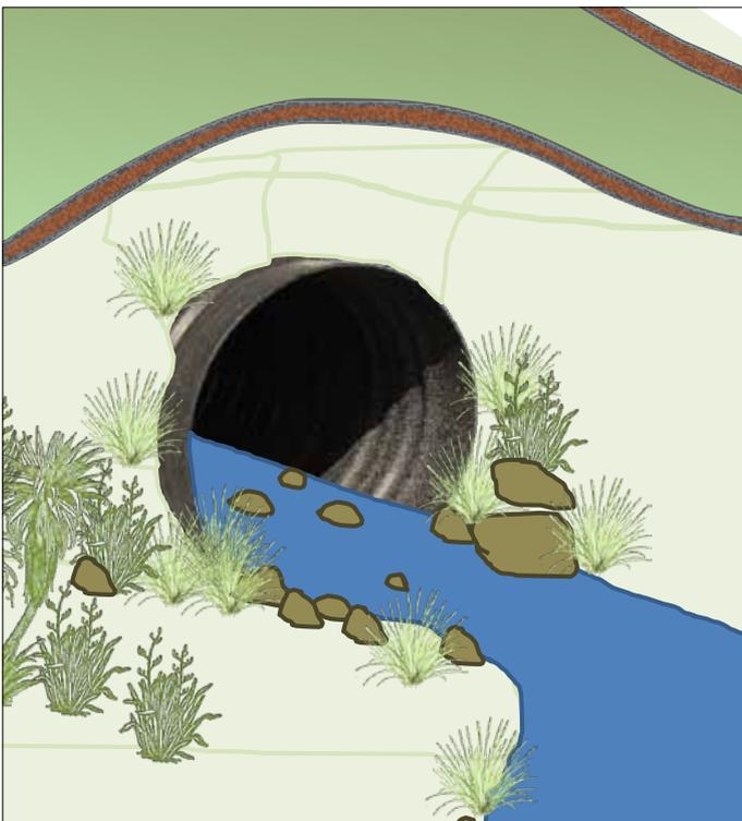
Ensure your culvert is at least as wide as your stream or creek. The bottom of the culvert should mimic the natural bed.
