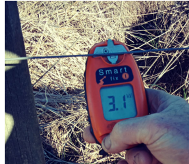
Fence voltage (earthed)
