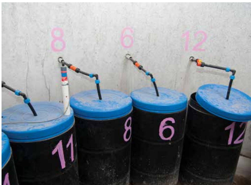
Figure 5.1 Lysimeters have been developed to quantify nutrient leaching losses from soil by capturing all the water leaving a defined area of soil, which can then be analysed for its nutrient concentrations. This information can be used to improve Overseer model estimates.
