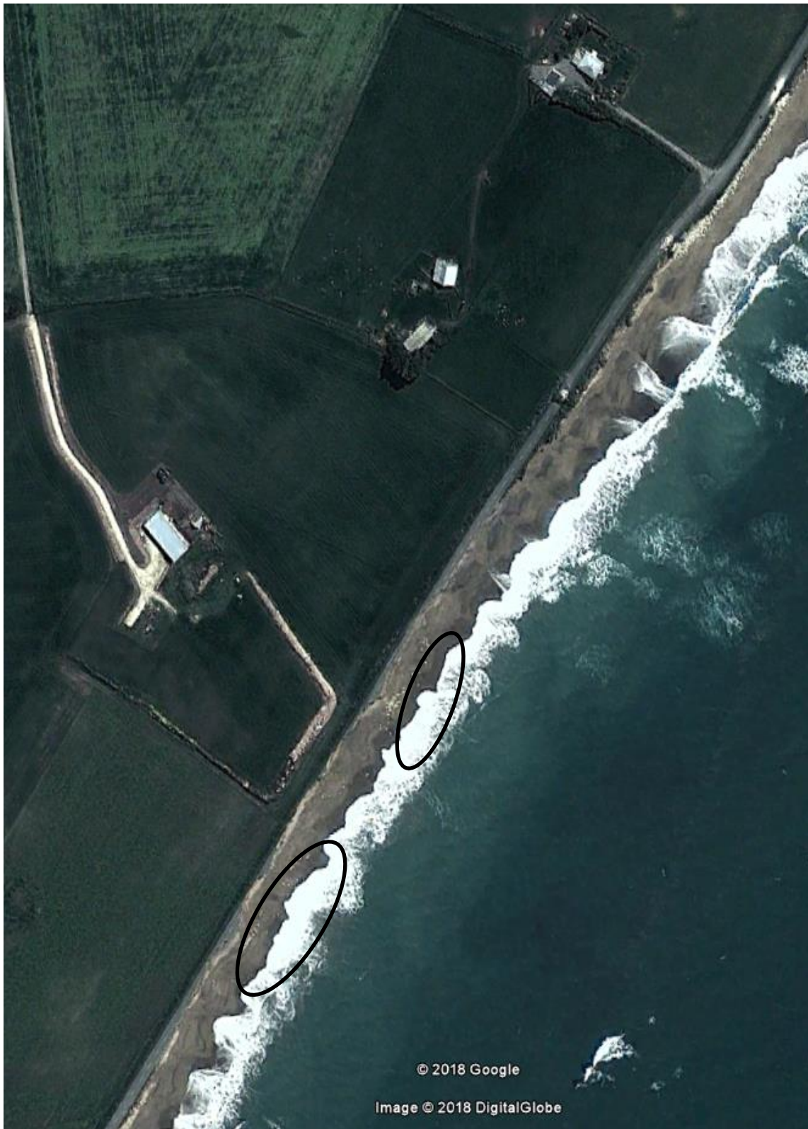
Figure 4-2: Riprap section on Beach Road viewed on satellite imagery of 03/10/2012. The view is the same as shown on Figure 4-1. Note the material of the failed riprap scattered on the foreshore (circled in black). Imagery source: DigitalGlobe.
