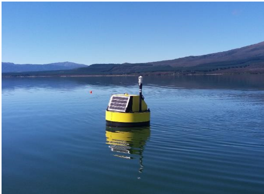
Figure 4-1 Monitoring buoy similar to that to be installed in Lake Hayes by ORC
