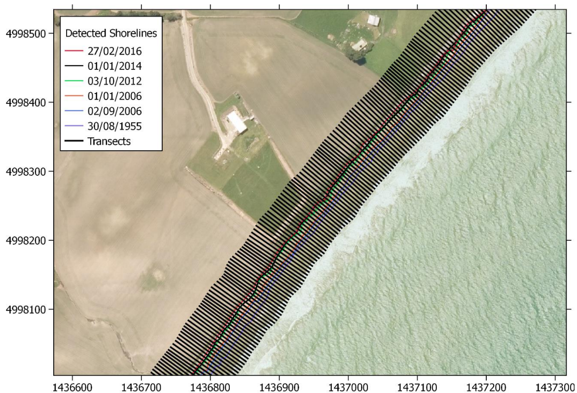
Figure 3-3: Example of transects perpendicular to the coast. The distance alongshore between each transect is 5 m. [Image source: LINZ].
