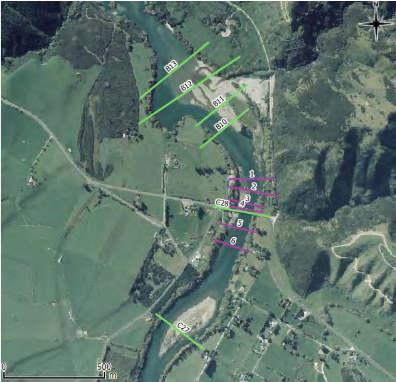
Figure 3-1 Cross-sections surveyed by Eliot Sinclair (shown in pink) and by ORC (shown in green)
